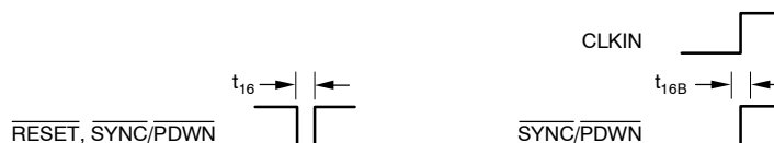
Figure 3. \overline{RESET} and \overline{SYNC/PDWN} Timing
