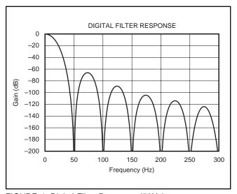
FIGURE 4. Digital Filter Response (50Hz).
