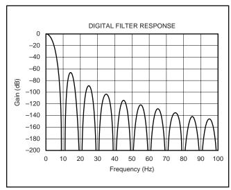
FIGURE 6. Digital Filter Response (10Hz Multiples).
