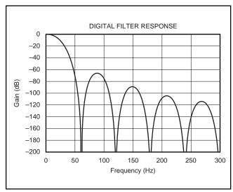
FIGURE 5. Digital Filter Response (60Hz).
