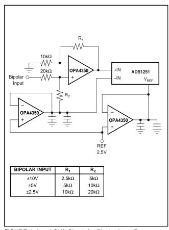
FIGURE 1. Level-Shift Circuit for Bipolar Input Ranges.
