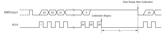
Figure 7-11. Offset-Calibration Timing
