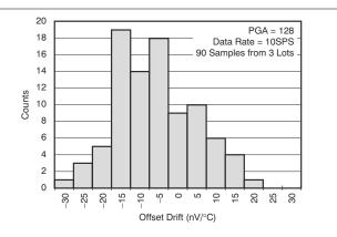
Figure 5-13. Offset Drift (-40°C to +25°C)
