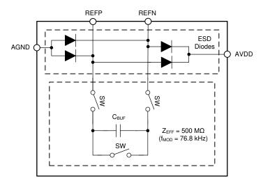
Figure 7-3. Simplified Reference Input Circuitry
