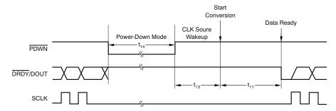
Figure 7-14. Wake-Up Timing From Power-Down Mode
