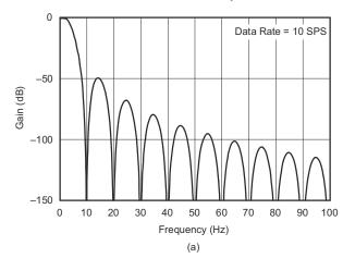
Figure 7-6. Digital Filter Frequency Response to 100 Hz
