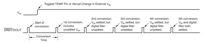
Figure 7-8. Settling Time in Continuous Conversion Mode
