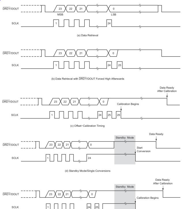
(e) Standby Mode/Single Conversions with Offset Calibration
