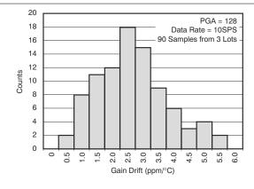
Figure 5-15. Gain Drift (-40°C to +25°C)
