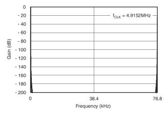
Figure 7-5. Digital Filter Frequency Response
