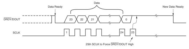
Figure 7-10. Data Retrieval With DRDY/DOUT Forced High Afterwards
