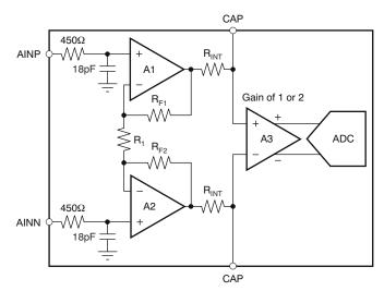
Figure 7-2. Simplified Diagram of the PGA
