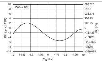
Figure 5-21. Integral Nonlinearity vs Input Signal
