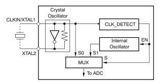
Figure 7-4. Equivalent Circuitry of the Clock Source
