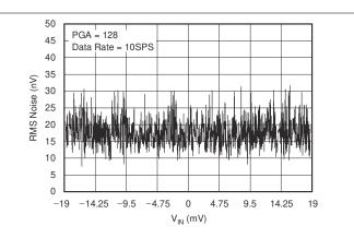
Figure 5-19. Noise vs Input Signal
