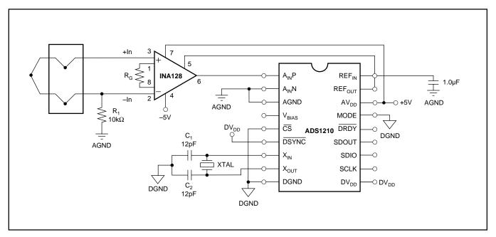
FIGURE 42. Dual Supply, High-Accuracy Thermocouple.
