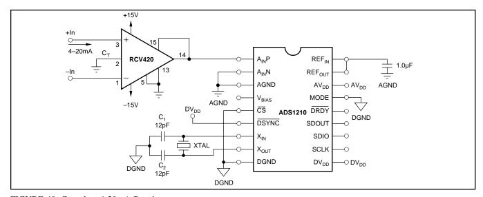
FIGURE 40. Complete 4-20mA Receiver.
