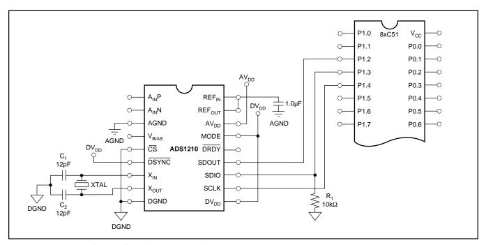
FIGURE 29. Three-Wire Interface with a 8xC51 Microprocessor.
