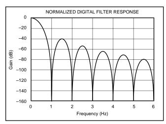
FIGURE 1. Normalized Digital Filter Response.
