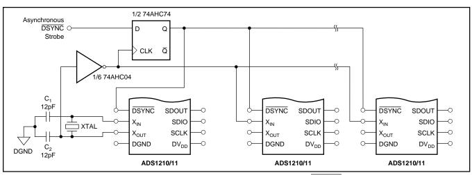
FIGURE 23. Exactly Synchronizing Multiple ADS1210/11s to an Asynchronous DSYNC Signal.
