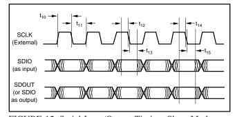
FIGURE 15. Serial Input/Output Timing, Slave Mode.
