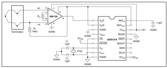
FIGURE 41. Single Supply, High-Accuracy Thermocouple.
