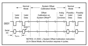
FIGURE 6. System Offset Calibration Timing.
