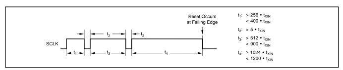
FIGURE 27. Resetting the ADS1210/11 (Slave Mode only).
