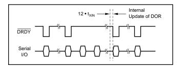
FIGURE 24. Timing of Data Output Register Update.
