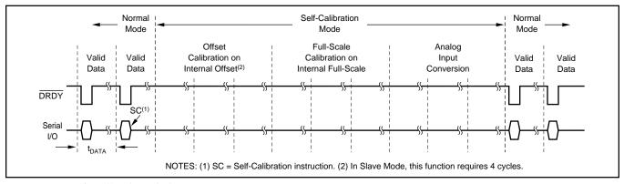
FIGURE 5. Self-Calibration Timing.
