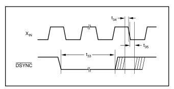
FIGURE 22.  $\overline{DSYNC}$  to  $X_{IN}$  Timing for Synchronizing Mutliple ADS1210/11s.
