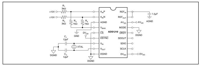
FIGURE 12. ±10V Input Configuration Using V<sub>BIAS</sub>.
