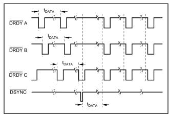
FIGURE 36. Effect of Synchronization on Output Data Timing.
