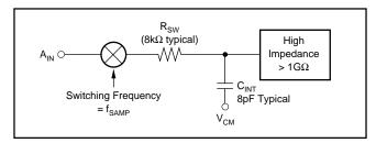
FIGURE 11. Analog Input Structure.
