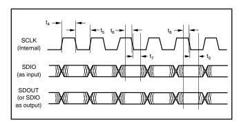
FIGURE 14. Serial Input/Output Timing, Master Mode.
