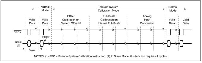
FIGURE 8. Pseudo System Calibration Timing.
