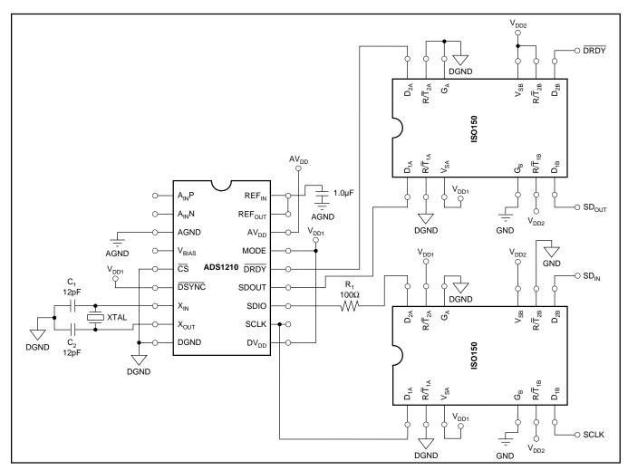
FIGURE 33. Isolated Four-Wire Interface.
