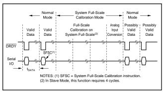
FIGURE 7. System Full-Scale Calibration Timing.
