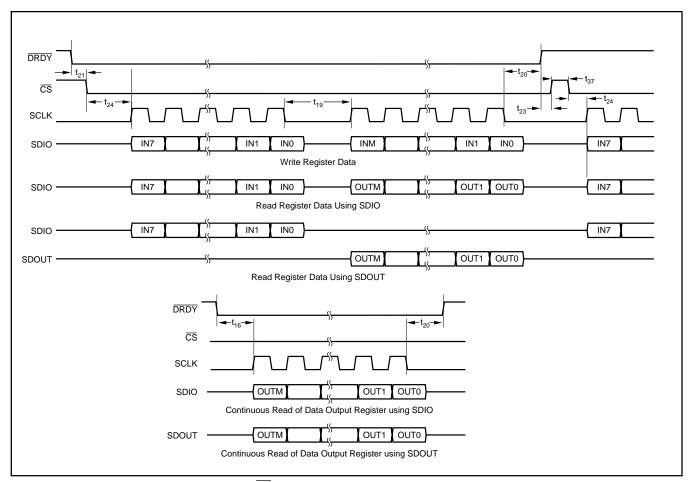
FIGURE 19. Serial Interface Timing (Using  $\overline{CS}$ ), Slave Mode.
