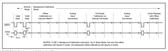
FIGURE 9. Background Calibration Timing.
