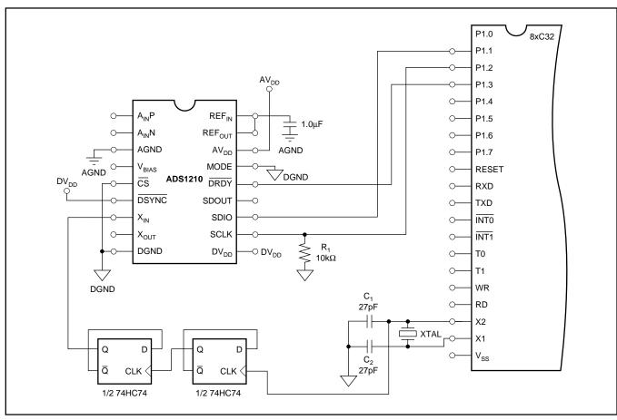
FIGURE 28. Three-Wire Interface with a 8xC32 Microprocessor.
