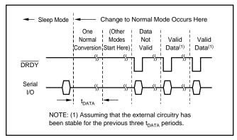
FIGURE 10. Sleep Mode to Normal Mode Timing.
