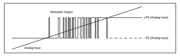
Figure 37. Analog Input vs Modulator Output of the ADS1208
