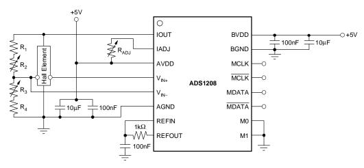
A. For Functional configuration (Mode 0), possible Hall elements include the Toshiba THS119 and the Philips KMZ10.
