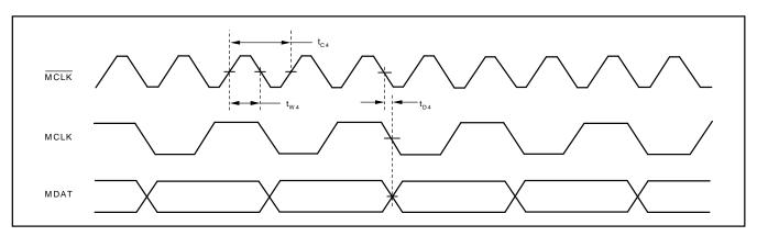
note: MCLK is system clock input. MCLK is modulator clock output. Modulator clock frequency is half of system clock frequency.
