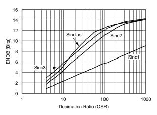
Figure 40. Measured ENOB vs OSR
