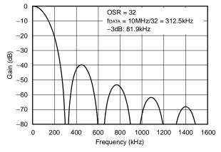
Figure 38. Frequency Response of Sinc<sup>3</sup> Filter
