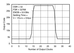
Figure 39. Pulse Response of Sinc<sup>3</sup> Filter  $(f_{MOD} = 10MHz)$
