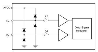
Figure 35. Equivalent Input Circuit
