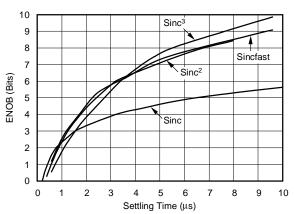
Figure 41. Measured ENOB vs Settling Time
