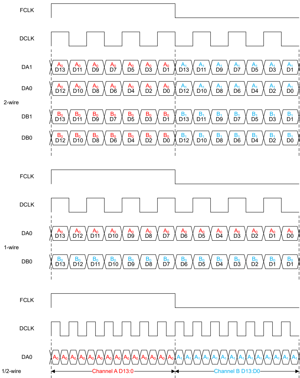
Figure 7-33. Output Data Format in Real Decimation (14-bit Output Resolution)
