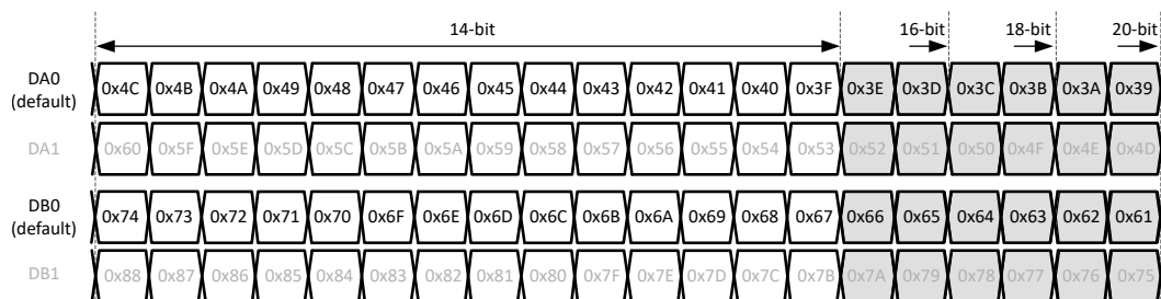
Figure 8-38. 1-wire output bit mapping
