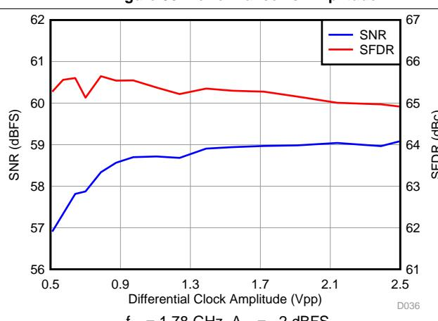
Figure 60. Performance vs Clock Amplitude
