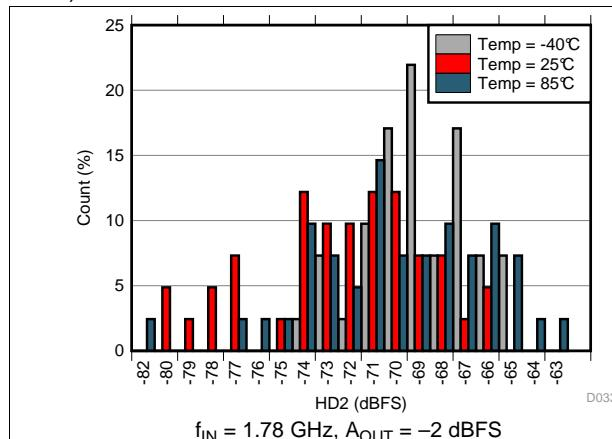
Figure 57. HD2 Histogram at AVDD19 = 2.0 V
