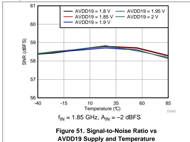
**Figure 51. Signal-to-Noise Ratio vs AVDD19 Supply and Temperature**
