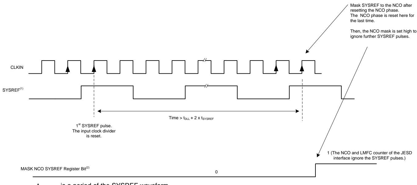
$t_{SYSREF}$  is a period of the SYSREF waveform.
