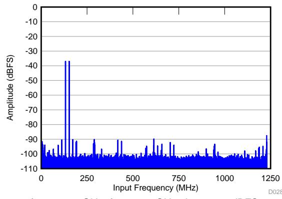
$f_{IN1} = 2.59$  GHz,  $f_{IN2} = 2.6$  GHz,  $A_{IN} = -36$  dBFS,
