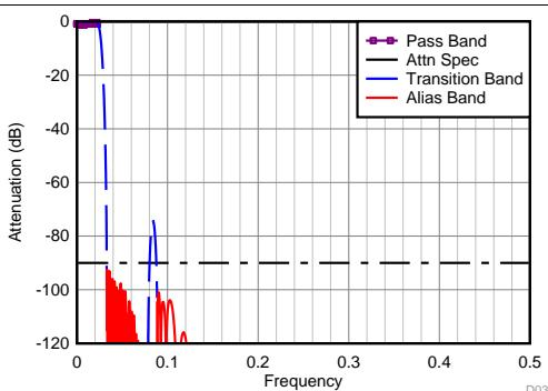
Figure 112. Divide-by-18 Filter Response
