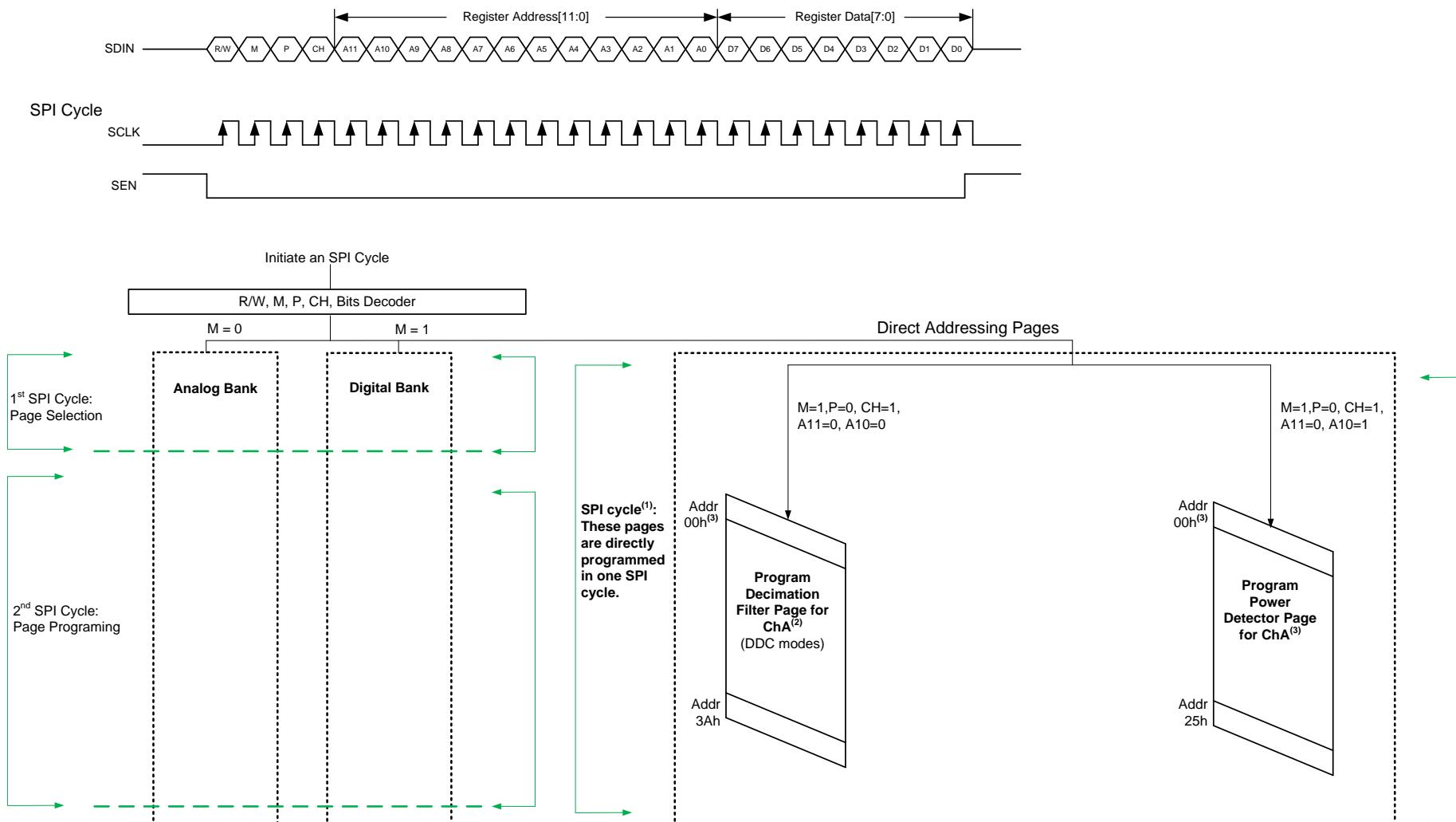
**Figure 143. SPI Registers: Direct Addressing**
