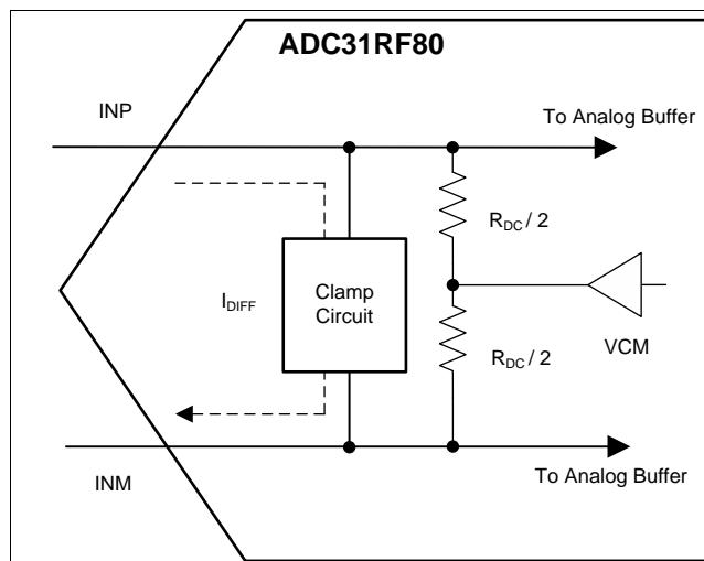
**Figure 85. Clamp Circuit in the ADC31RF80**
