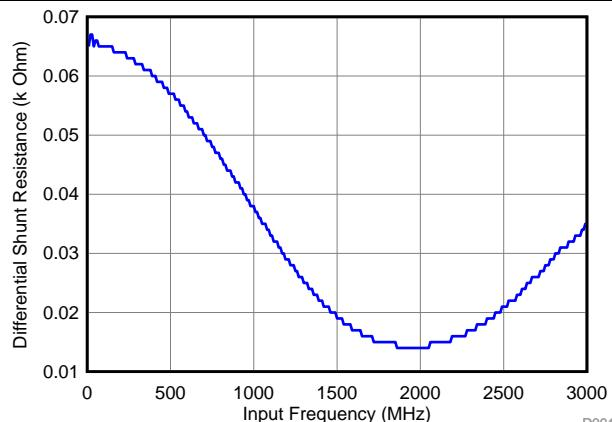
**Figure 83. Differential Input Resistance vs Input Frequency**
