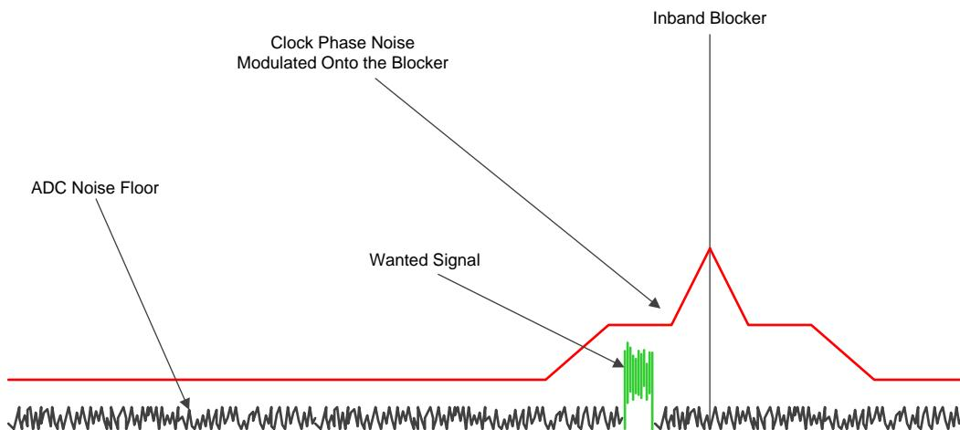
**Figure 265. Small Wanted Signal in Presence of Interferer**
