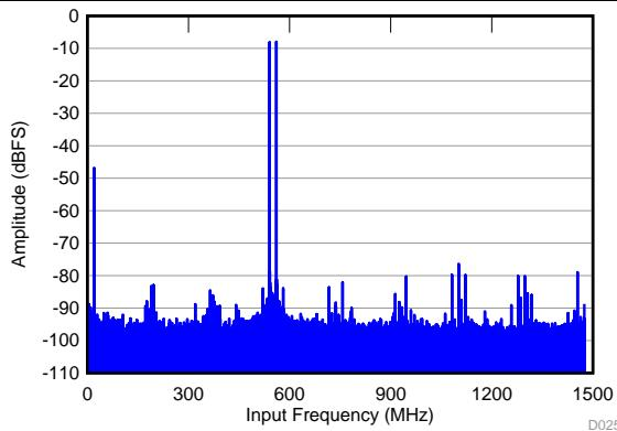
$f_{IN1} = 3.49$  MHz,  $f_{IN2} = 3.51$  GHz, IMD = 75 dBFS,
