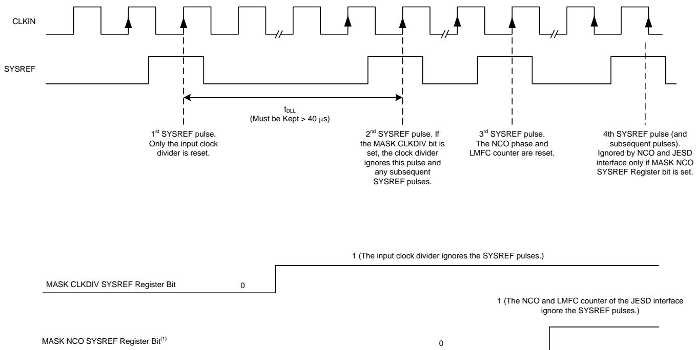
Alternatively, the SYSREF buffer can be powered down with the PDN SYSREF bit.
