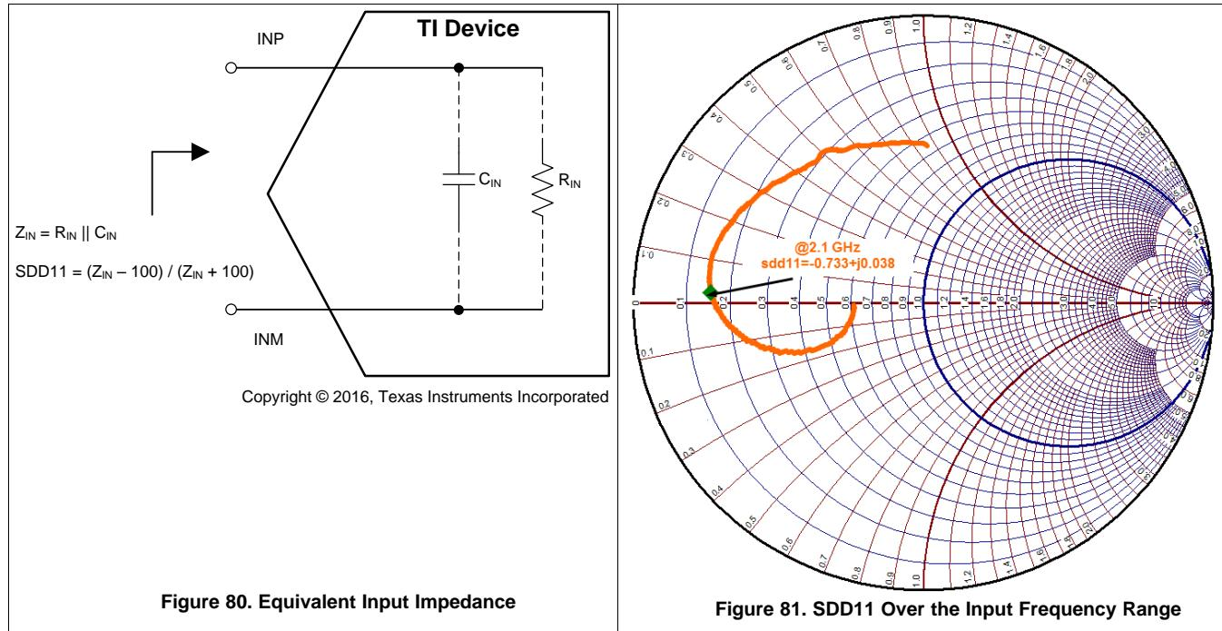
Figure 80. Equivalent Input Impedance
