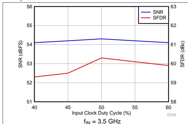
**Figure 63. Performance vs Clock Duty Cycle**
