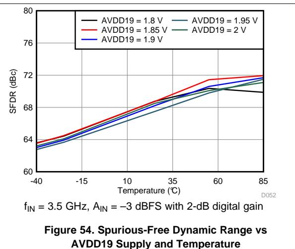
**Figure 54. Spurious-Free Dynamic Range vs AVDD19 Supply and Temperature**
