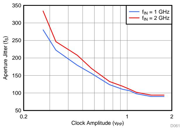
**Figure 88. Equivalent Aperture Jitter vs Input Clock Amplitude**
