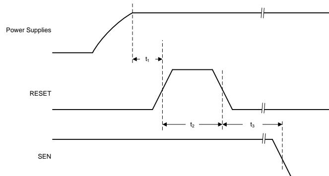
**Figure 262. Hardware Reset Timing Diagram**
