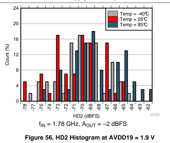
**Figure 56. HD2 Histogram at AVDD19 = 1.9 V**
