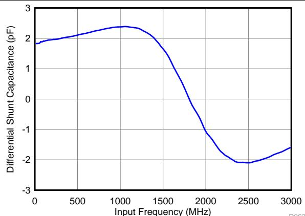
**Figure 82. Differential Input Capacitance vs Input Frequency**
