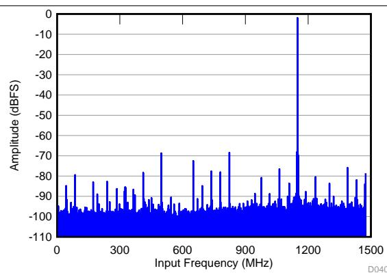
**Figure 64. Power-Supply Rejection Ratio FFT for Test Signal on AVDD Supply**
