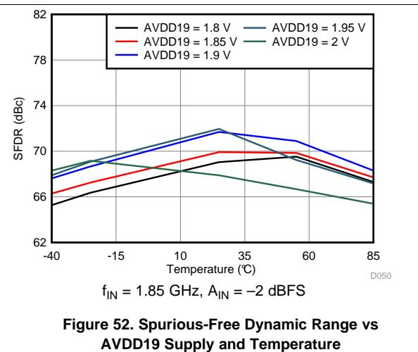
**Figure 52. Spurious-Free Dynamic Range vs AVDD19 Supply and Temperature**
