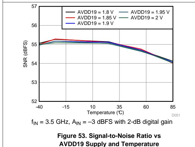
**Figure 53. Signal-to-Noise Ratio vs AVDD19 Supply and Temperature**
