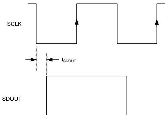
**Figure 135. SDOUT Timing**
