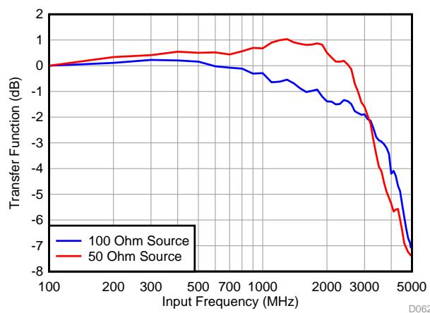
**Figure 84. Input Bandwidth with a  $100\text{-}\Omega$  Source Resistance**
