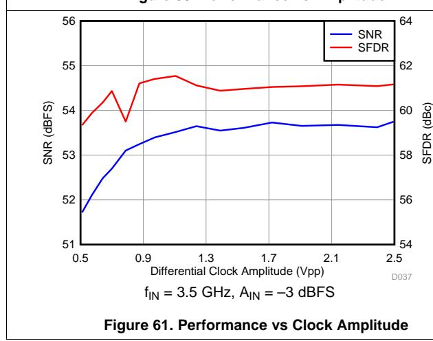
Figure 61. Performance vs Clock Amplitude
