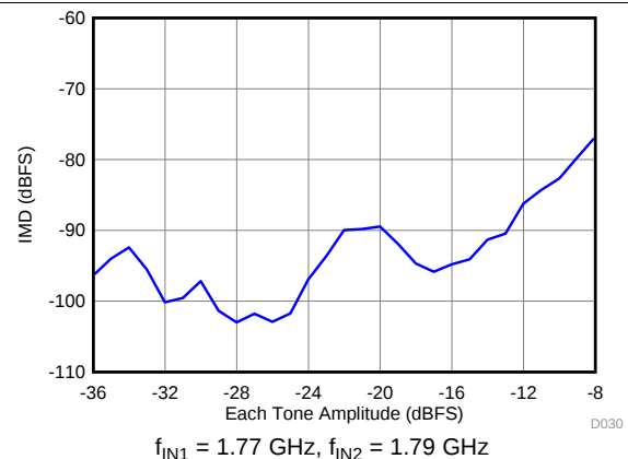
Figure 32. Intermodulation Distortion vs Input Amplitude (1770 MHz and 1790 MHz, f_s = 2457.6 \text{ MSPS} )
