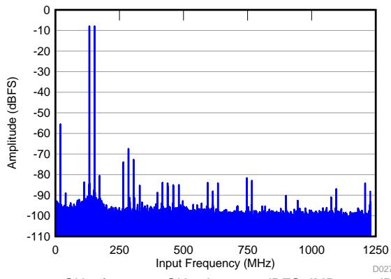
$f_{IN1} = 2.59$  GHz,  $f_{IN2} = 2.6$  GHz,  $A_{IN} = -8$  dBFS, IMD = 68 dBFS
