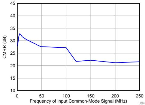
**Figure 67. Common-Mode Rejection Ratio vs Tone Frequency**
