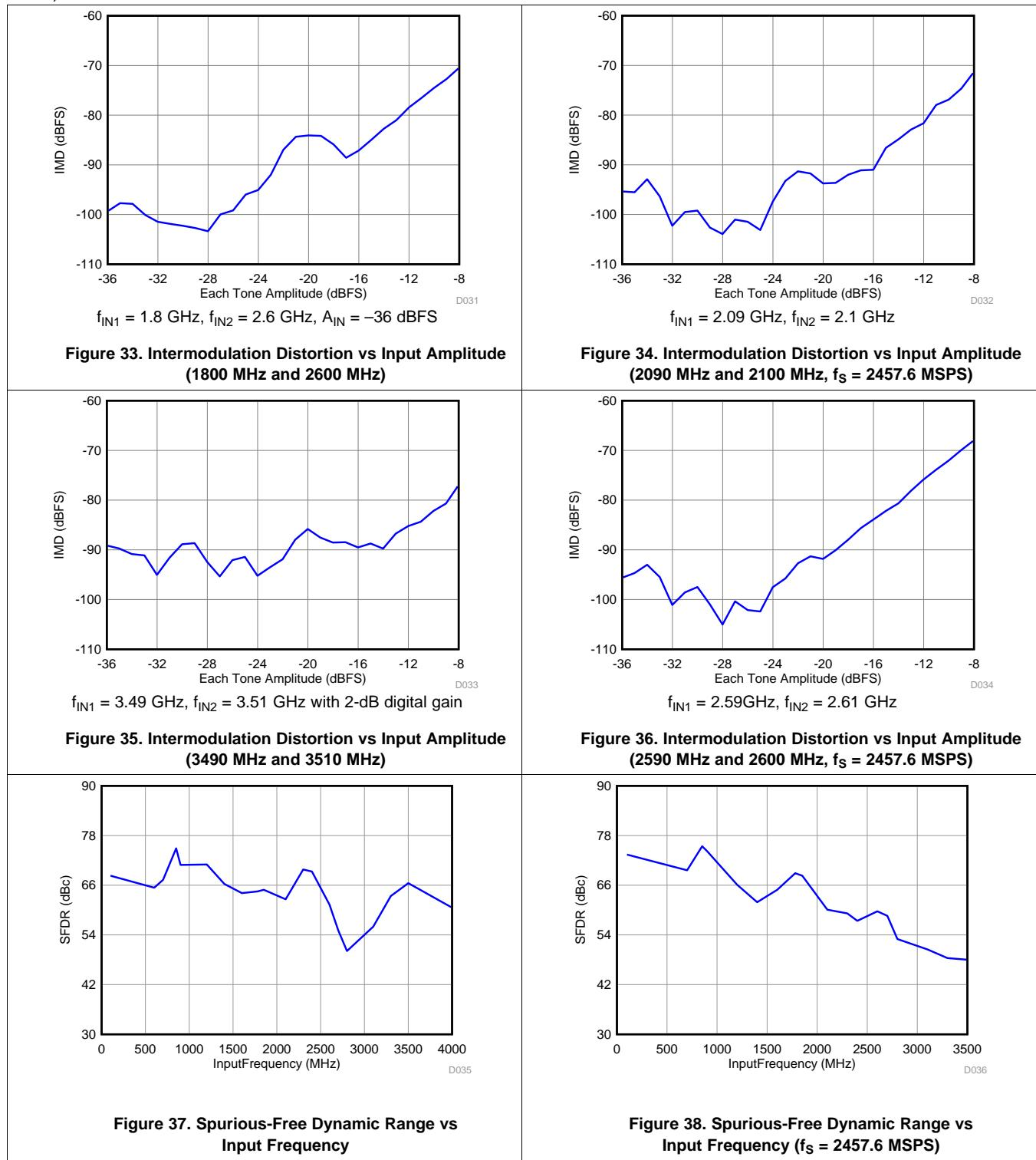
**Figure 33. Intermodulation Distortion vs Input Amplitude (1800 MHz and 2600 MHz)**
