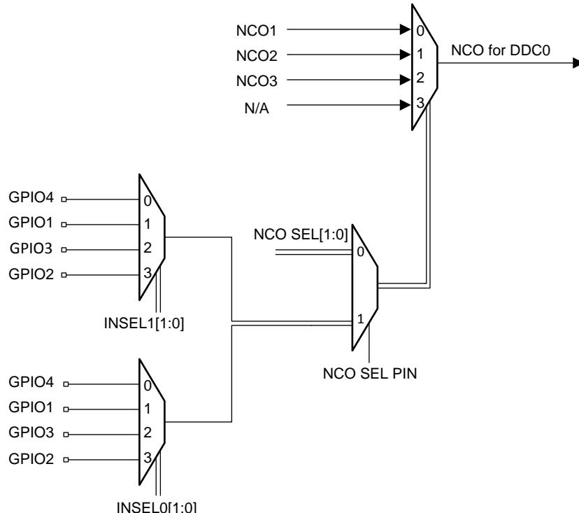
**Figure 120. NCO Switching from GPIO and SPI**
