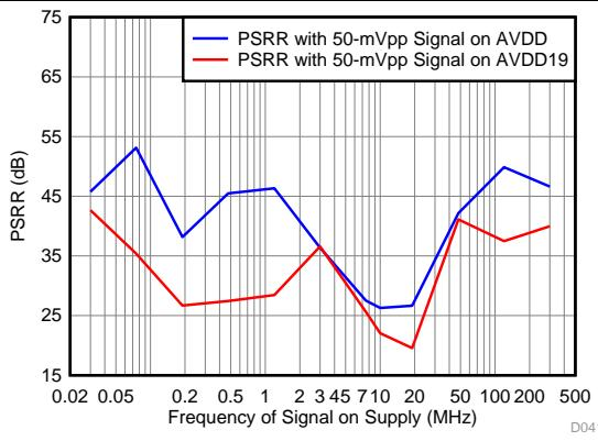
**Figure 65. Power-Supply Rejection Ratio vs Tone Frequency**
