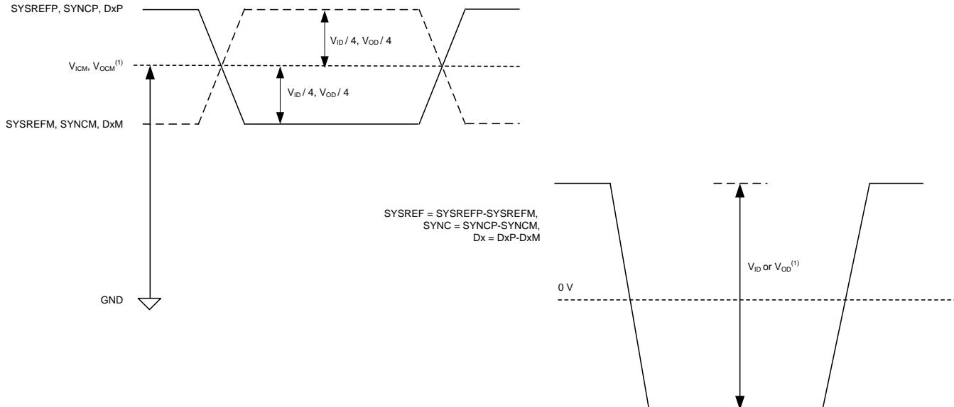
$V_{OCM}$  is not the same as  $V_{ICM}$ . Similarly,  $V_{OD}$  is not the same as  $V_{ID}$ .
