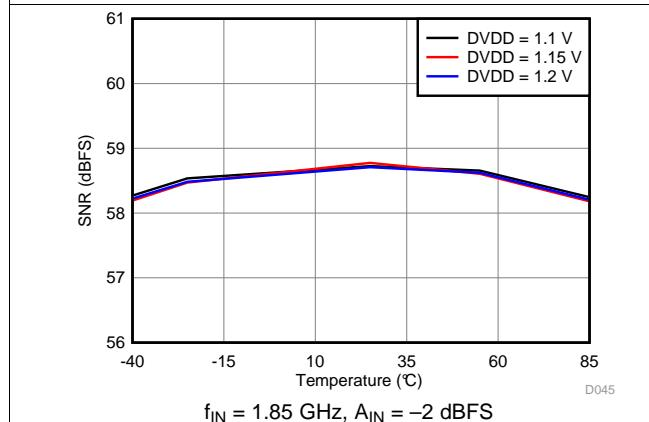
**Figure 47. Signal-to-Noise Ratio vs DVDD Supply and Temperature**
