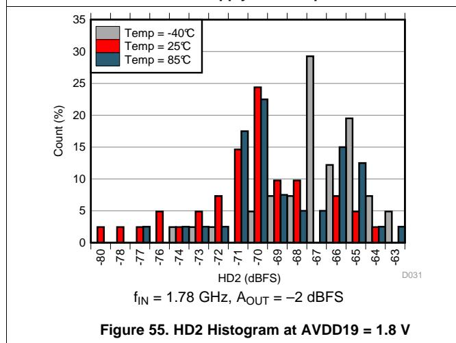
**Figure 55. HD2 Histogram at AVDD19 = 1.8 V**
