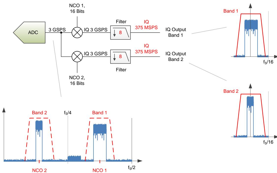
**Figure 96. Dual-Band Example**
