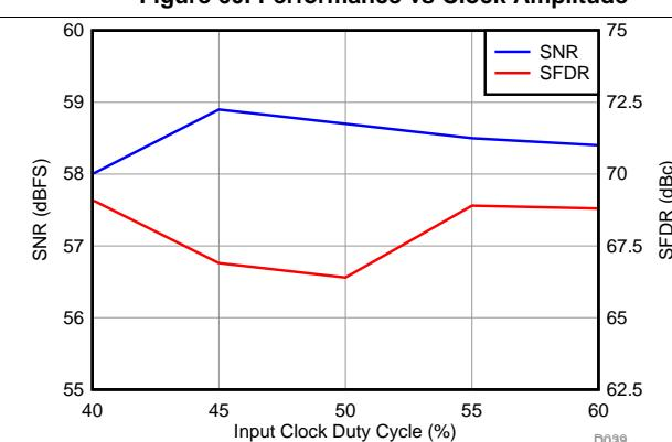
Figure 62. Performance vs Clock Duty Cycle
