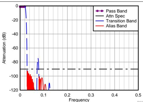
Figure 114. Divide-by-20 Filter Response
