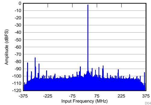
**Figure 68. FFT in 4x Decimation (Complex Output)**
