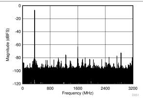
DES\_EN = 1, FG calibration,  $f_S$  = 6400 MSPS,  $f_1$  = 342 MHz,  $f_2$  = 352 MHz,  $A_{\text{IN}}$  = -7 dBFS per tone, SFDR = -73 dBFS, IMD3 = -81 dBFS, IMD2 = -88 dBFS
