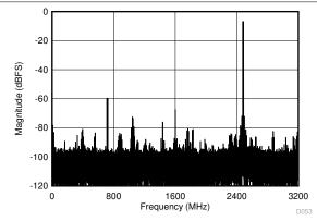
DES\_EN = 1, FG calibration,  $\rm f_S$  = 6400 MSPS,  $\rm f_1$  = 2483 MHz,  $\rm f_2$  = 2493 MHz,  $\rm A_{IN}$  = -7 dBFS per tone, SFDR = -60 dBFS, IMD3 = -72 dBFS, IMD2 = -78 dBFS
