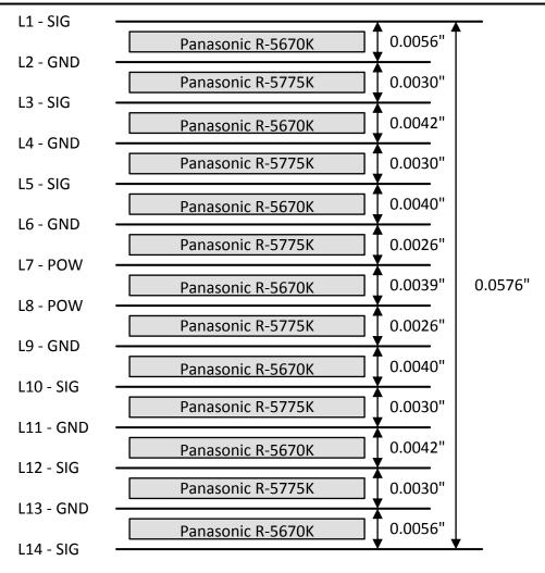
1/4 oz Copper on L1 and L14 \$1/2 oz Copper on L2, L3, L4, L5, L10, L11, L12 and L13 \$1 oz Copper on L6, L7, L8 and L9  $$100\text{-}\Omega$$  differential signaling on SIG layers Finished thickness is 0.0620" including plating and solder mask
