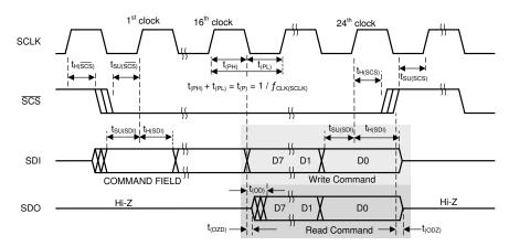
Figure 6-9. Serial Interface Timing
