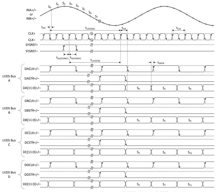
Figure 6-7. Single-Channel, 4-Bus, Aligned-Mode Timing (LDEMUX = 1, DES\_EN = 1, LALIGNED = 1)
