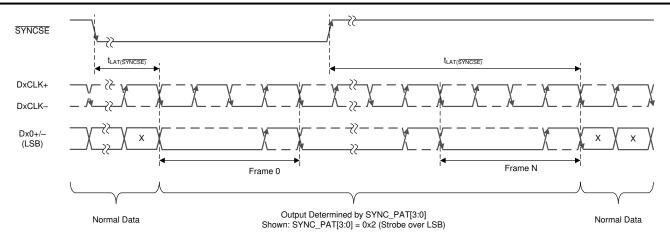
Figure 6-8. SYNCSE Timing Diagram
