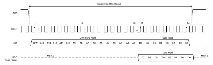
Figure 7-5. Serial Interface Protocol: Single Read/Write Operation
