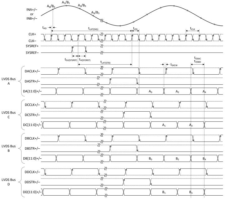
Figure 6-2. Dual-Channel, 4-Bus, Staggered-Mode Timing (LDEMUX = 1, DES\_EN = 0, LALIGNED = 0)
