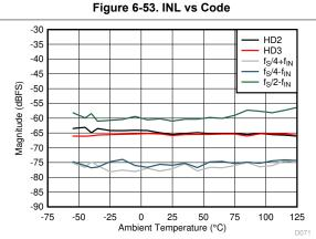
DES\_EN = 1, FG calibration,  $f_S$  = 6400 MSPS,  $f_{IN}$  = 2488 MHz,  $A_{IN}$  = -1 dBFS
