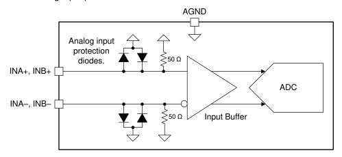
Figure 7-1. ADC12DL3200 Analog Input Internal Termination
