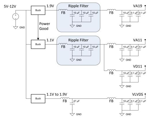
Ripple Filter Notch Frequency to Match Fs of Buck Converter FB = Ferrite Bead Filter
