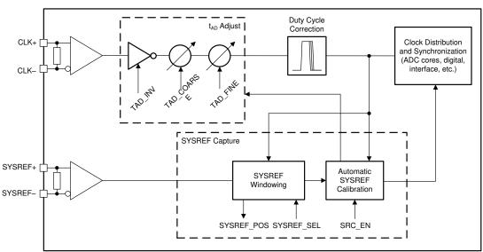
Figure 7-2. ADC12DL3200 Clocking Subsystem
