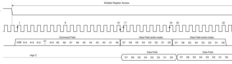
Figure 7-6. Serial Interface Protocol: Streaming Read/Write Operation
