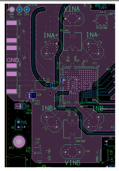
Figure 8-16. Bottom Layer Routing: Additional CLK Routing, DA4-7, DB4-7
