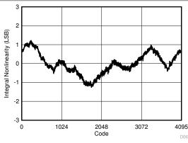
DES\_EN = 1, FG calibration,  $f_S$  = 6400 MSPS,  $f_{IN}$  = 247 MHz
