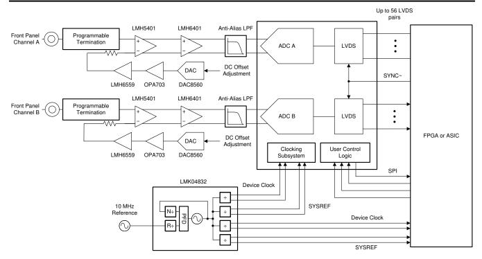
Figure 8-4. Typical Configuration for a Reconfigurable Oscilloscope
