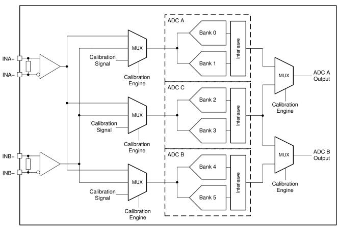
Figure 7-4. ADC12DL3200 Calibration System Block Diagram
