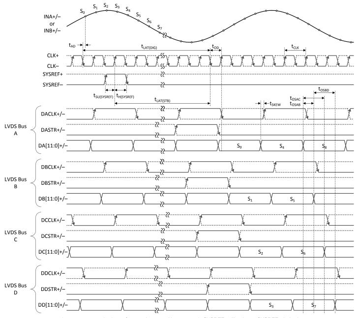
Figure 6-6. Single-Channel, 4-Bus, Staggered-Mode Timing (LDEMUX = 1, DES\_EN = 1, LALIGNED = 0)
