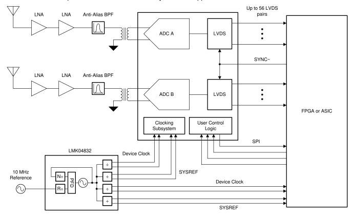
Figure 8-1. Typical Configuration for Wideband RF Sampling
