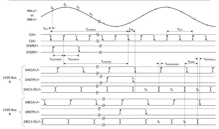
Figure 6-4. Single-Channel, 2-Bus, Staggered-Mode Timing (LDEMUX = 0, DES\_EN = 1, LALIGNED = 0)
