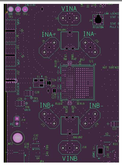
Figure 8-15. GND1 Cutouts to Optimize Impedance of Component Pads
