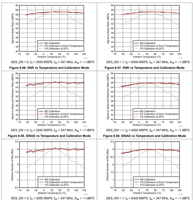
Figure 6-60. ENOB vs Temperature and Calibration Mode
