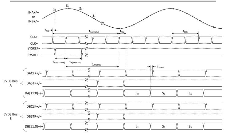
Figure 6-5. Single-Channel, 2-Bus, Aligned-Mode Timing (LDEMUX = 0, DES\_EN = 1, LALIGNED = 1)
