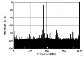
DES\_EN = 0, FG calibration,  $f_S$  = 3200 MSPS,  $f_1$  = 2483 MHz,  $f_2$  = 2493 MHz,  $A_{IN}$  = -7 dBFS per tone, SFDR = -71 dBFS, IMD3 = -71 dBFS, IMD2 = -75 dBFS
