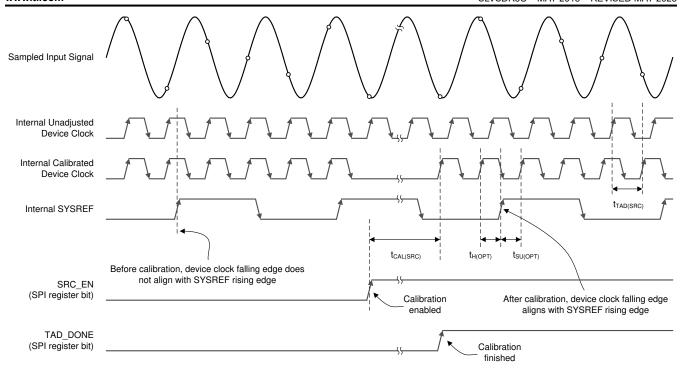
Figure 7-3. SYSREF Calibration Timing Diagram
