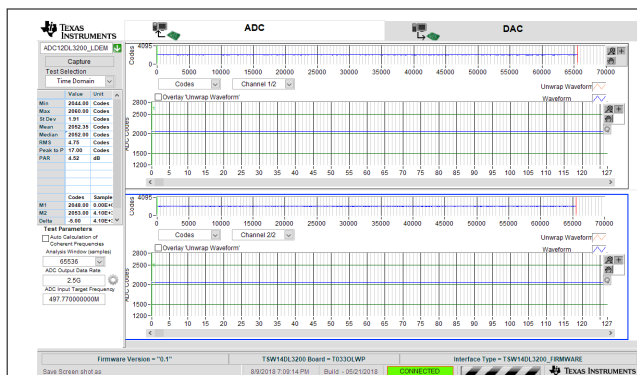
Figure 8-9. Idle-Channel Noise (No Input) for 2.5-GSPS, Dual-Channel Oscilloscope
