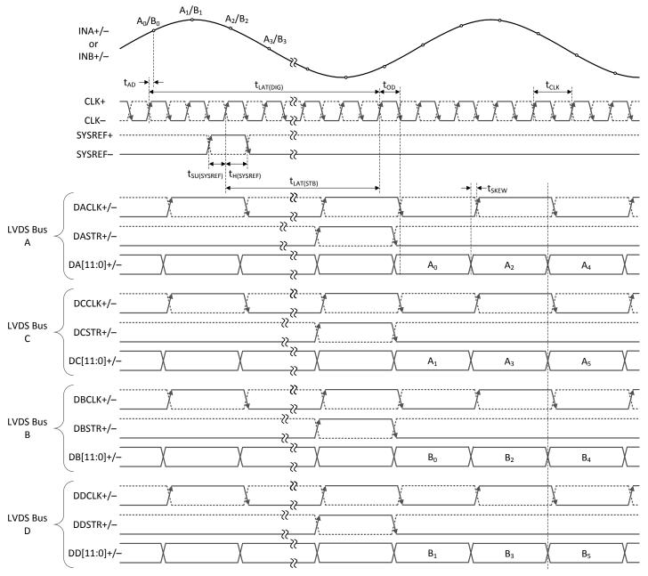
Figure 6-3. Dual-Channel, 4-Bus, Aligned-Mode Timing (LDEMUX = 1, DES\_EN = 0, LALIGNED = 1)
