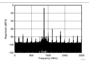
DES\_EN = 1, FG calibration,  $f_S$  = 6400 MSPS,  $f_1$  = 4992 MHz,  $f_2$  = 5002 MHz,  $A_{IN}$  = -7 dBFS per tone, SFDR = -60 dBFS, IMD3 = -62 dBFS, IMD2 = -78 dBFS
