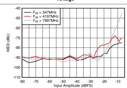
Figure 5-102. DES Mode: IMD3 vs Input Amplitude
