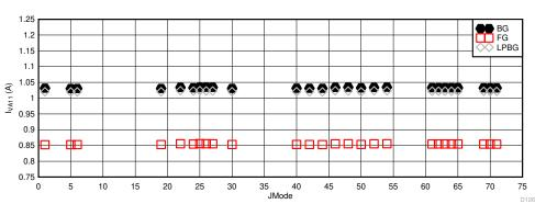
Figure 5-111. DES Mode: I<sub>VA19</sub> vs JMODE at 10.4GSPS
