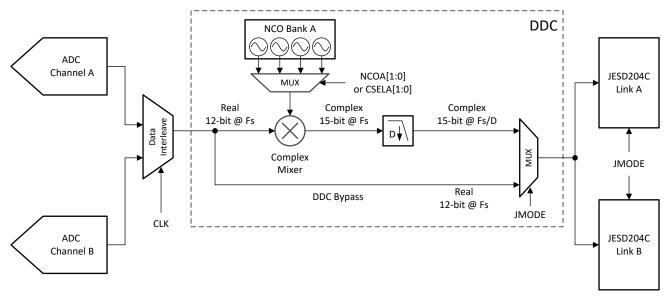
Figure 6-9. Digital Down Conversion Block in Single Channel Mode
