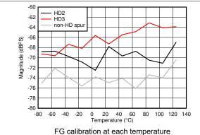
Figure 5-89. DES Mode: HD2, HD3 and Worst non-HD Spur vs
