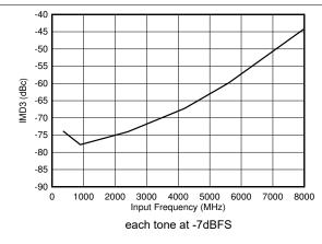
Figure 5-101. DES Mode: IMD3 vs Input Frequency
