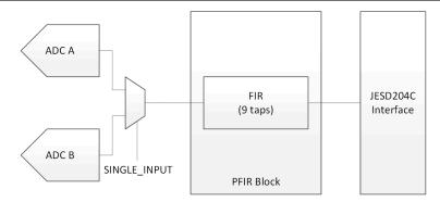
Figure 6-5. Single Channel Equalization PFIR Block Diagram
