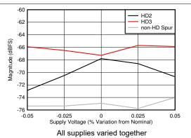
Figure 5-96. DES Mode: HD2, HD3 and Worst non-HD Spur vs Supply Voltage
