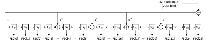
Figure 6-22. FEC Parity Bit Generator
