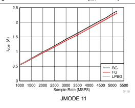
Figure 5-136. Dual Channel Mode: I<sub>VD11</sub> vs Sample Rate
