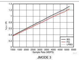
Figure 5-135. Dual Channel Mode: I<sub>VD11</sub> vs Sample Rate
