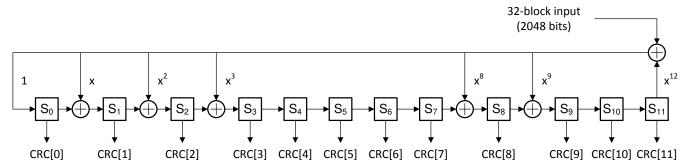
Figure 6-21. CRC-12 Parity Bit Generator
