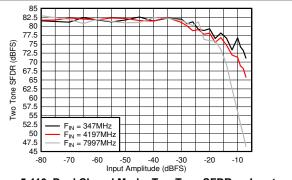
Figure 5-110. Dual Chanel Mode: Two Tone SFDR vs Input Amplitude
