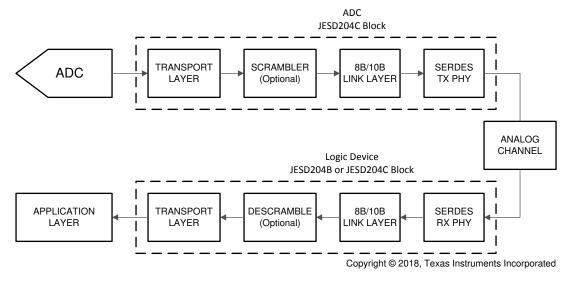
Figure 6-19. Simplified 8B/10B Encoded JESD204C Interface Diagram
