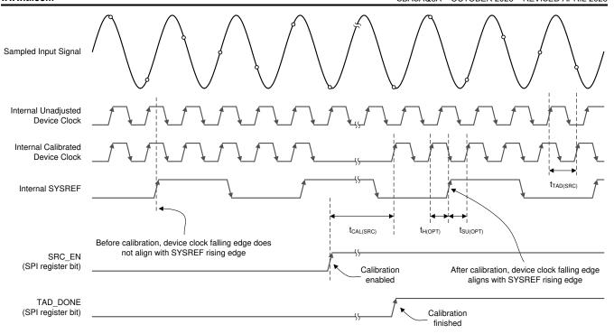
Figure 6-3. SYSREF Calibration Timing Diagram
