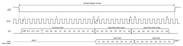
Figure 6-27. Serial Interface Protocol: Streaming Read/Write
