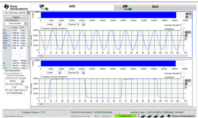
Figure 190. 200-MHz, Sine-Wave (Channel A) and 40-MHz, Square-Wave (Channel B) Time Domain for 5-GSPS, Single-Channel Oscilloscope
