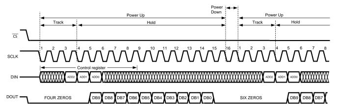
Figure 1. ADC108S102 Operational Timing Diagram
