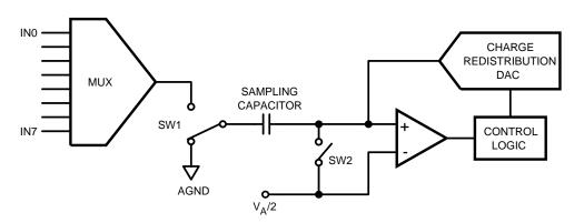
Figure 35. ADC108S102 in Hold Mode
