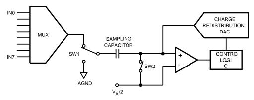
Figure 34. ADC108S102 in Track Mode
