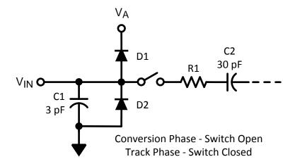
Figure 37. Equivalent Input Circuit
