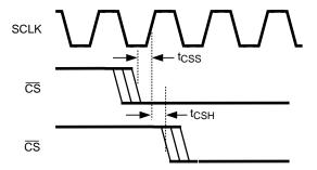
Figure 3. SCLK and CS Timing Parameters
