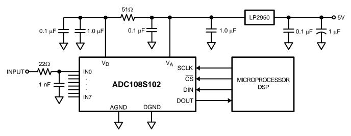
Figure 38. Typical Application Circuit
