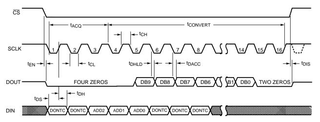
Figure 2. ADC108S102 Serial Timing Diagram
