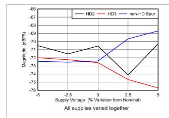
Figure 5-97. Dual Channel Mode: HD2, HD3 and Worst Spur vs Supply Voltage
