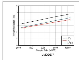
Figure 5-113. DES Mode: Power Dissipation vs Sample Rate
