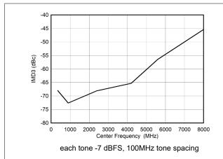
Figure 5-105. Dual Channel Mode: IMD3 vs Input Frequency
