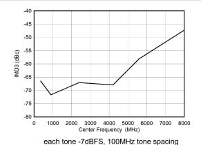
Figure 5-100. DES Mode: IMD3 vs Input Frequency
