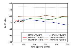
Figure 5-107. Dual Channel Mode: IMD3 vs Tone Spacing
