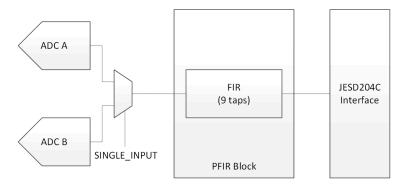
Figure 6-5. Single Channel Equalization PFIR Block Diagram
