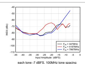
Figure 5-106. Dual Channel Mode: IMD3 vs Input Amplitude
