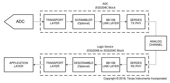
Figure 6-8. Simplified 8B/10B Encoded JESD204C Interface Diagram
