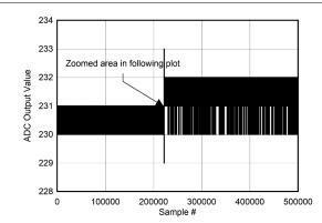
Figure 5-121. Background Calibration Core Transition (DC Signal)
