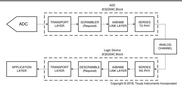
Figure 6-9. Simplified 64B/66B Encoded JESD204C Interface Diagram
