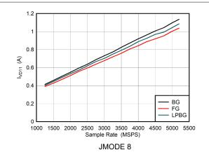
Figure 5-116. Dual Channel Mode: I<sub>VD11</sub> vs Sample Rate
