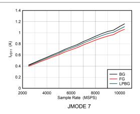
Figure 5-112. DES Mode: I<sub>VD11</sub> vs Sample Rate
