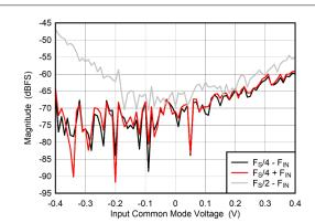
Figure 5-99. DES Mode:  $F_{\rm S}/2$ - $F_{\rm IN}$ ,  $F_{\rm S}/4$  +/- $F_{\rm IN}$  vs Input Common Mode Voltage
