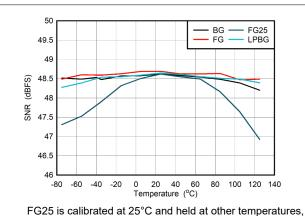
Figure 5-87. DES Mode: SNR vs Temperature and Calibration
