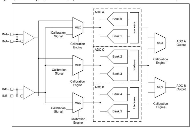
Figure 6-14. ADC08DJ5200RF Calibration System Block Diagram
