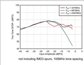
Figure 5-109. Dual Channel Mode: Two Tone SFDR vs Input Amplitude
