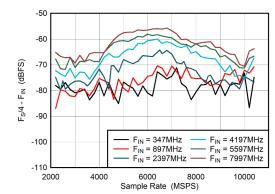
Figure 5-43. DES Mode: F<sub>S</sub>/4 - F<sub>IN</sub> vs Sample Rate
