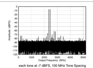
Figure 5-13. DES Mode: Two Tone FFT at 2397 MHz
