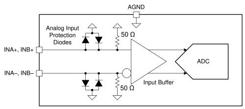
Figure 6-1. ADC08DJ5200RF Analog Input Internal Termination and Protection Diagram
