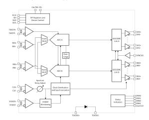
ADC08DJ5200RF Block Diagram
