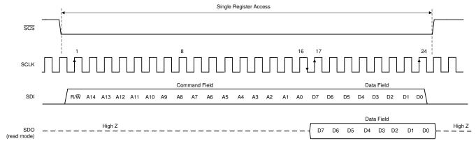
Figure 6-15. Serial Interface Protocol: Single Read/Write
