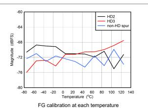
Figure 5-86. DES Mode: HD2, HD3 and Worst Spur vs
