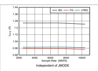
Figure 5-110. DES Mode: IVA19 vs Sample Rate
