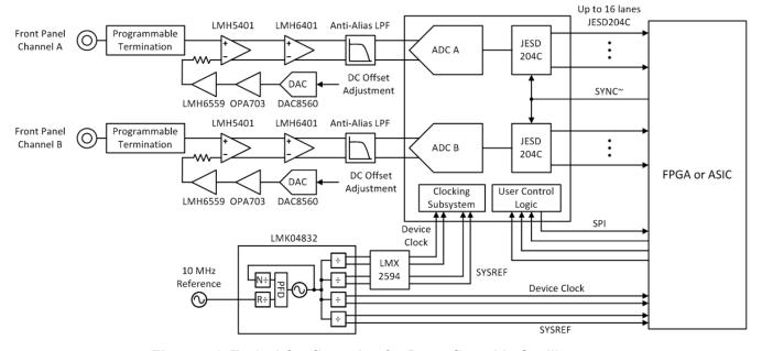
Figure 7-1. Typical Configuration for Reconfigurable Oscilloscope
