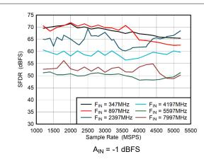
Figure 5-47. Dual Channel Mode: SFDR vs Sample Rate
