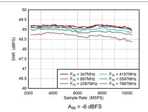
Figure 5-30. DES Mode: SNR vs Sample Rate
