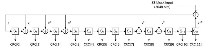
Figure 6-10. CRC-12 Parity Bit Generator
