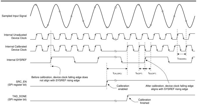
Figure 6-3. SYSREF Calibration Timing Diagram
