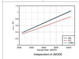
Figure 5-111. DES Mode: IVA11 vs Sample Rate
