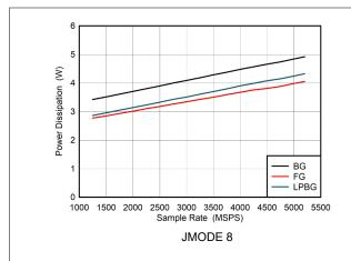
Figure 5-117. Dual Chanel Mode: Power Dissipation vs Sample Rate
