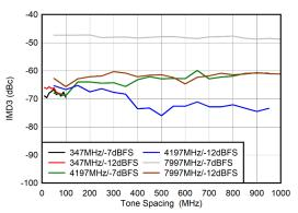
Figure 5-102. DES Mode: IMD3 vs Tone Spacing
