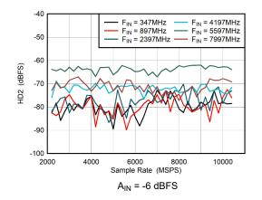
Figure 5-35. DES Mode: HD2 vs Sample Rate
