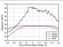
Figure 5-98. DES Mode: SNR, SFDR and SINAD vs Input Common Mode Voltage
