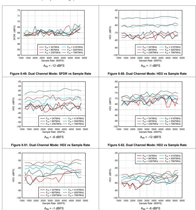
Figure 5-53. Dual Channel Mode: HD3 vs Sample Rate
