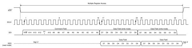
Figure 6-16. Serial Interface Protocol: Streaming Read/Write
