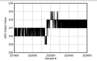
Figure 5-122. Background Calibration Core Transition (DC Signal Zoomed)
