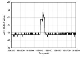
Figure 5-120. Background Calibration Core Transition (AC Signal Zoomed)
