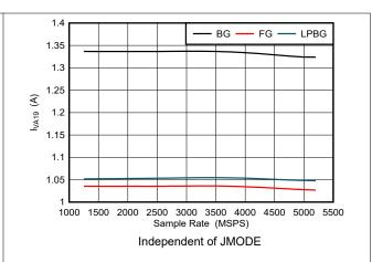
Figure 5-114. Dual Channel Mode:  $I_{VA19}$  vs Sample Rate
