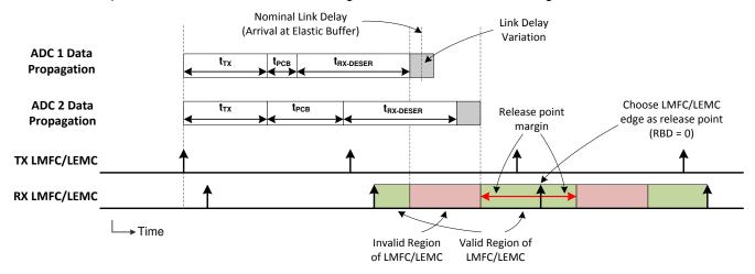
Figure 6-12. LMFC/LEMC Valid Region Definition for Elastic Buffer Release Point Selection
