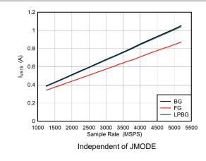
Figure 5-115. Dual Channel Mode: I<sub>VA11</sub> vs Sample Rate
