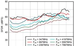
Figure 5-32. DES Mode: SFDR vs Sample Rate
