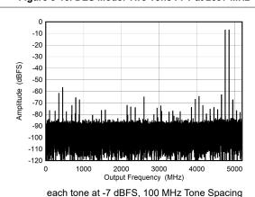
Figure 5-15. DES Mode: Two Tone FFT at 5597 MHz
