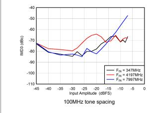
Figure 5-101. DES Mode: IMD3 vs Input Amplitude
