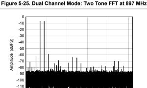
1000 1500 Output Frequency (MHz) each tone at -7 dBFS, 100 MHz Tone Spacing
