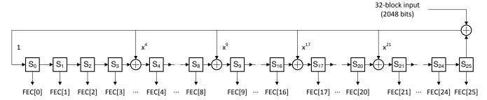
Figure 6-11. FEC Parity Bit Generator
