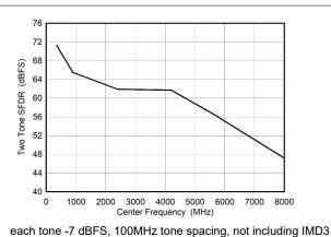
Figure 5-103. DES Mode: Two Tone SFDR vs Input Frequency
