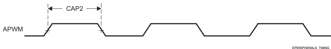
Figure 6-17. ECAP Switching Characteristics
