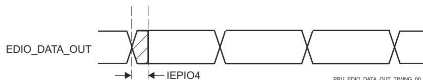
Figure 6-76. PRU-ICSS IEP Digital IOs Timing Requirements
