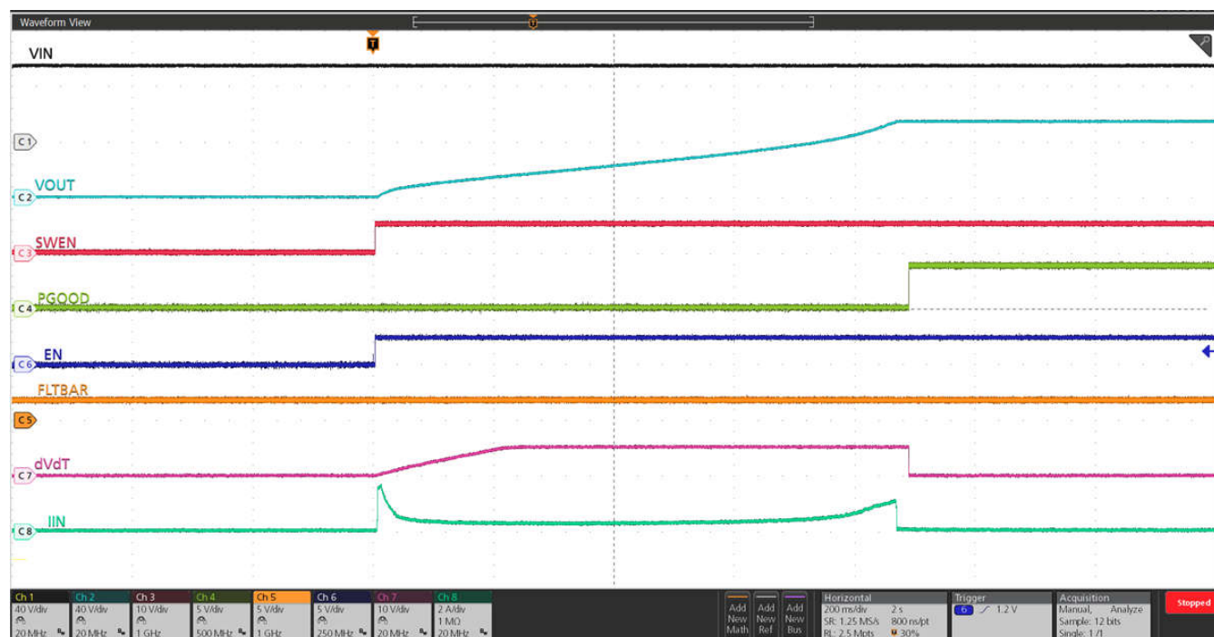
Figure 3-8. Power-Up Using ENABLE With Six Devices in Parallel (Condition 1)
