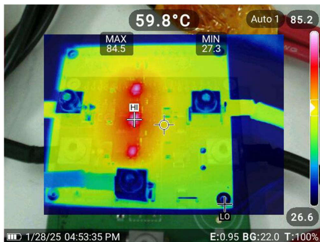
Figure 3-16. Thermal Performance With Six Devices in Parallel
