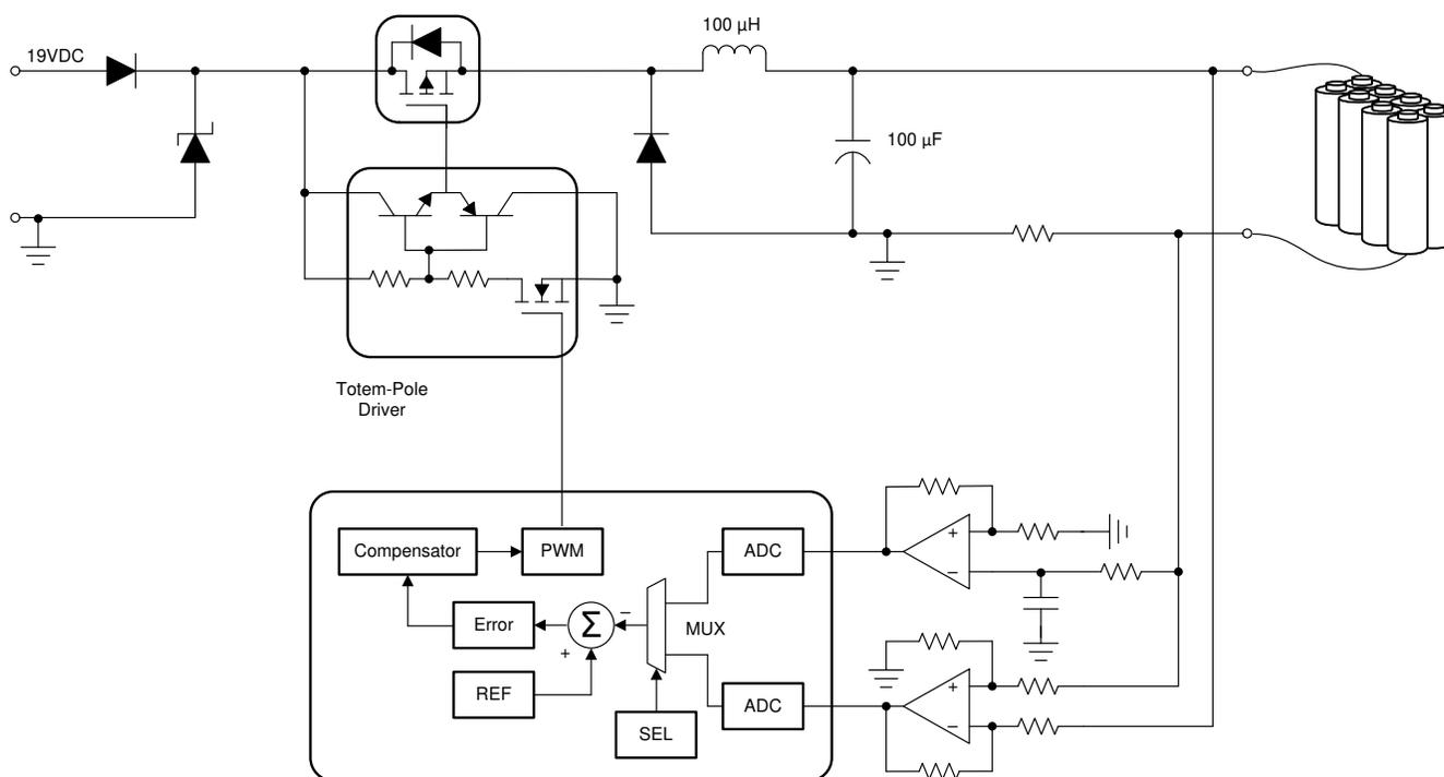
**Figure 1-1. Asynchronous Buck Topology Charger Controlled by System MCU**
