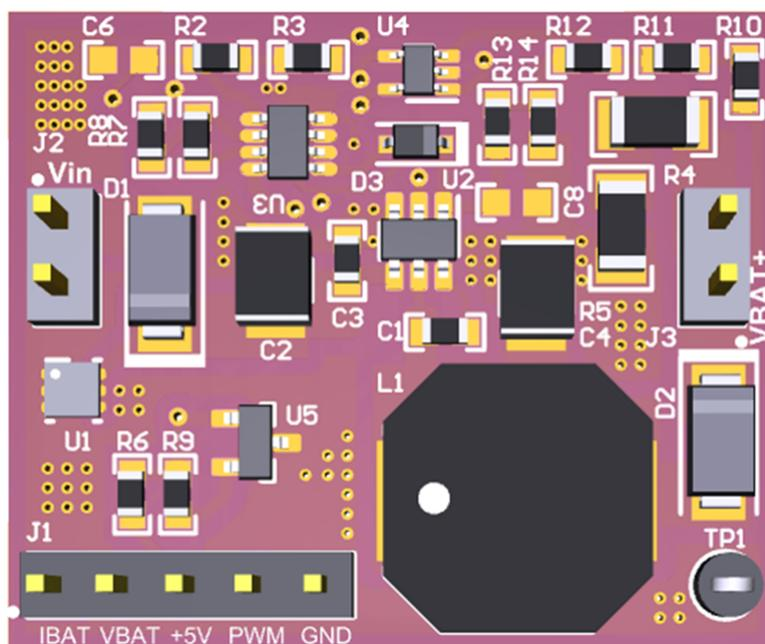
**Figure 3-1. TIDA-050042 Printed-Circuit Board**
