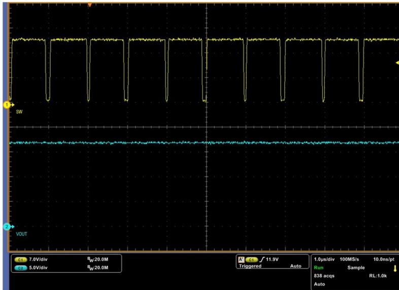
Figure 3-4. CV Mode Steady State
