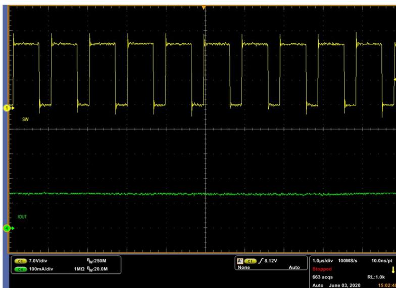
Figure 3-2. Pre-Charging Mode Steady State
