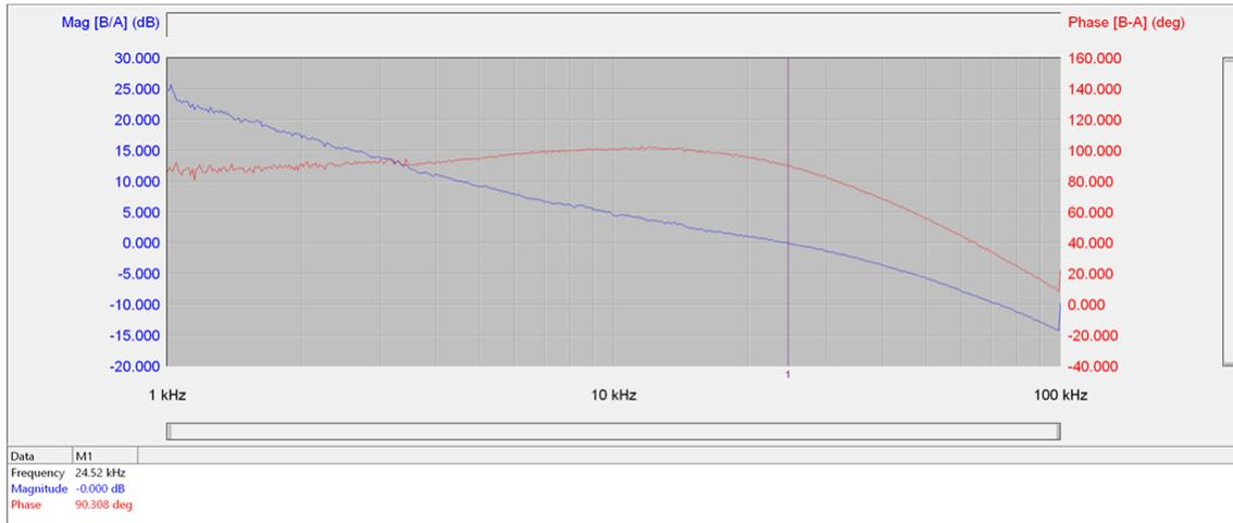
**Figure 3-10. Current Open Loop Stability**
