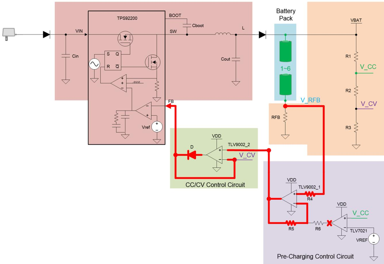
**Figure 2-4. Constant Current Control Design**
