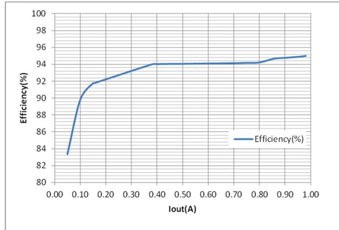
**Figure 3-7. Efficiency Versus Output Current**
