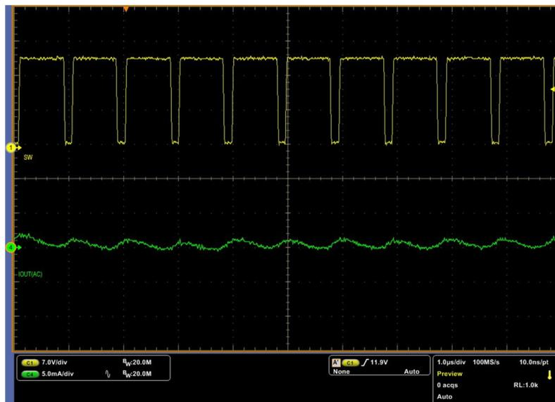
Figure 3-5. CC Mode Current Ripple
