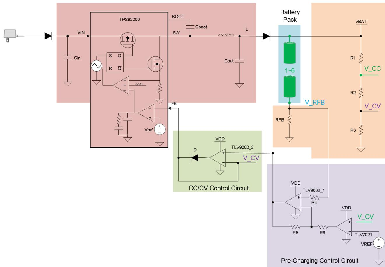
Figure 2-1. TIDA-050042 Block Diagram
