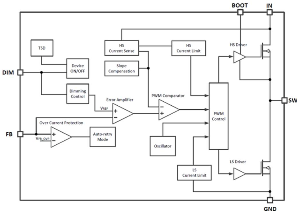
Figure 2-2. TPS92200 Functional Block Diagram
