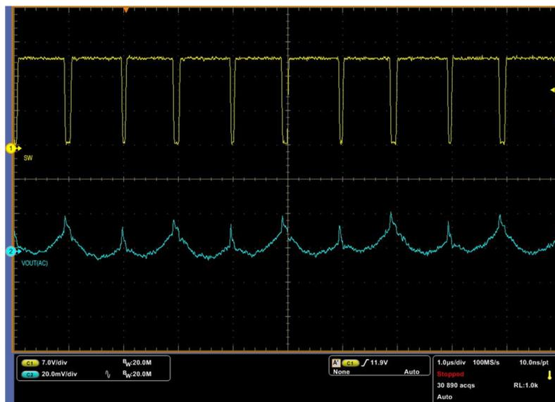
Figure 3-6. CV Mode Voltage Ripple
