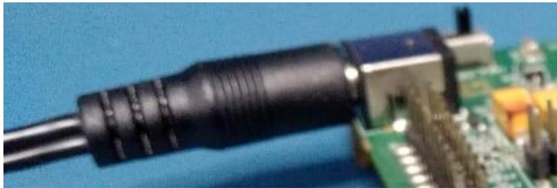
**NOTE:** Power supplies other than the SMI24-5-V-P6 may be substituted if the DC output voltage, current rating, polarity, and barrel jack size (inside diameter and outside diameter) are equivalent. Power supplies with DC voltage greater than 5.25V are not acceptable because of the over voltage protection circuit on the board which is intended to prevent damage to the ICs.
