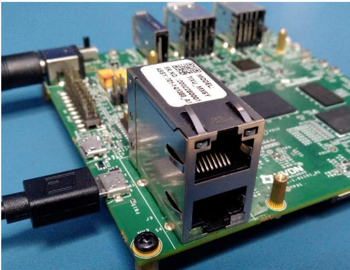
Use TeraTerm or Putty to open a Terminal and get the debug log from the device node if the host PC is running Windows. Change port number according to the COMx port found in Device Manager for the FTDI chip.
