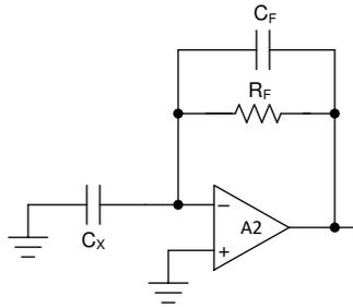
**Figure 2-5. Capacitor Measurement Circuit w/ Compensation Capacitor**
