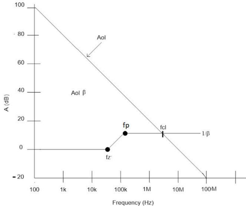
**Figure 2-8. Bode Plot of Capacitive Measurement with Series Resistance**
