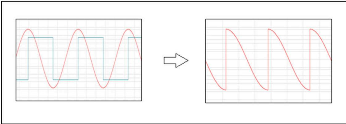
**Figure 2-11. Square Wave Modulation with 90° phase**
