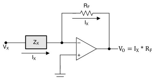
**Figure 1-1. Auto Balancing Circuit Amplifier Configuration**
