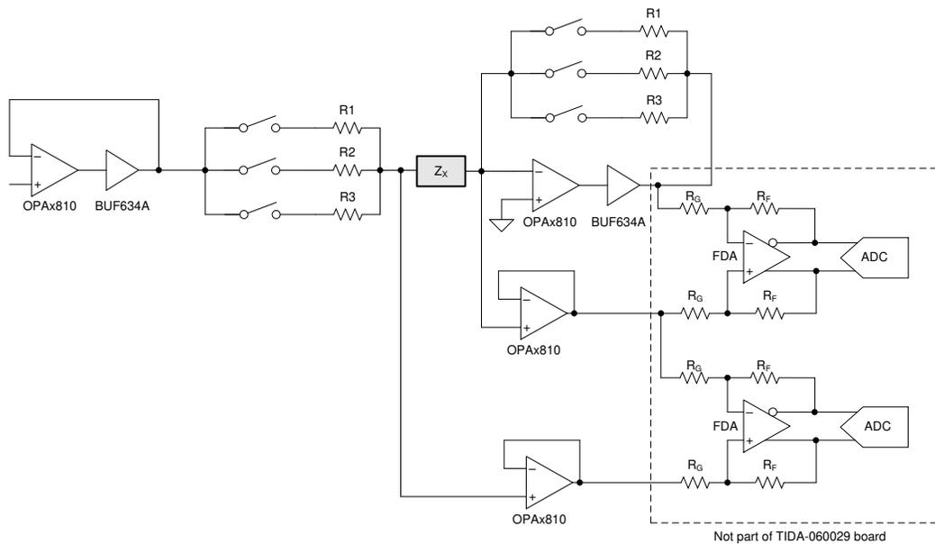
Figure 2-1. TIDA-060029 Block Diagram
