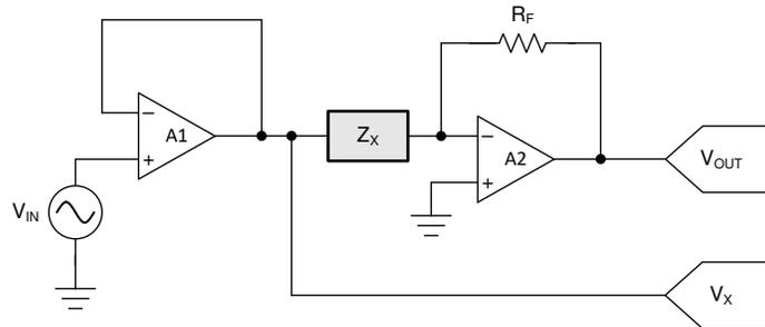
**Figure 2-2. Basic Impedance Measurement Circuit**
