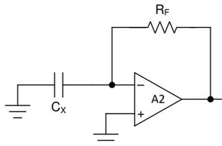
**Figure 2-3. Capacitor Measurement Circuit**
