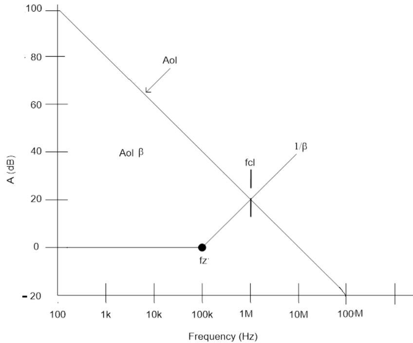
**Figure 2-4. Bode Plot of Capacitor Measurement**
