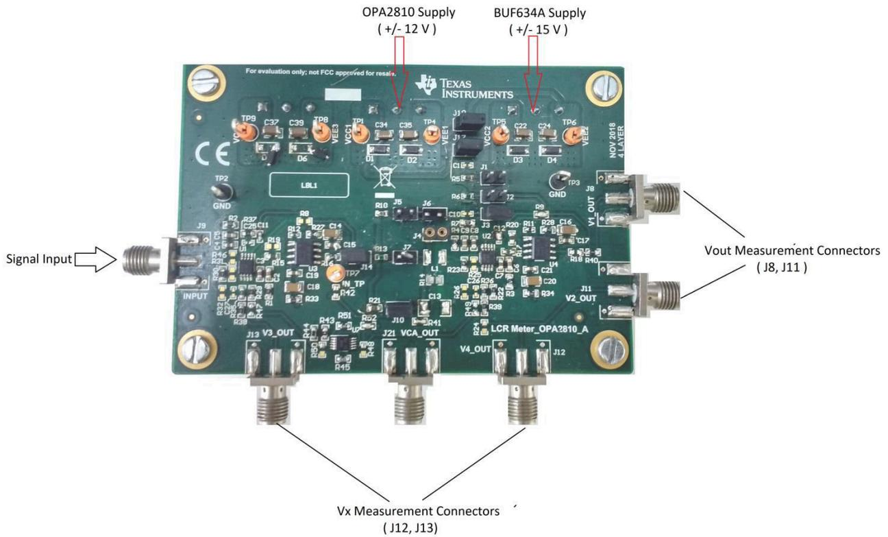
**Figure 3-2. Board Connections**
