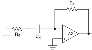
Figure 2-7. Capacitive Measurement with Series Resistance
