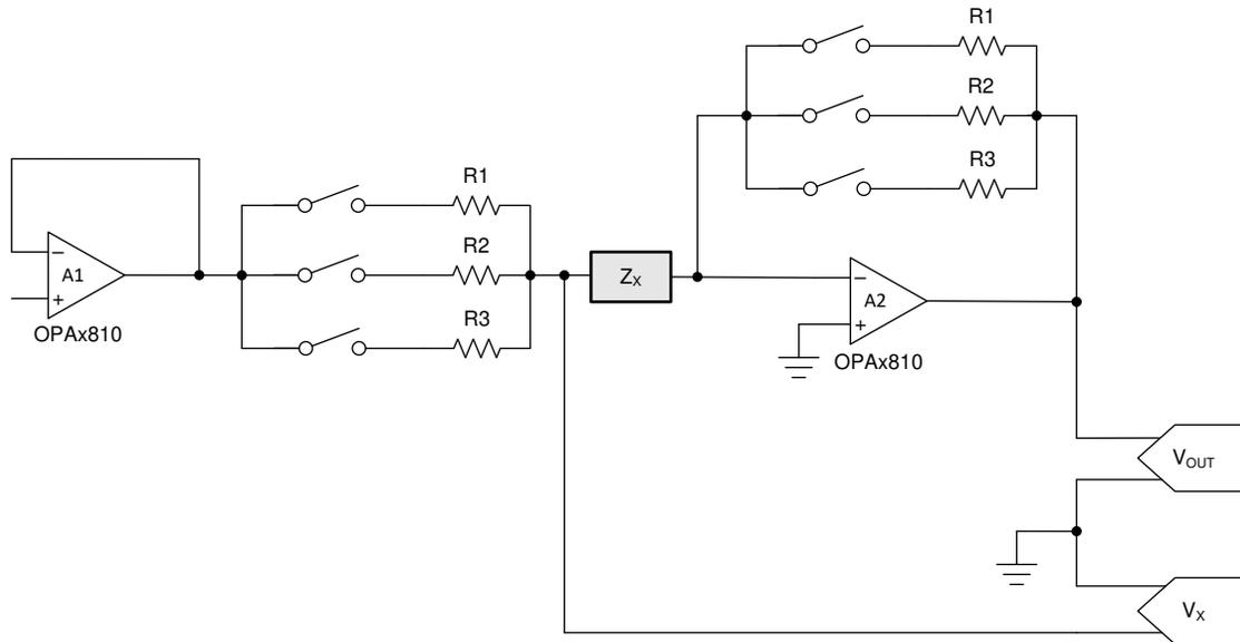
Figure 2-6. Impedance Measurement Design
