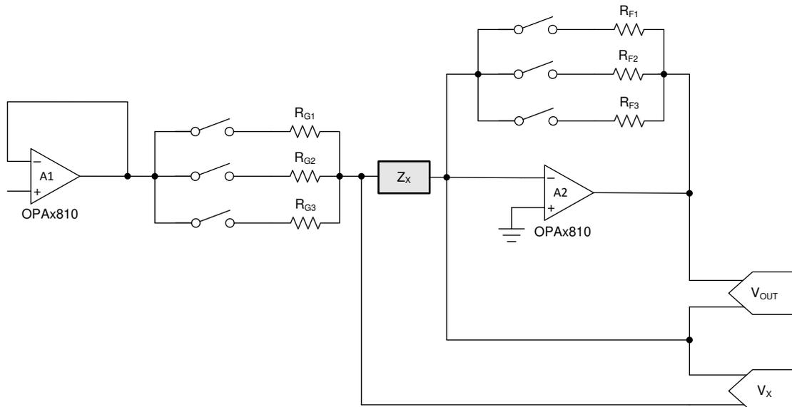
Figure 2-9. Method 1 of Impedance Measurement
