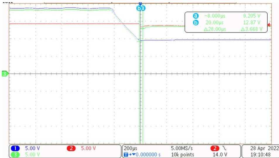
Figure 3-1. 19 V to Battery Switchover 200- $\mu$ s Time Division
