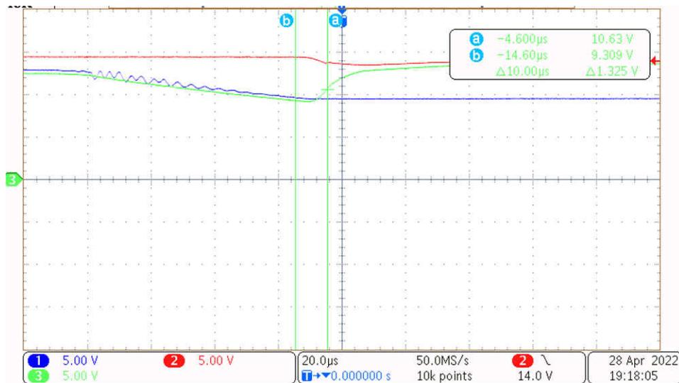
**Figure 3-4. 12 V to Battery Switchover 20- $\mu$ s Time Division**
