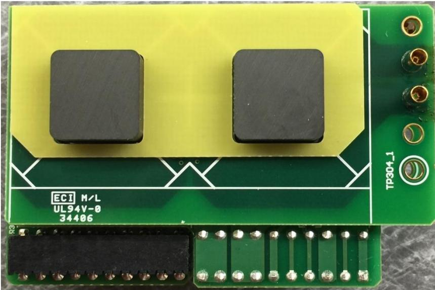
**Step 10:** Apply Winding\_Sec1 board on top of Winding\_Gap board placed as shown below. Then apply the assembled PCB windings and the U core to PMP20978 load card Rev A board as shown below. Then apply Mill-Max pins (P/N: 3106-2-00-15-00-00-08-0) to pin receptacles on Winding\_Pri1 through Winding\_Pri4 Steps 1 through 10 complete the transformer assembly.
