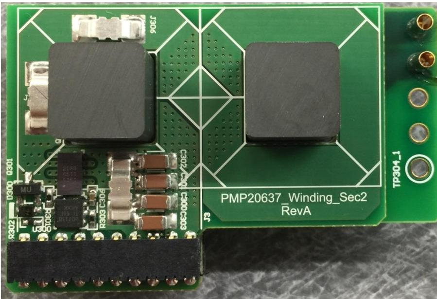
**Step 8:** Apply another Winding\_Sec2 board on top of the Winding\_Sec2 board placed in step 7 back to back as shown below. Then apply Winding\_Gap board on top of the Winding\_Sec2 board as shown below.
