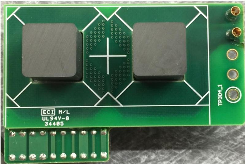
**Step 7:** Apply Winding\_Gap board on top of Winding\_Pri1 board as shown below. Then apply Winding\_Sec2 board on top of Winding\_Gap board as shown below.
