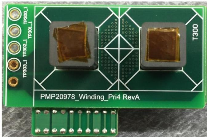
Step 2: Apply Winding\_Gap board on top of Winding\_Pri4 board as shown below. Then apply Winding\_Sec2 board on top of Winding\_Gap board as shown below.
