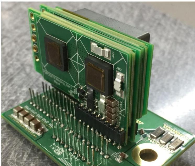
**Step 6:** Apply Winding\_Sec1 and Winding\_Gap boards to the U core as shown below.
