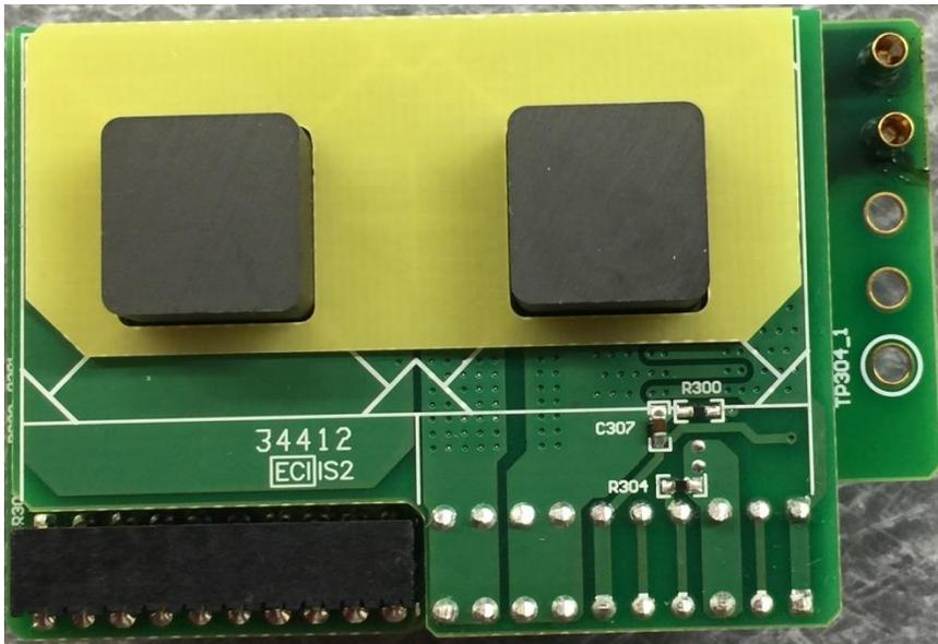
**Step 9:** Apply Winding\_Pri2 board on top of Winding\_Gap board placed as shown below. Then apply Winding\_Gap on top of the Winding\_Pri2 board as shown below.
