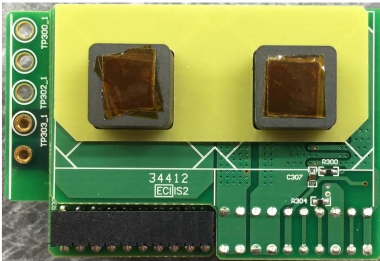
**Step 4:** Apply Winding\_Pri3 board on top of Winding\_Gap board placed as shown below. Then apply Winding\_Gap on top of the Winding\_Pri3 board as shown below.
