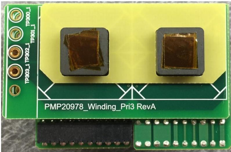
**Step 5:** Apply Winding\_Sec1 board on top of Winding\_Gap board placed as shown below. Then apply the assembled PCB windings and the U core to PMP20978 load card Rev A board as shown below. Steps 1 through 5 complete half of the transformer assembly.
