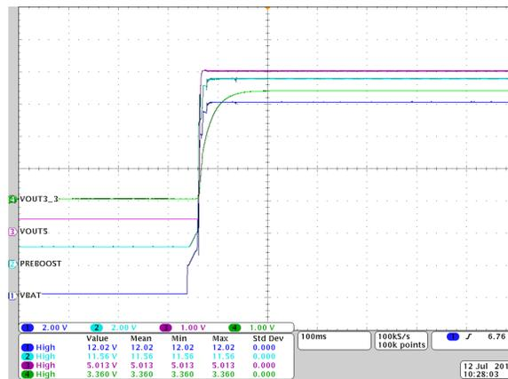
[Figure 26](#) shows the output voltages and the performance of the LM5150-Q1 pre-boost. To minimize output undershoot when waking up, the LM5150-Q1 boosts the  $V_{OUT}$  regulation target during the first 128 cycles after the wake-up event.
