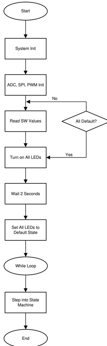
Figure 23. TIDA-01628 State Machine Transition Graph
