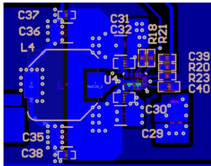
4.3.3.3 LM43602-Q1 3.3 V Buck Converter Layout
