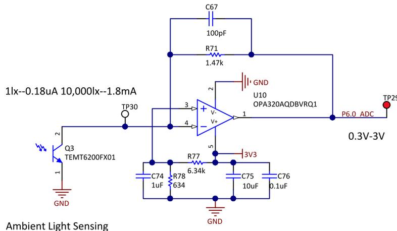
This design, as Figure 16 shows, uses a 10:1 resistor divider to get a 0.3-V bias, which is sufficient for the OPA320-Q1 device to get an accurate conversion result. The basic characteristics of the TEMA6200FX01 show that the maximum photo current under 10 k Lux is about 1.8 mA and 0.18  $\mu$ A under 1 Lux. The gain resistor R71 can be defined by: Equation 3.
