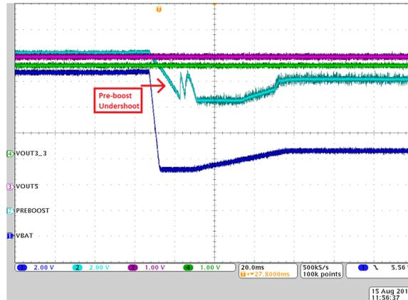
Figure 27 shows TIDA-01628 still outputting the proper voltage rails even as it undergoes cold cranking conditions and  $V_{IN}$  drops to 3.5 V. During cold cranking and initial VBAT voltage drop to 3.5 V, the pre-boost minimizes its output undershoot (similar to Figure 26) and when the VBAT voltage goes from 6.5 V to 8.5 V, pre-boost goes into standby mode to conserve battery.
