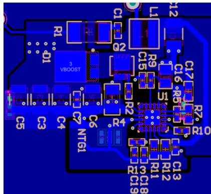
4.3.3.2 LMR33630-Q1 5-V Buck Converter Layout
