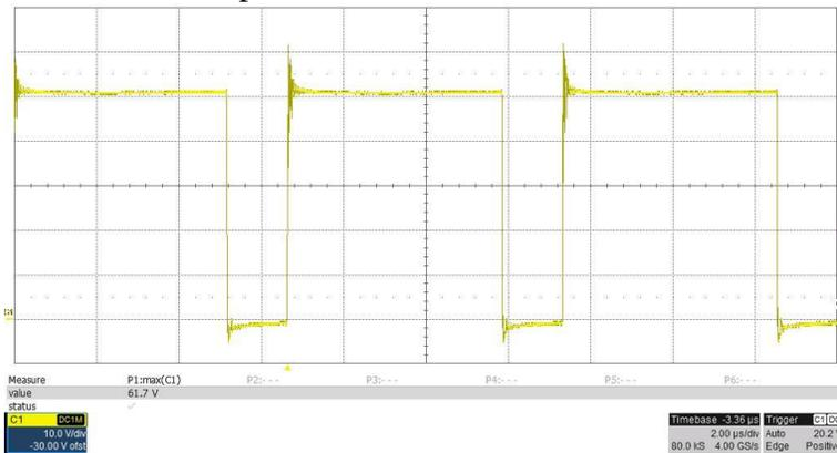
Vanode-GND, D8, 100V/div, 2usec/div, 40VDC input, 750MHz bandwidth
