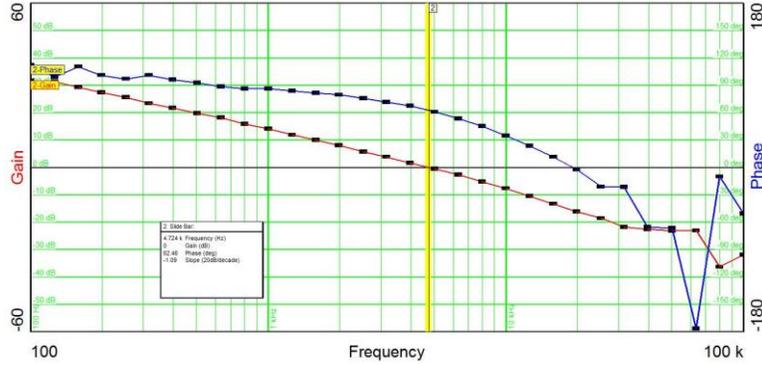
Bandwidth= 4.7 kHz Phase Margin=62 degrees Gain Margin=16dB
