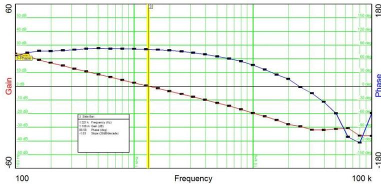
Bandwidth= 1.3 kHz Phase Margin=80 degrees Gain Margin=29dB
