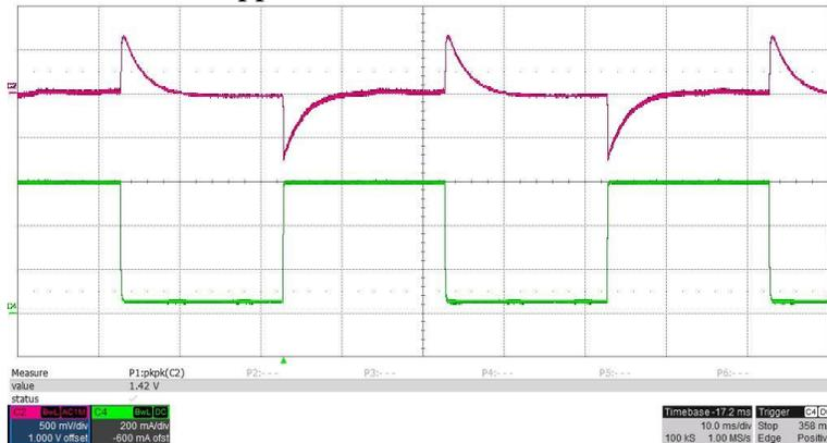
Output load step response, 300mA to 600mA load step, 24VAC input
