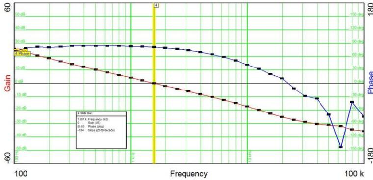
Bandwidth= 1.6 kHz Phase Margin=80 degrees Gain Margin=27dB
