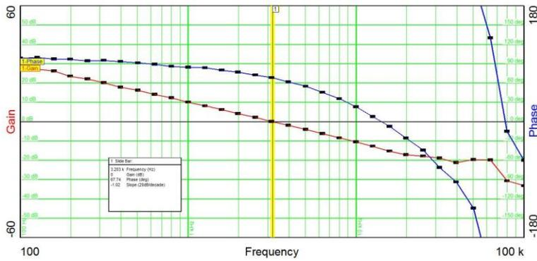
Bandwidth= 3.2 kHz Phase Margin=67 degrees Gain Margin=13dB
