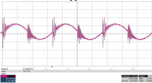
Input ripple, 12VDC input
