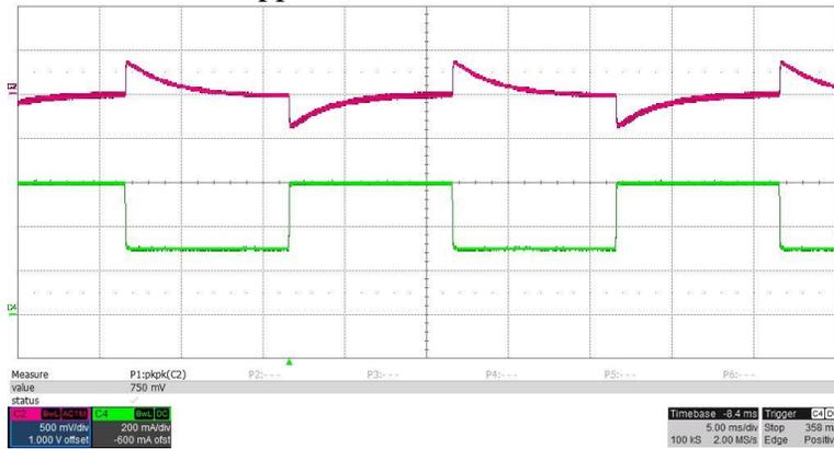
Output load step response, 60mA to 600mA load step, 24VAC input
