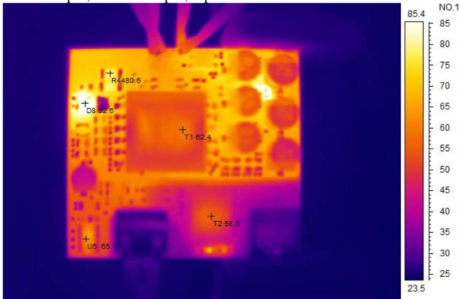
12VDC input, 600mA output, bottom:
