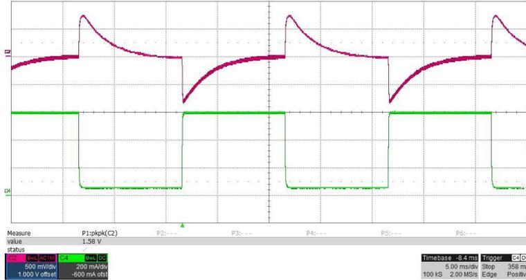
Output load step response, 300mA to 600mA load step, 12VDC input
