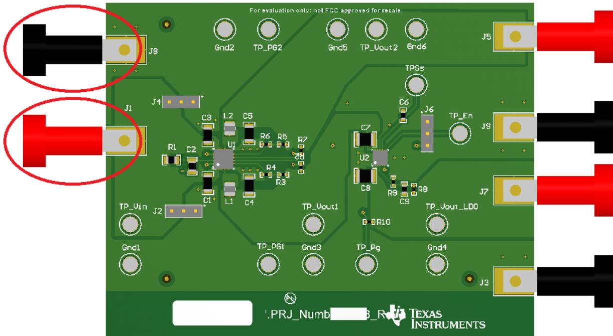
**Figure 3. Reference Design Input-Power-Supply Connectors**
