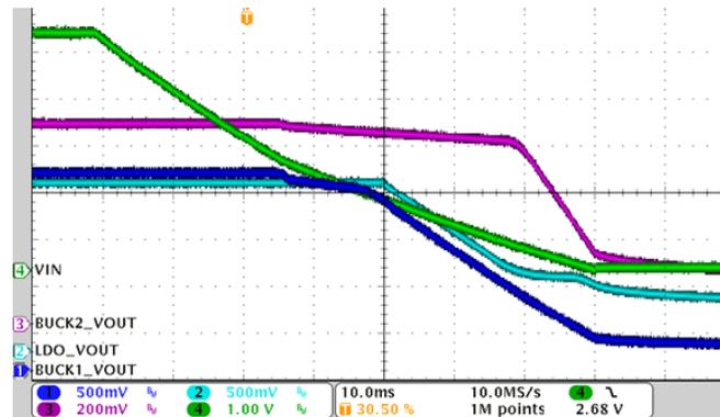
Figure 19. Shutdown Without Load
