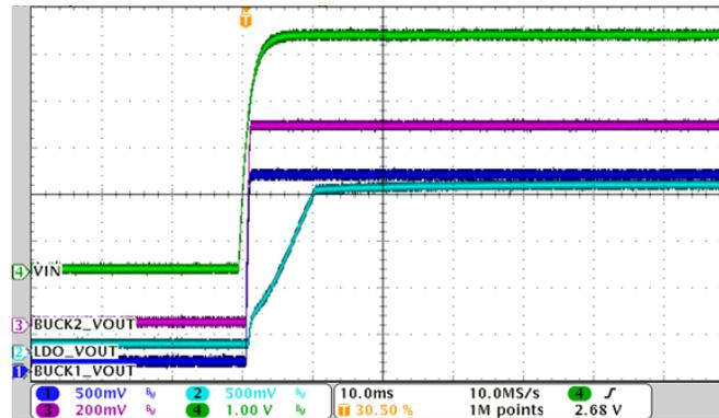
Figure 18. Start-Up Without Load
