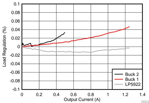
Figure 11. System Output Voltages Load Regulation
