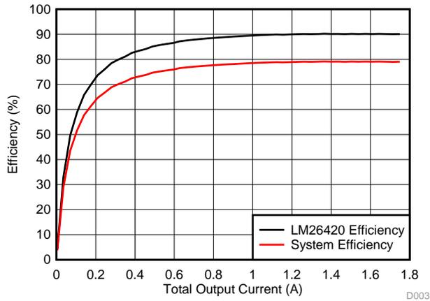
Figure 12. System Efficiency
