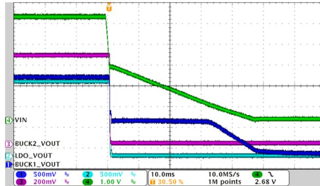
Figure 21. Shutdown With Full Load
