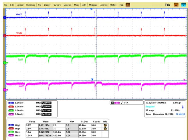
Figure 14. 3.3-V DRV8850 Board—95% Duty Cycle
