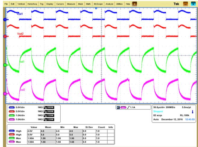
Figure 16. 5-V DRV8850 Board—50% Duty Cycle
