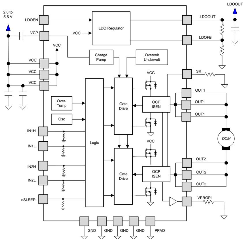
Figure 2. DRV8850 Functional Block Diagram
