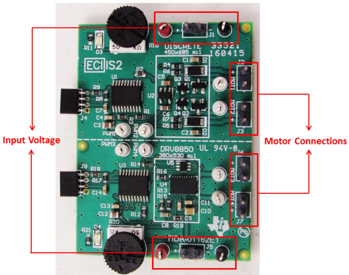
Figure 7. Input and Output Connections
