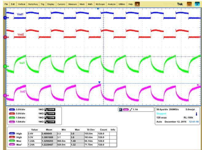
Figure 12. 3.3-V DRV8850 Board—50% Duty Cycle
