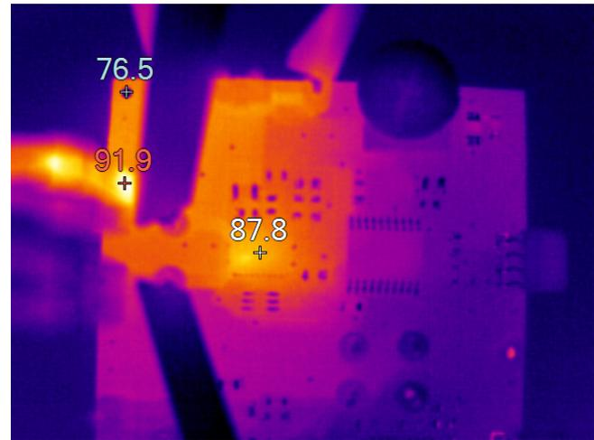
Figure 20. 5-V DRV8850 Board at 95% Duty Cycle
