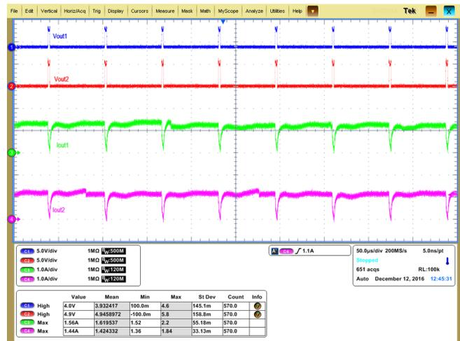
Figure 18. 5-V DRV8850 Board—95% Duty Cycle
