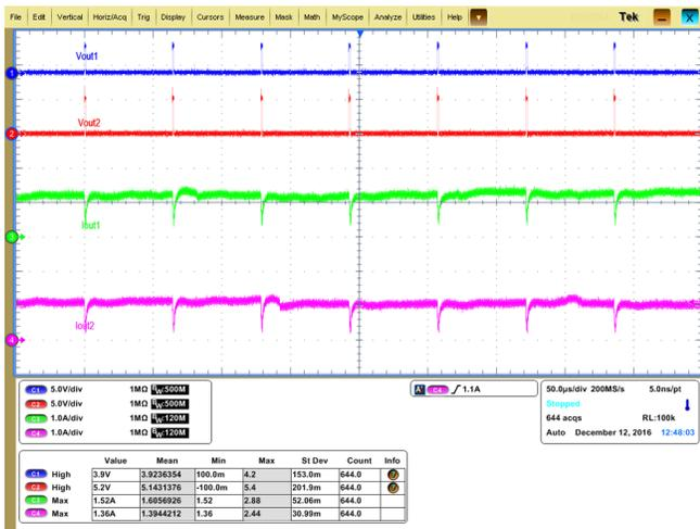
Figure 17. 5-V Discrete Board—95% Duty Cycle
