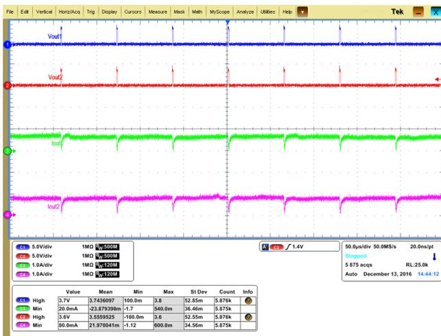
Figure 13. 3.3-V Discrete Board—95% Duty Cycle
