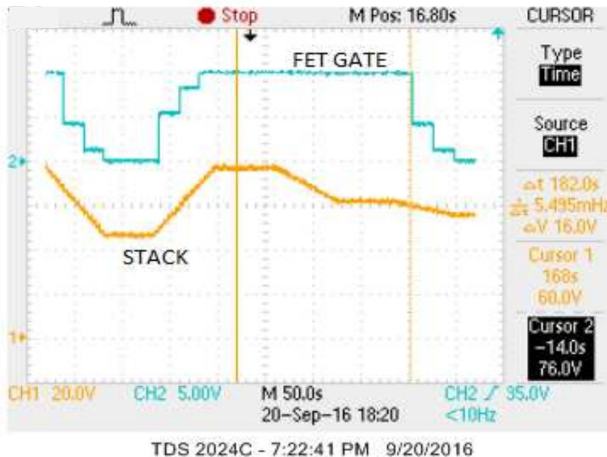
Figure 10. Cumulative Stack Voltage Versus Gate Voltage Enabling Fuse
