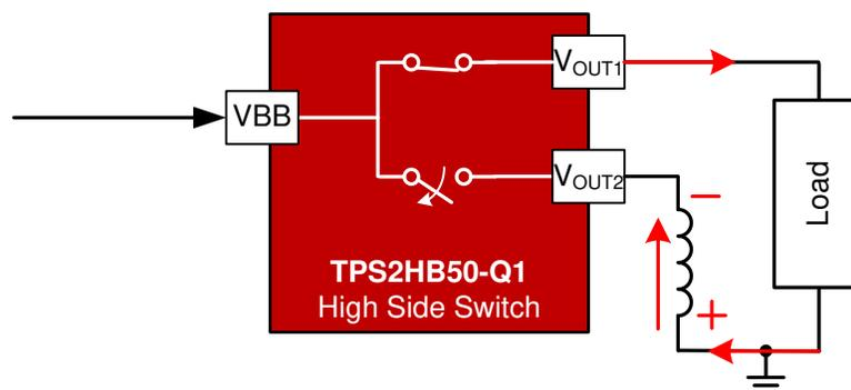
Since this load is pulse-width modulated it is constantly turning on and off quickly which makes the addition of a flyback diode even more necessary.
