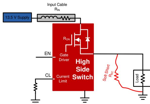
As previously discussed, existing high-side switches have a very high current-limit threshold and will not shut the current off to the load unless it passes that threshold or hits thermal shutdown. Therefore, if the short-circuit resistance is 1.5  $\Omega$ , then the current through the output is calculated by [Equation 1](#).
