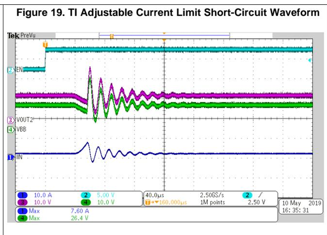
This is unacceptable for most applications that a short circuit on one output can cause other outputs to turn off. It is obvious that the cable inductance is causing the VBB of the device to ring which rings the output. However, with setting the current limit low for the specific load, the disturbance on VBB is limited and does not cause the entire part to go into an undervoltage event and shut down.
