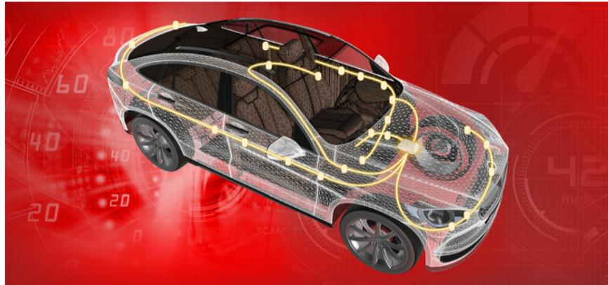
As [Figure 5](#) illustrates, these wires can be up to 3 meters long and have to be routed around large mechanical components of the vehicle. This means that while the resistance is very low the inductance of the wire can be up to 5  $\mu\text{H}$ . This is also true of the output cables that go to the load. However, since they are obviously carrying less current than the input cable, their resistance per unit length will be high because they are smaller gage.
