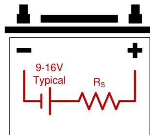
Load dump occurs when the battery is connected in the system to the alternator and then abruptly gets disconnected. This causes the voltage on the power line to increase as high as 120 V and can take up to 400 ms to decay. In most vehicles; however, the load dump pulse is suppressed by large circuitry that can clamp it down to 40 V. For this reason TI makes all of their smart high-side switches tolerant of voltages up to 40 V so that it can survive a load dump condition.
