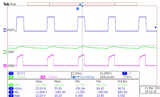
Since the current sense mechanism is measuring the current going through the switch, when pulse-width modulating the enable pin, the current sense output turns off. So taking into consideration that the measured current is only valid when the part is enabled gives an error graph of Figure 21 and an average error of 3.19%. However, looking at the error graph, the error does increase for the light load and, decreases as the current rises.
