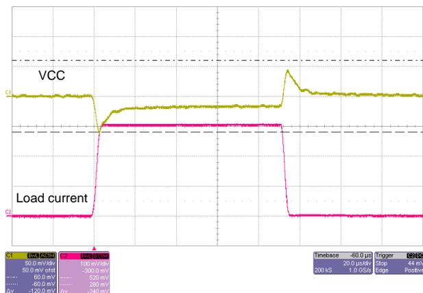
Figure 5. VCC Transient Response (5 V<sub>IN</sub>, 3- to 6-A Load Step, JP2 Shorted, Measured at J33)
