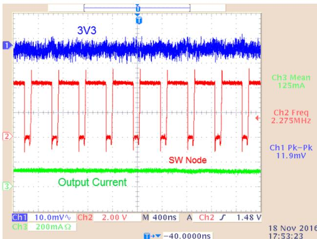
Figure 46. "3V3" Ripple (125-mA Load; 24- $V_{AC}$  Source)
