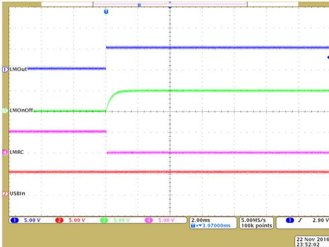
Figure 31. ORing Startup (LMOOut Power Up; USB Source Present)
