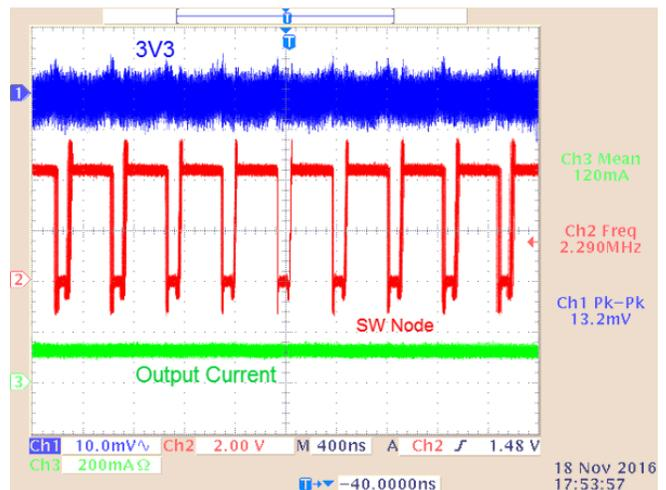
Figure 47. "3V3" Ripple Persist (120-mA Load; 24- $V_{AC}$  Source)
