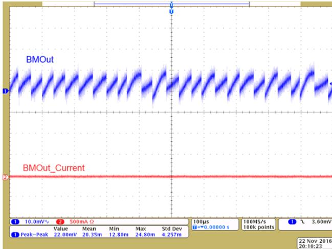
Figure 58. "BMOut" Ripple (1 mA; Battery and USB Sources)
