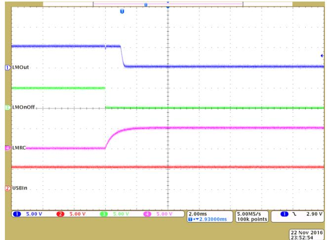
Figure 32. ORing Shutdown (LMOOut Power Loss; USB Source Present)
