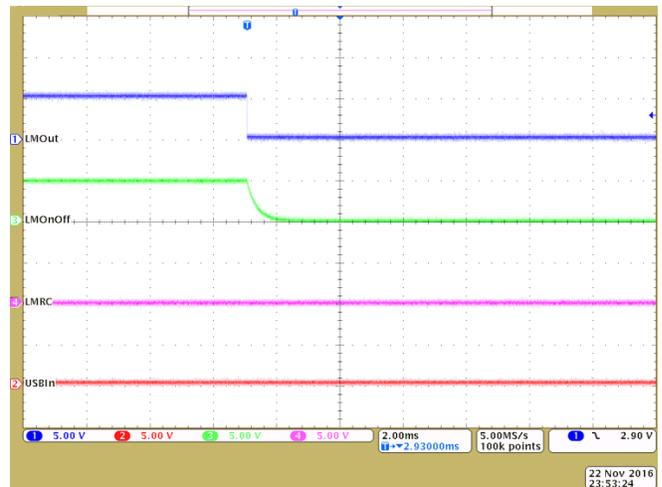
Figure 34. ORing Shutdown (LMOOut Power Loss; USB Source Absent)
