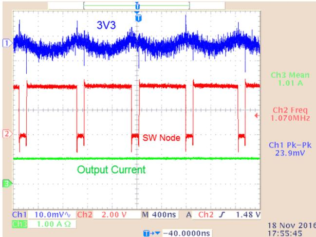
Figure 48. "3V3" Ripple (1-A Load; 24-V<sub>AC</sub> Source Plus Battery)
