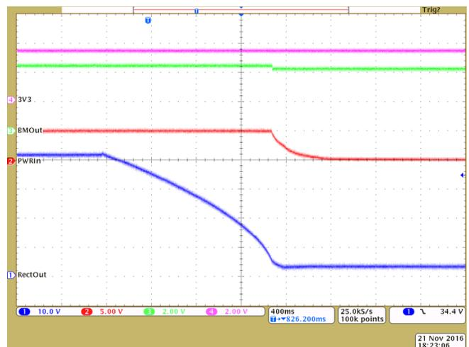
Figure 24. 30-V<sub>AC</sub> Shutdown
