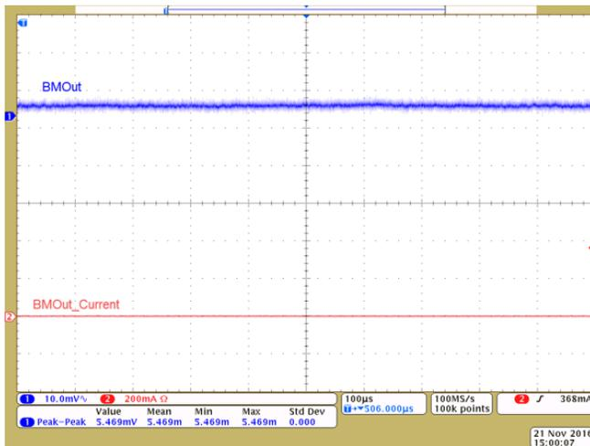
Figure 56. "BMOut" Ripple (0 A; Battery Source Only)
