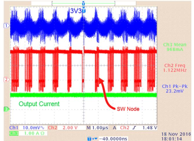
Figure 49. "3V3" Ripple Persist (1-A Load; 24-V<sub>AC</sub> Source Plus Battery)
