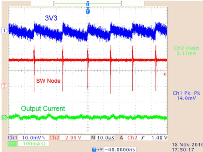
Figure 44. "3V3" Ripple (No Load; 24- $V_{AC}$  Source)
