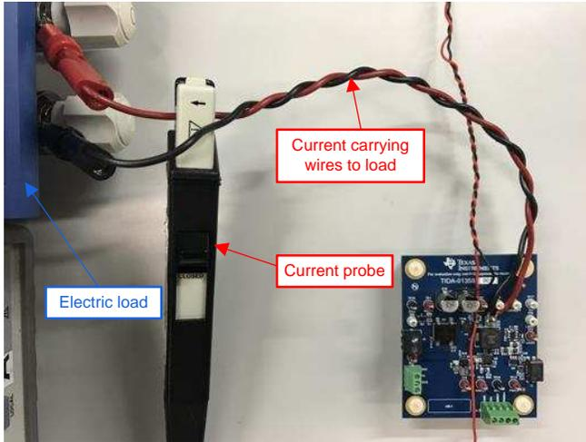
Figure 15. Current Probe and Electronic Load Test Setup
