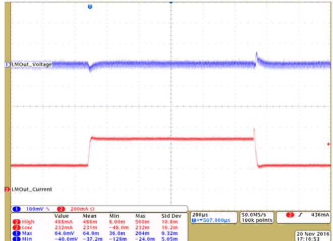
Figure 36. LM5166 Transient Response (200 to 480 mA)
