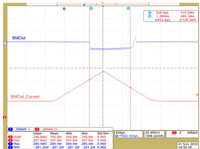
Figure 42. BMOOut Transient Response (250- to 750-mA Slow Ramp; Battery and PWRin Source)
