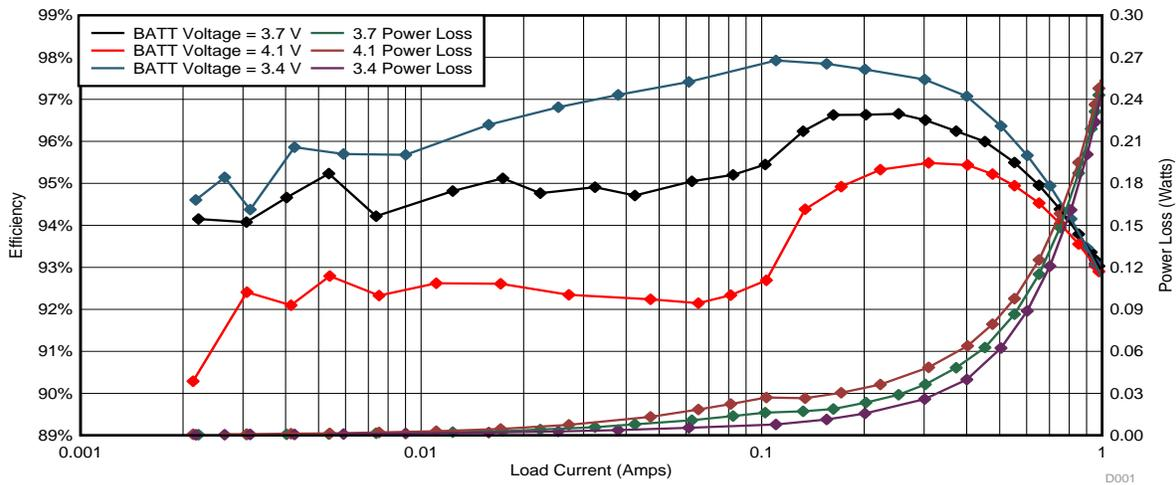
Figure 61. Battery to 3V3 Power Bus Efficiency and Power Loss
