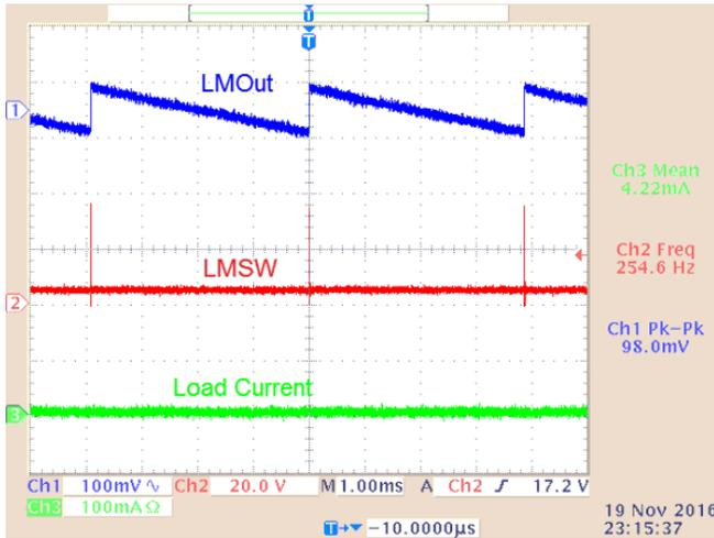
Figure 51. LMOut Ripple (No Load)
