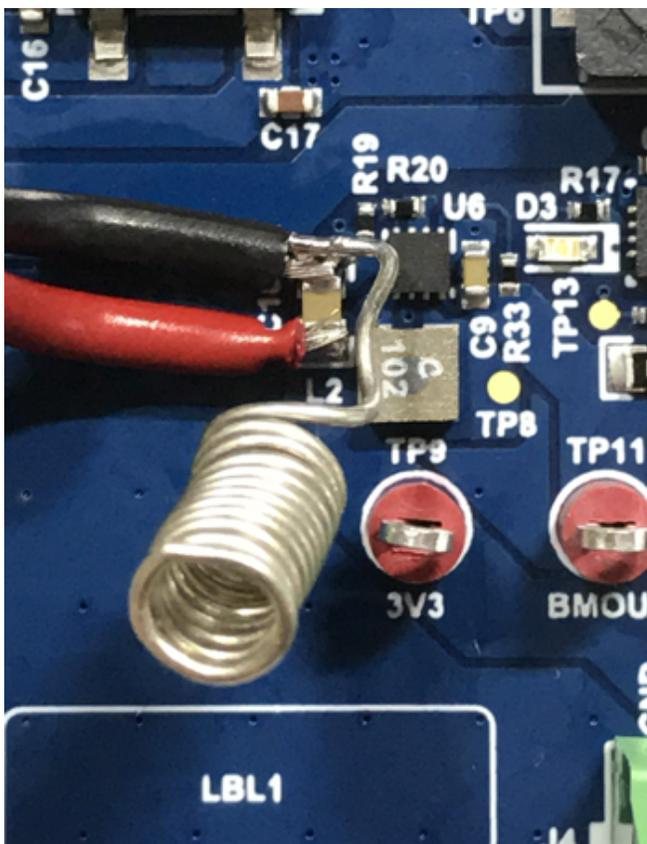
Figure 13. Soldered Output Wires Test Setup
