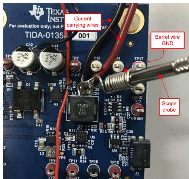
Figure 14. Scope Probe and Barrel Test Setup
