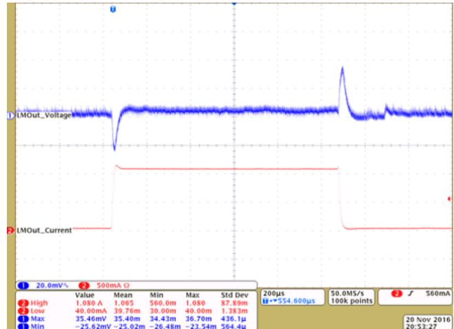
Figure 39. TLV62080 Transient Response (0 to 1 A)
