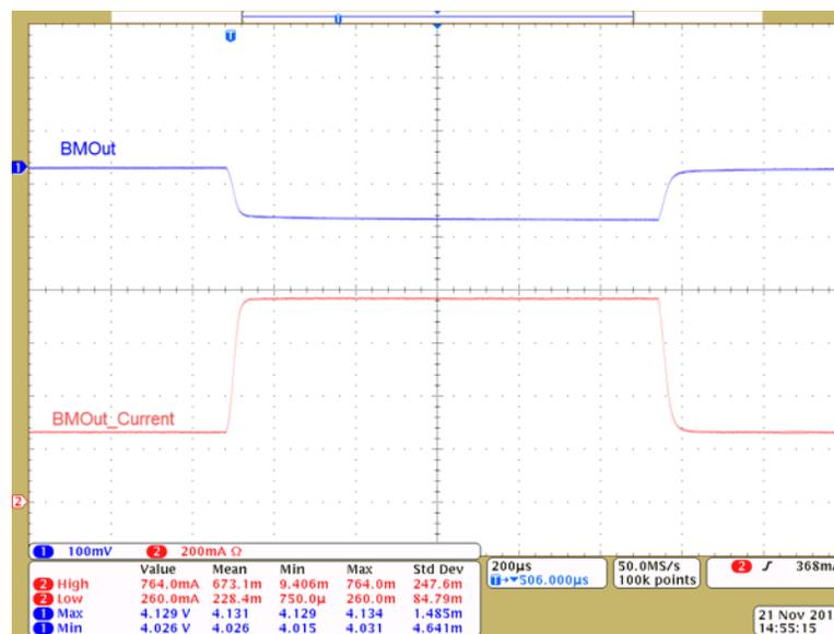
Figure 43. BM24072 Transient Response (250 to 750 mA; Battery Only)
