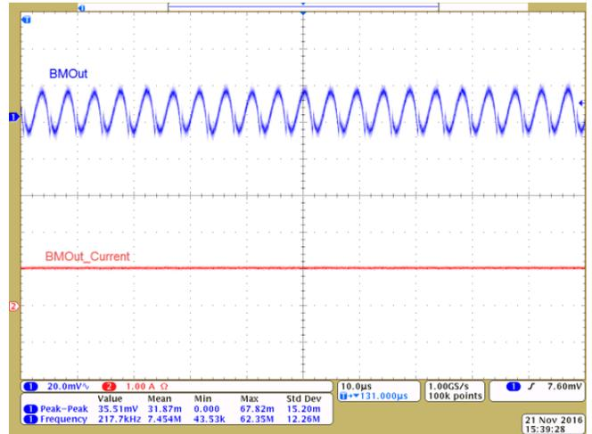
Figure 59. "BMOut" Ripple (1 A; Battery and USB Sources)
