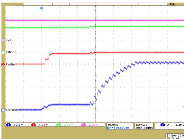
Figure 23. 30-V<sub>AC</sub> Startup
