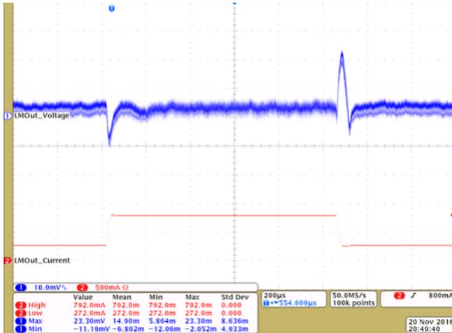
Figure 38. TLV61080 Transient Response (250 to 750 mA)
