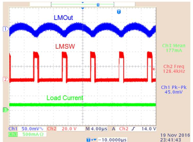
Figure 54. LMOut Ripple Persist (180-mA Load)
