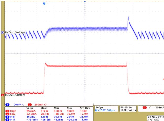
Figure 35. LM5166 Transient Response (0 to 480 mA)
