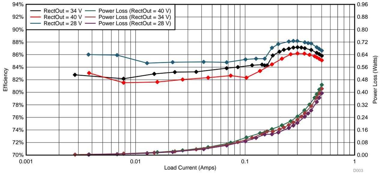
Figure 63. LM5166 Efficiency and Power Loss
