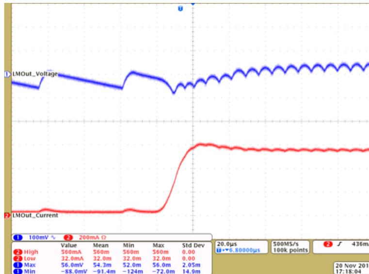
Figure 37. LM5166 Transient Response Slew
