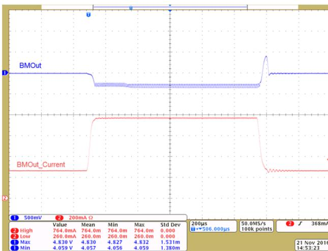
Figure 41. BM24072 Transient Response (250- to 750-mA; Battery and PWRin Source)
