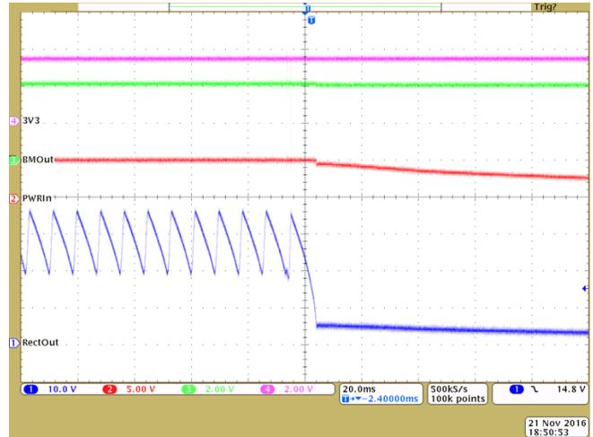
Figure 20. 24-V<sub>AC</sub> Shutdown (3V3 Load = 750 mA)
