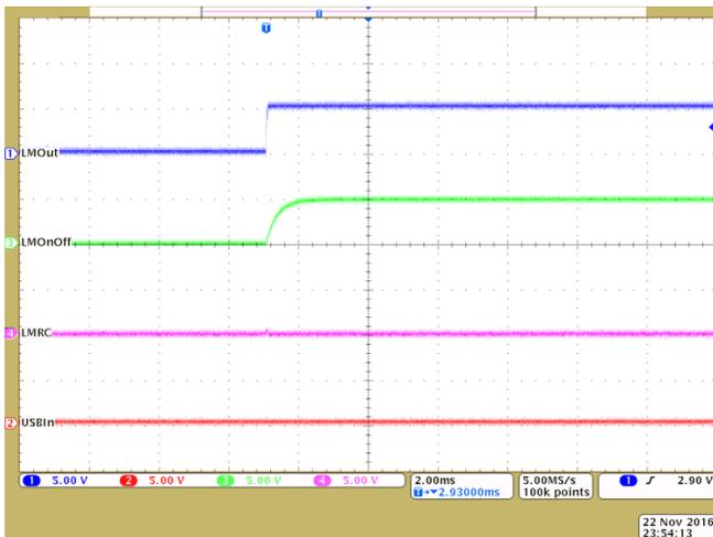
Figure 33. ORing Startup (LMOOut Power Up; USB Source Absent)
