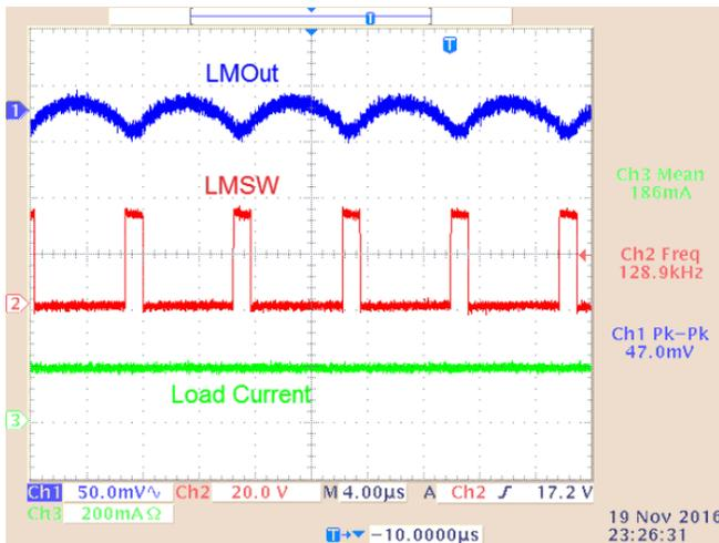
Figure 53. LMOut Ripple (180-mA Load)
