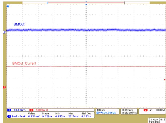
Figure 57. "BMOut" Ripple (1 A; Battery Source Only)
