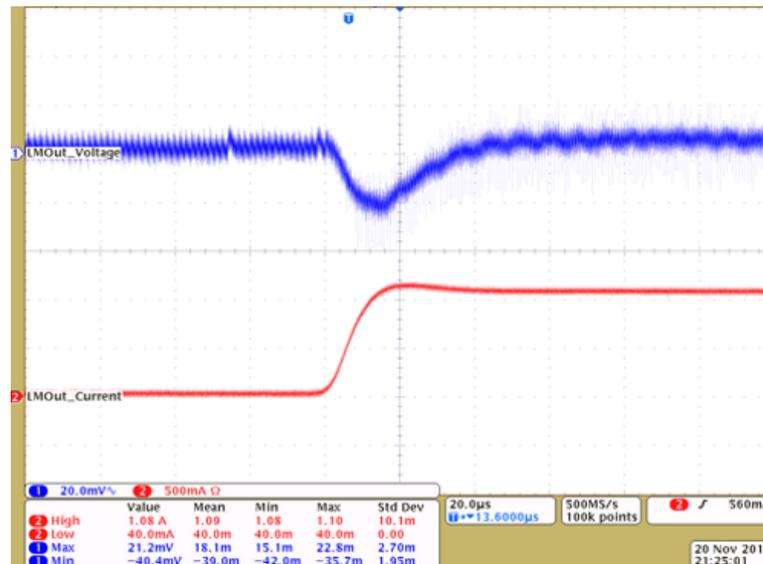
Figure 40. TLV62080 Transient Response Slew
