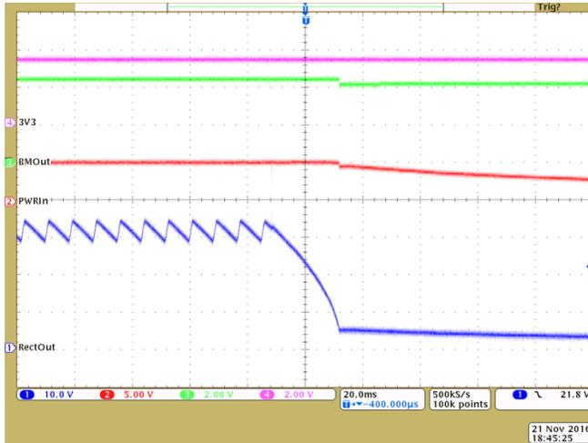
Figure 19. 24-V<sub>AC</sub> Shutdown (3V3 Load = 200 mA)
