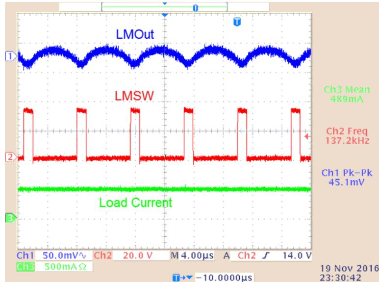
Figure 55. LMOut Ripple (490-mA Load)
