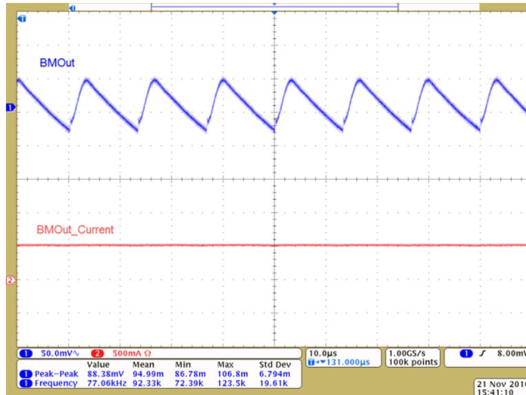
Figure 60. "BMOut" Ripple (500 mA; Battery and USB Sources)
