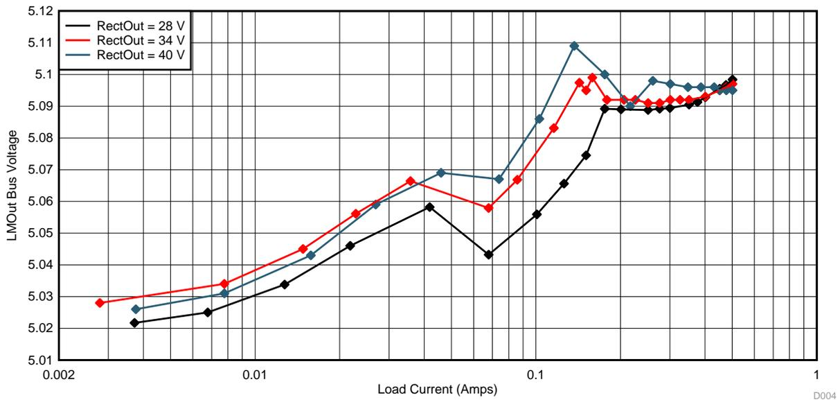
Figure 64. LM5166 Load Regulation
