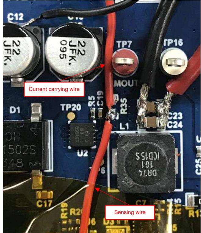
Figure 16. Separate Sensing and Current Carrying Wires Test Setup
