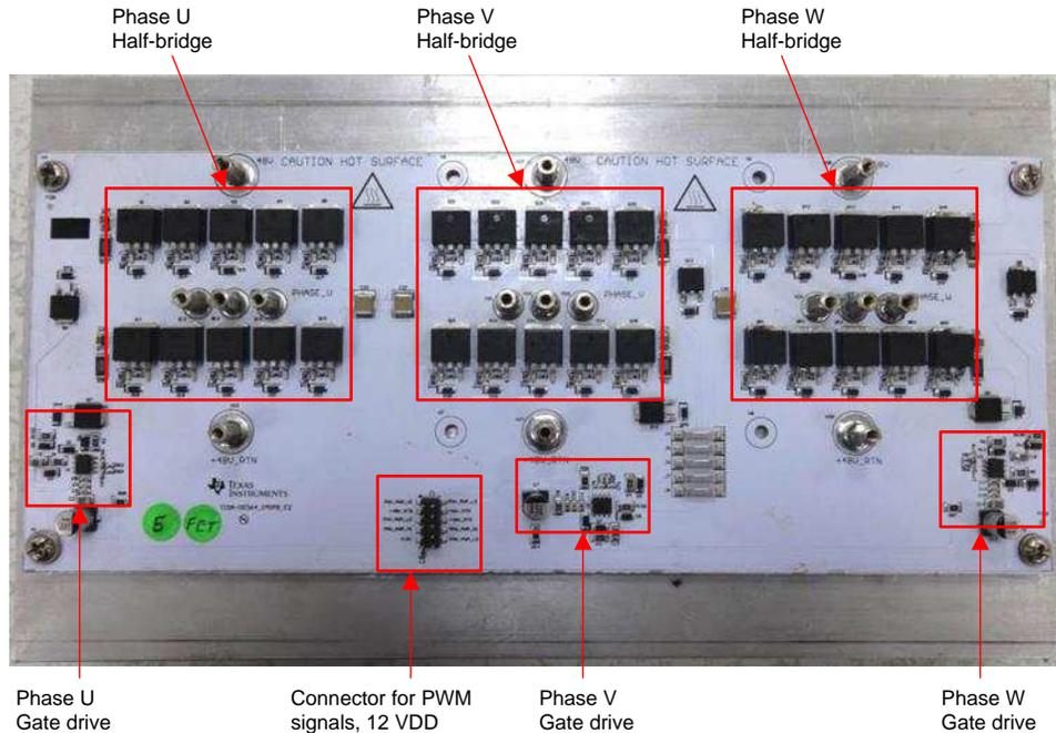
**Figure 20. Inverter Board Description**
