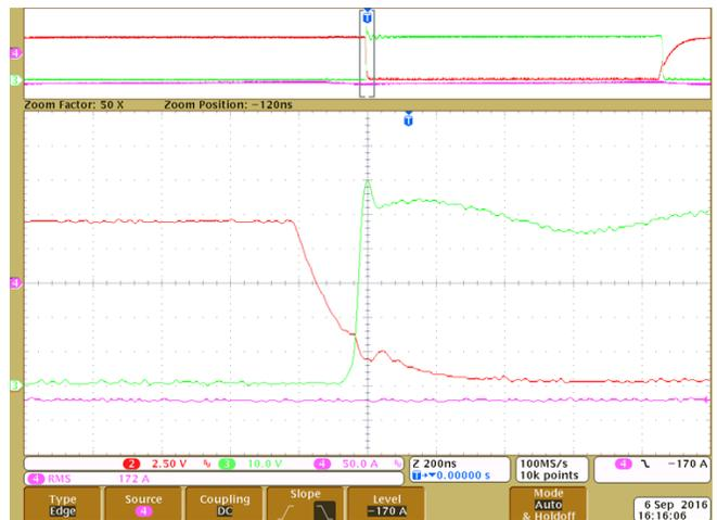
Figure 40. Bottom FET Hard Switch OFF
