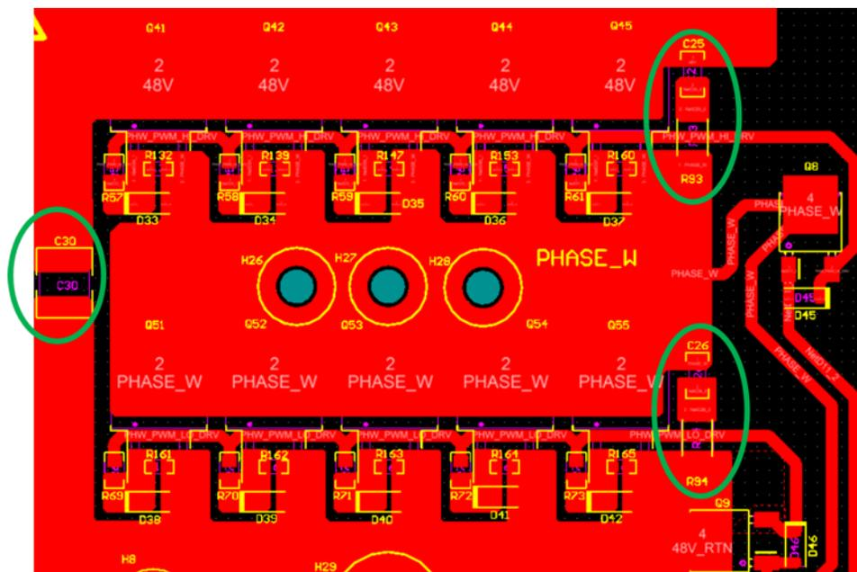
**Figure 52. Location of Decoupling Capacitor and Snubber Circuit**
