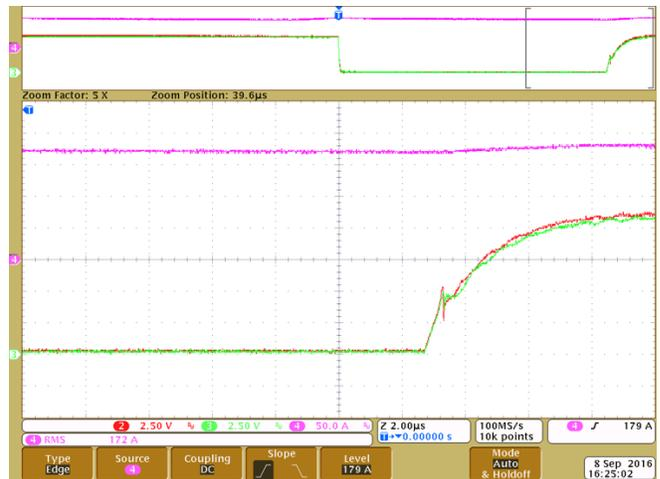
Figure 44. Top FET Hard Switch ON
