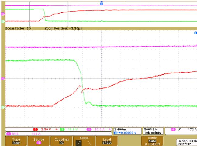
Figure 29. Top FET Hard Switch ON
