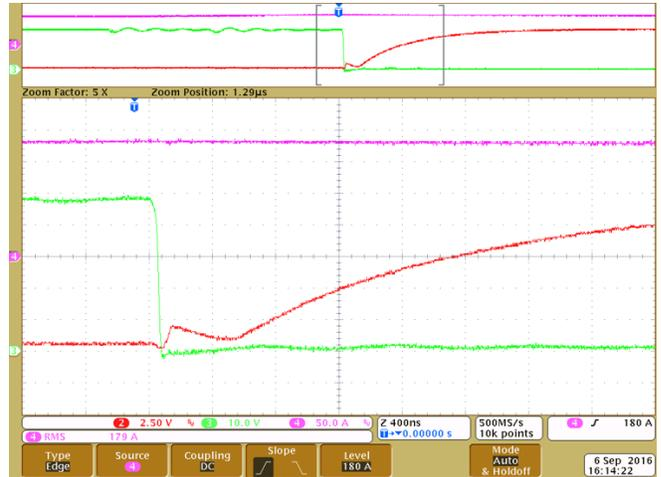
Figure 36. Bottom FET Soft Switch ON
