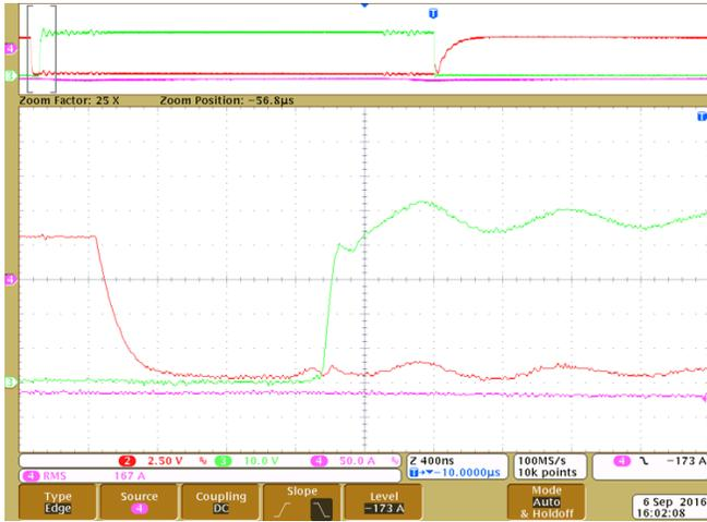
Figure 41. Top FET Soft Switch OFF
