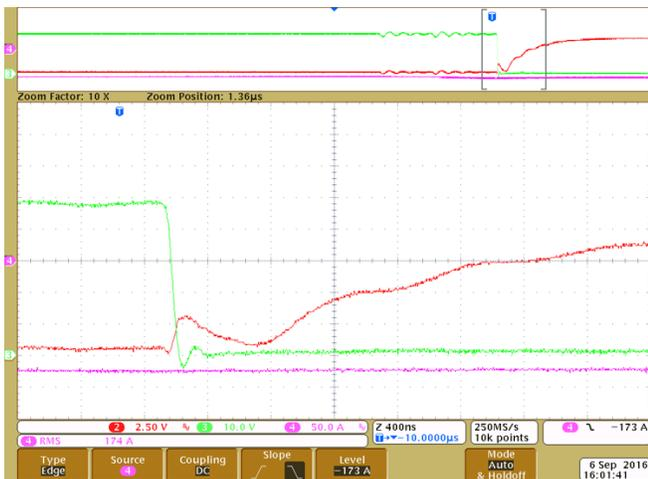
Figure 39. Top FET Soft Switch ON
