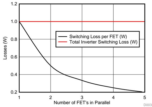
Figure 10. Normalized Switching Loss versus Parallel FETs
