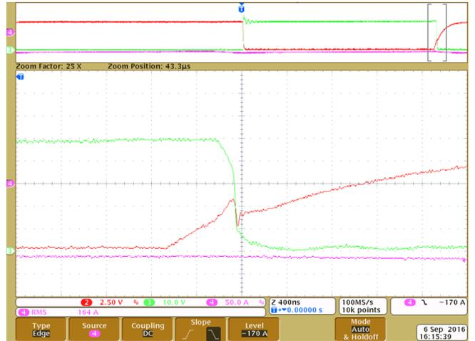
Figure 42. Bottom FET Hard Switch ON
