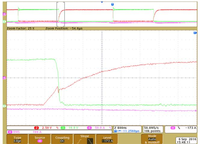
Figure 34. Bottom FET Hard Switch ON
