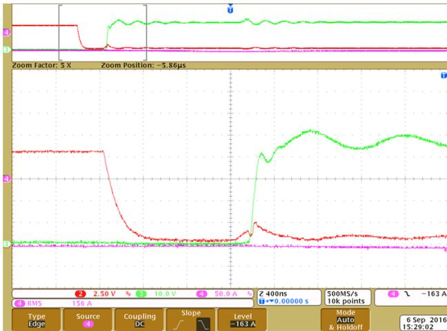
Figure 33. Top FET Soft Switch OFF
