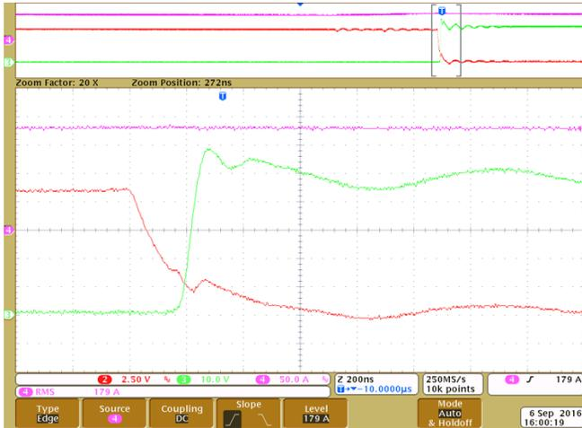
Figure 35. Top FET Hard Switch OFF
