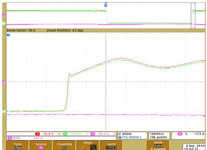
Figure 50. Top FET Soft Switch ON
