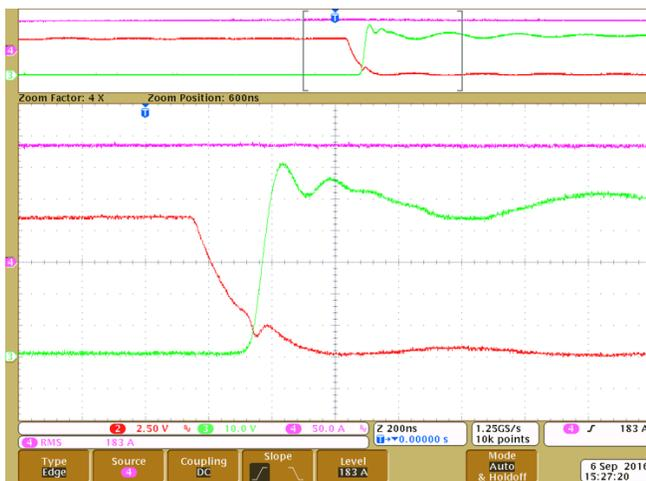
Figure 27. Top FET Hard Switch OFF
