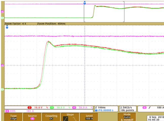
Figure 47. Top FET Hard Switch OFF
