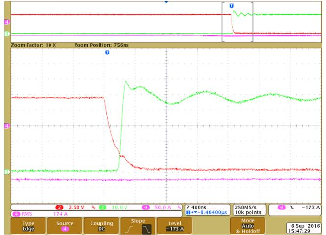
Figure 32. Bottom FET Hard Switch OFF
