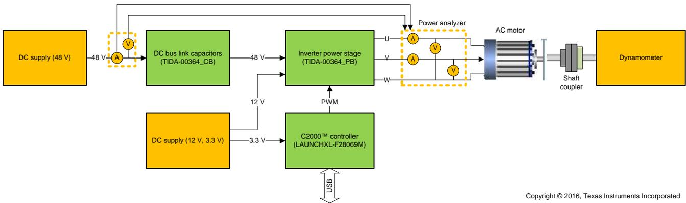
Figure 23. Test Setup Block Diagram
