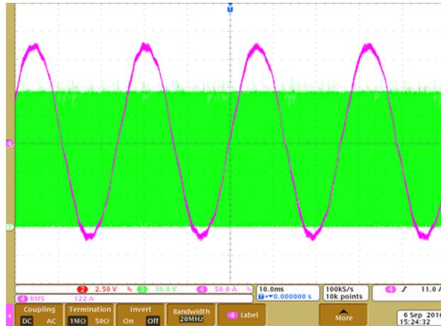
Figure 26. Motor Phase Current Waveform
