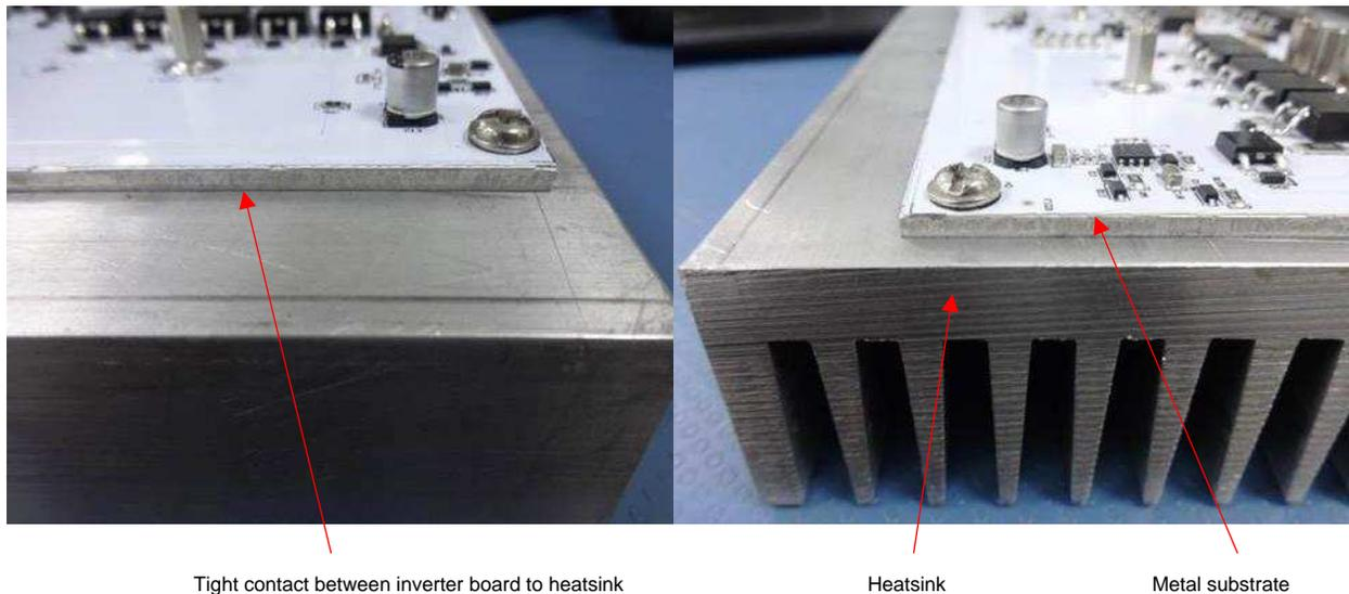
**Figure 21. Tight Connection to Heatsink**
