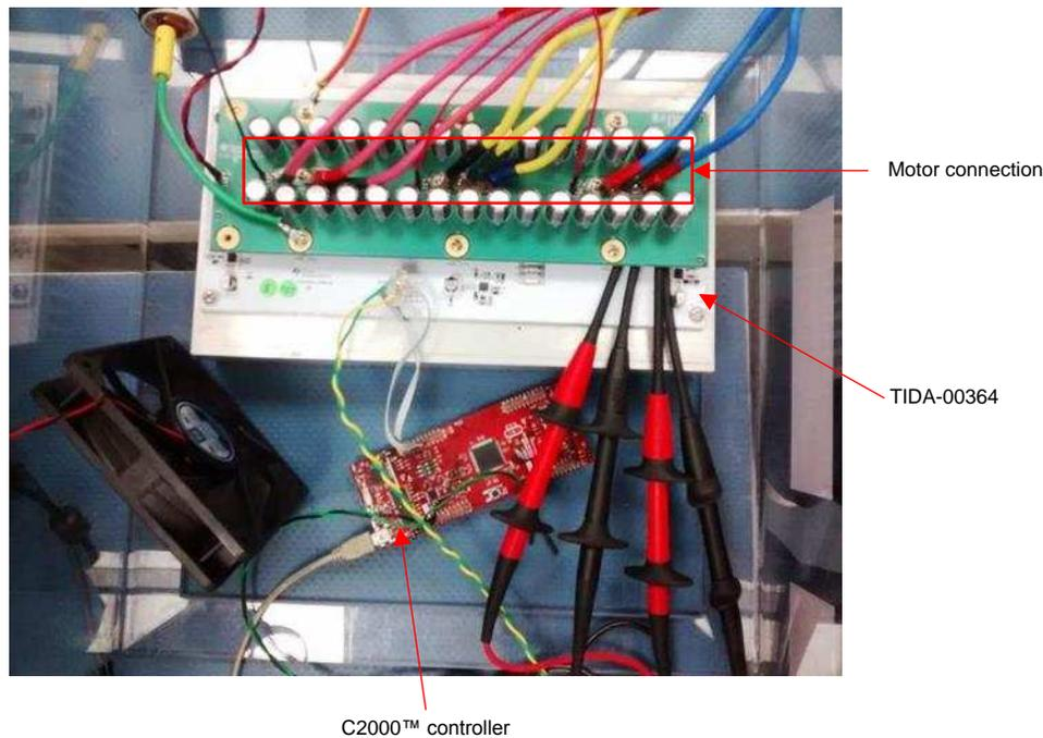
**Figure 25. Test Setup Showing Controller Interface**
