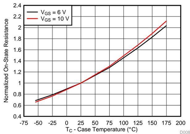
Figure 13.  $R_{DS(on)}$  Variation With Temperature
