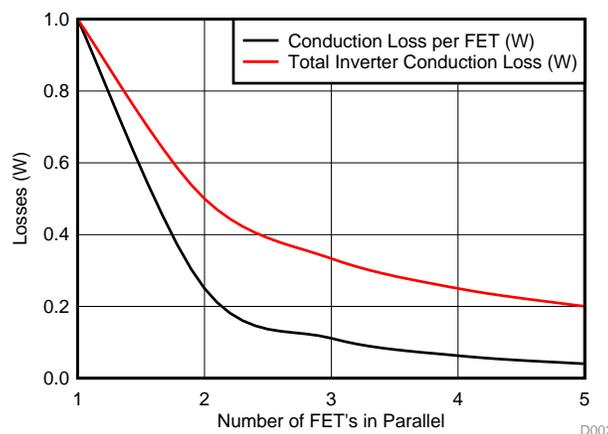
**Figure 9. Normalized Conduction Loss versus Parallel FET's**
