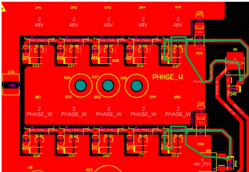
Figure 53. MOSFET Gate Turnoff Loop
