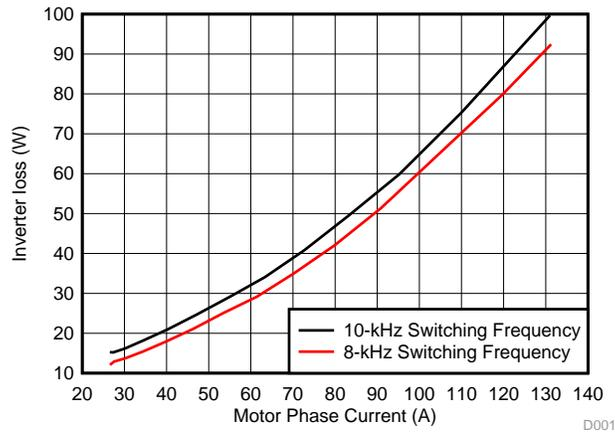
**Figure 51. Inverter Loss versus Motor Phase Current**
