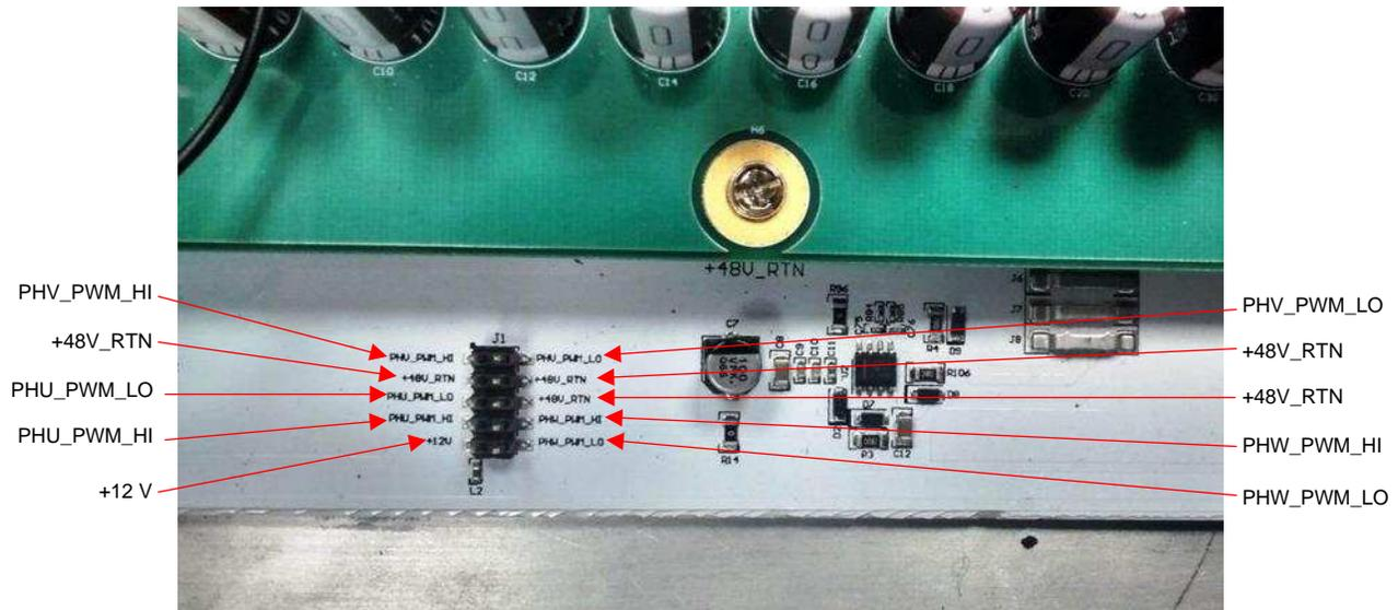
**Figure 22. Controller Interface Connector Description**
