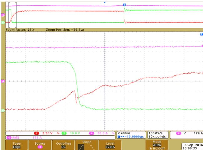
Figure 37. Top FET Hard Switch ON
