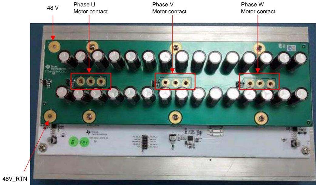
**Figure 19. Power Connections**
