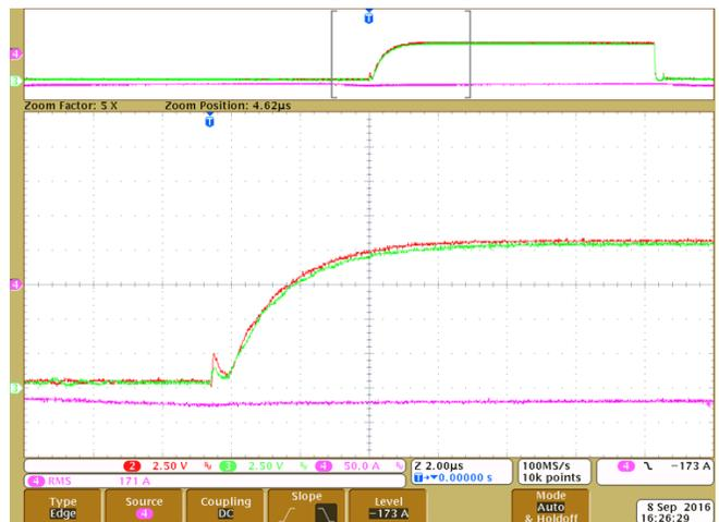
Figure 46. Top FET Soft Switch ON
