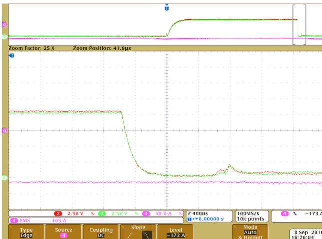
Figure 45. Top FET Soft Switch OFF
