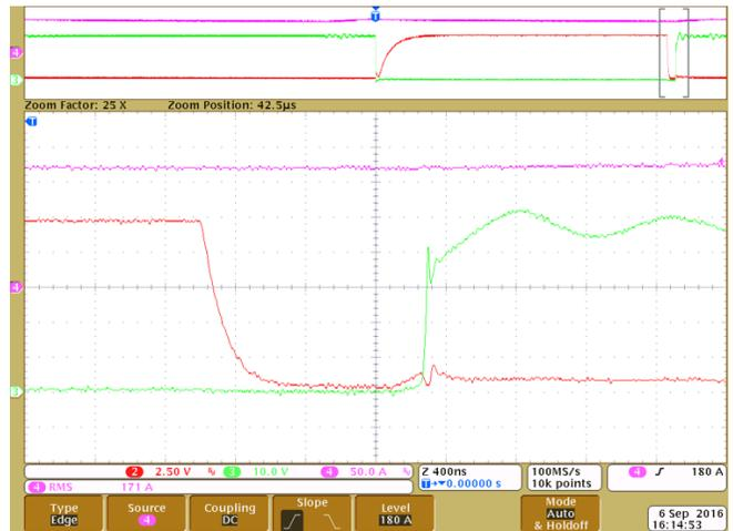
Figure 38. Bottom FET Soft Switch OFF
