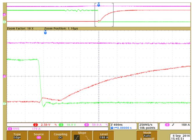
Figure 28. Bottom FET Soft Switch ON
