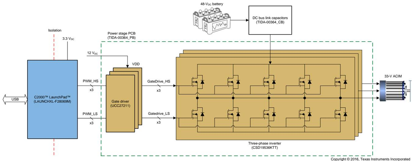
**Figure 2. Block Diagram**
