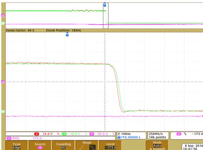
Figure 49. Top FET Soft Switch OFF
