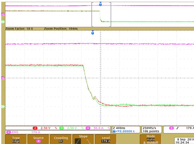
Figure 43. Top FET Hard Switch OFF
