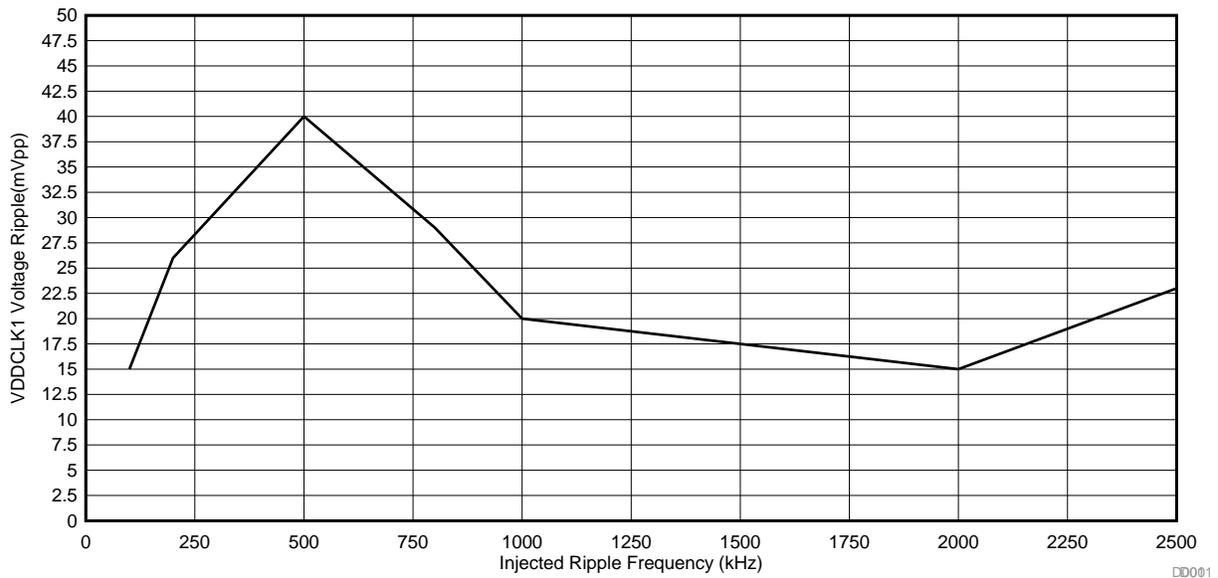
Figure 6. Spur Suppression at VDDCLK1 versus Injected Ripple Frequency
