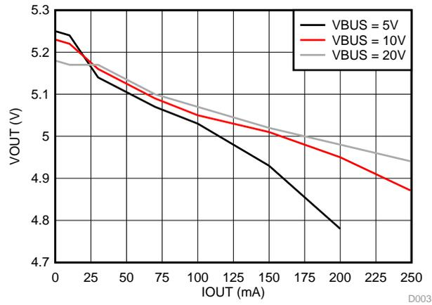
**Figure 2. Load Regulation of Primary-Side Regulation Solution ( $V_{OUT} = 5\text{ V}$ )**
