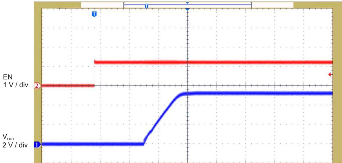
**Figure 4. Start Up By EN Pin ( $V_{BUS} = 10\text{ V}$ ,  $I_{OUT} = 10\text{ mA}$ )**
