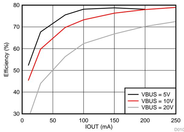
Figure 9. Efficiency of Secondary-Side Regulation Solution
