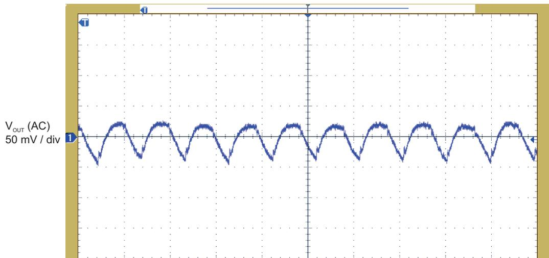
Figure 11.  $V_{OUT}$  Ripple of Secondary-Side Regulation Solution
