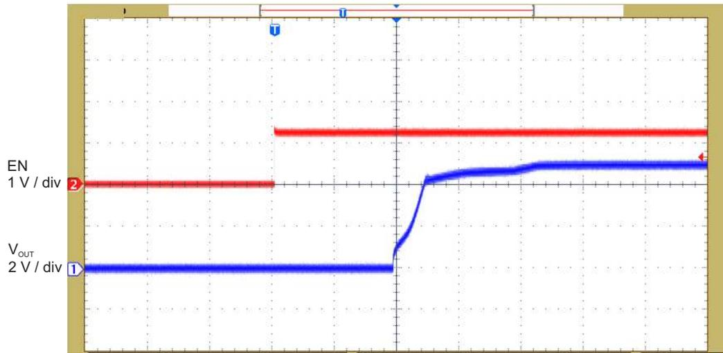
Figure 10. Start-Up Waveform of Secondary-Side Regulation Solution
