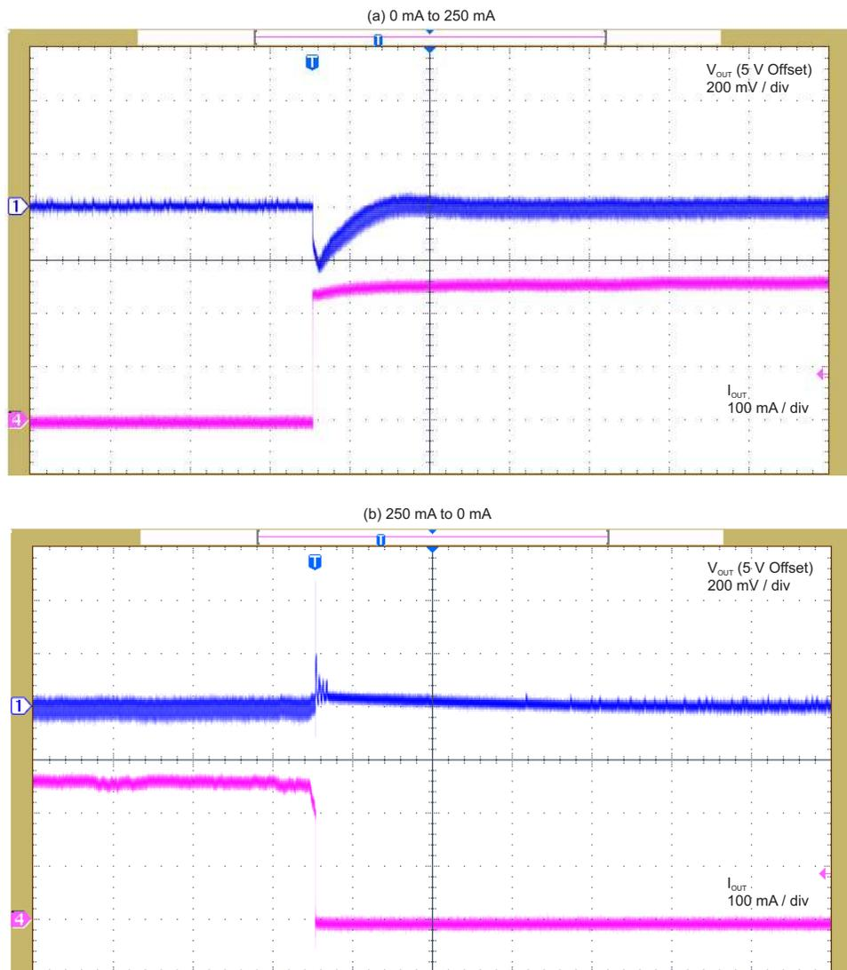
Figure 12. Load Transient of Secondary-Side Regulation Solution
