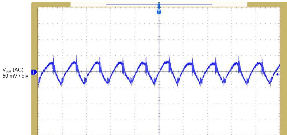
**Figure 5.  $V_{OUT}$  Ripple at  $V_{IN} = 10\text{ V}$  and  $I_{OUT} = 250\text{ mA}$**
