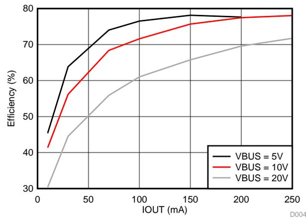
**Figure 3. Efficiency of Primary-Side Regulation Solution**
