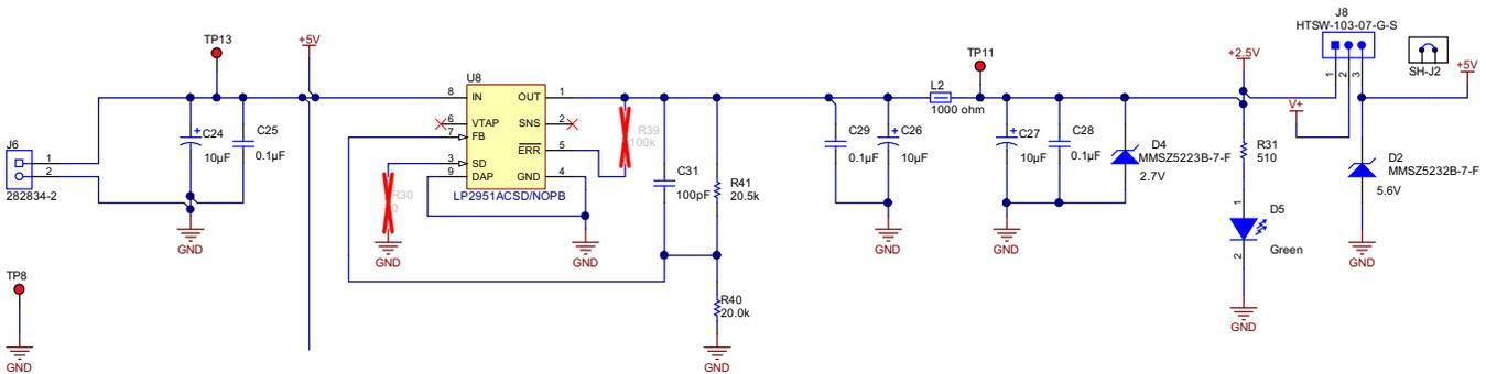
Figure 14. Circuit Diagram for 2.5-V Supply
