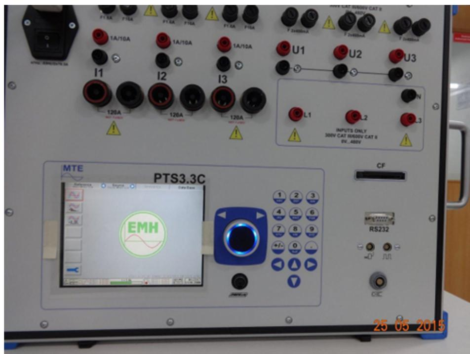
Figure 23. Test System (Including Programmable Power Source)
