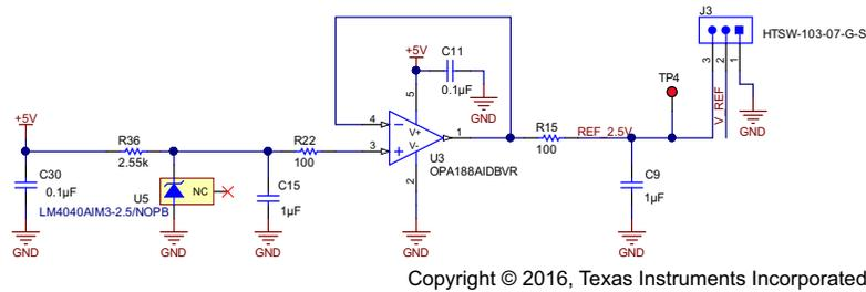
Figure 13. Circuit Diagram for 2.5-V Voltage Reference
