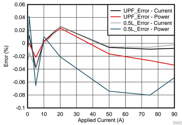
**Figure 26. Fast Settling Current and Power Accuracy for 50 Hz**
