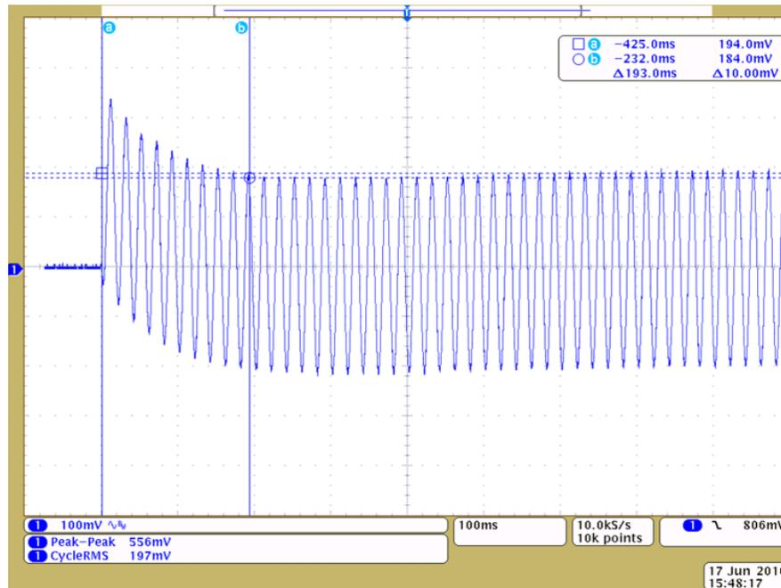
Figure 28. Integrator Output Waveform for Precision Measurement
