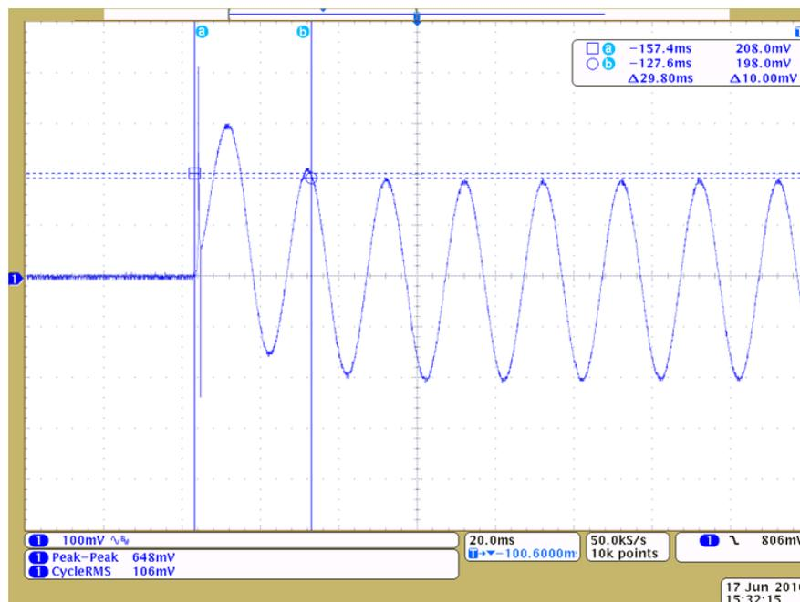
Figure 29. Integrator Output Waveform for Fast Settling
