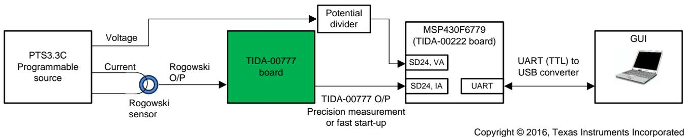
**Figure 22. Test Setup to Connect TIDA-00777 and TIDA-00222**
