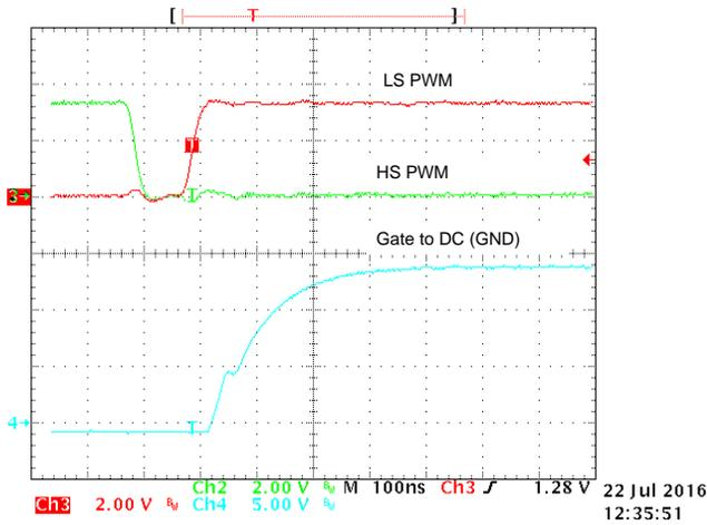
Figure 21. SM72295 Low-Side Gate Driver Output Voltage During Turnon
