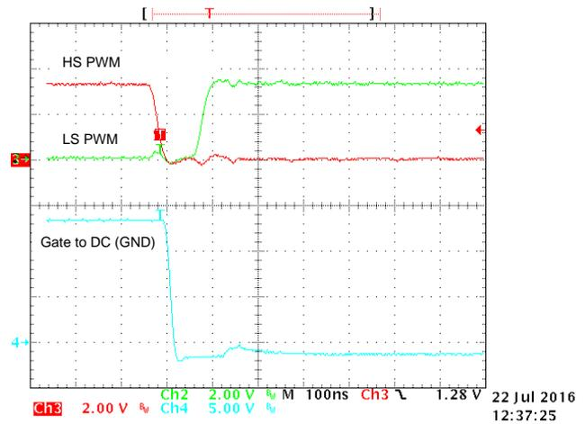
Figure 22. SM72295 Low-Side Gate Driver Output Voltage During Turnoff
