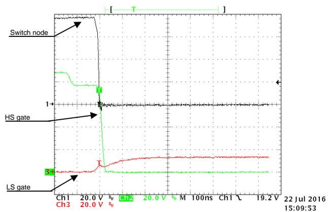
Figure 32. Phase A Falling Switch Node Voltage, High-Side, and Low-Side Gate to GND at -10-A Output Current
