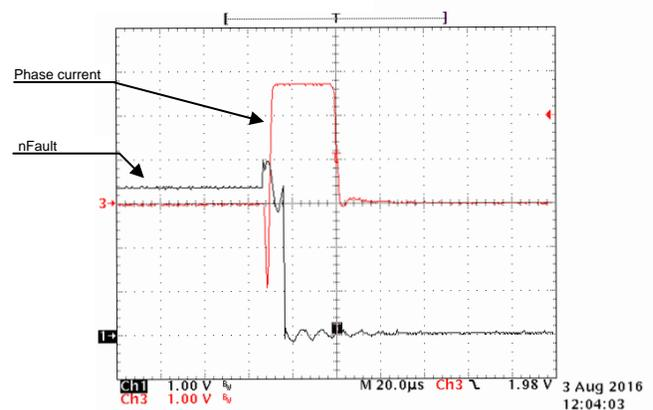
**Figure 53. Short-Circuit Current Between Motor Terminal Phase B to GND and SM72295 nFAULT Signal**
