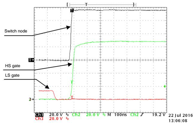
Figure 26. Phase A Rising Switch Node Voltage, High-Side, and Low-Side Gate to GND at 1-A Output Current
