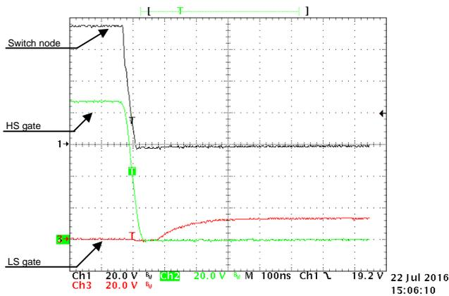
Figure 29. Phase A Falling Switch Node Voltage, High-Side, and Low-Side Gate to GND at 10-A Output Current
