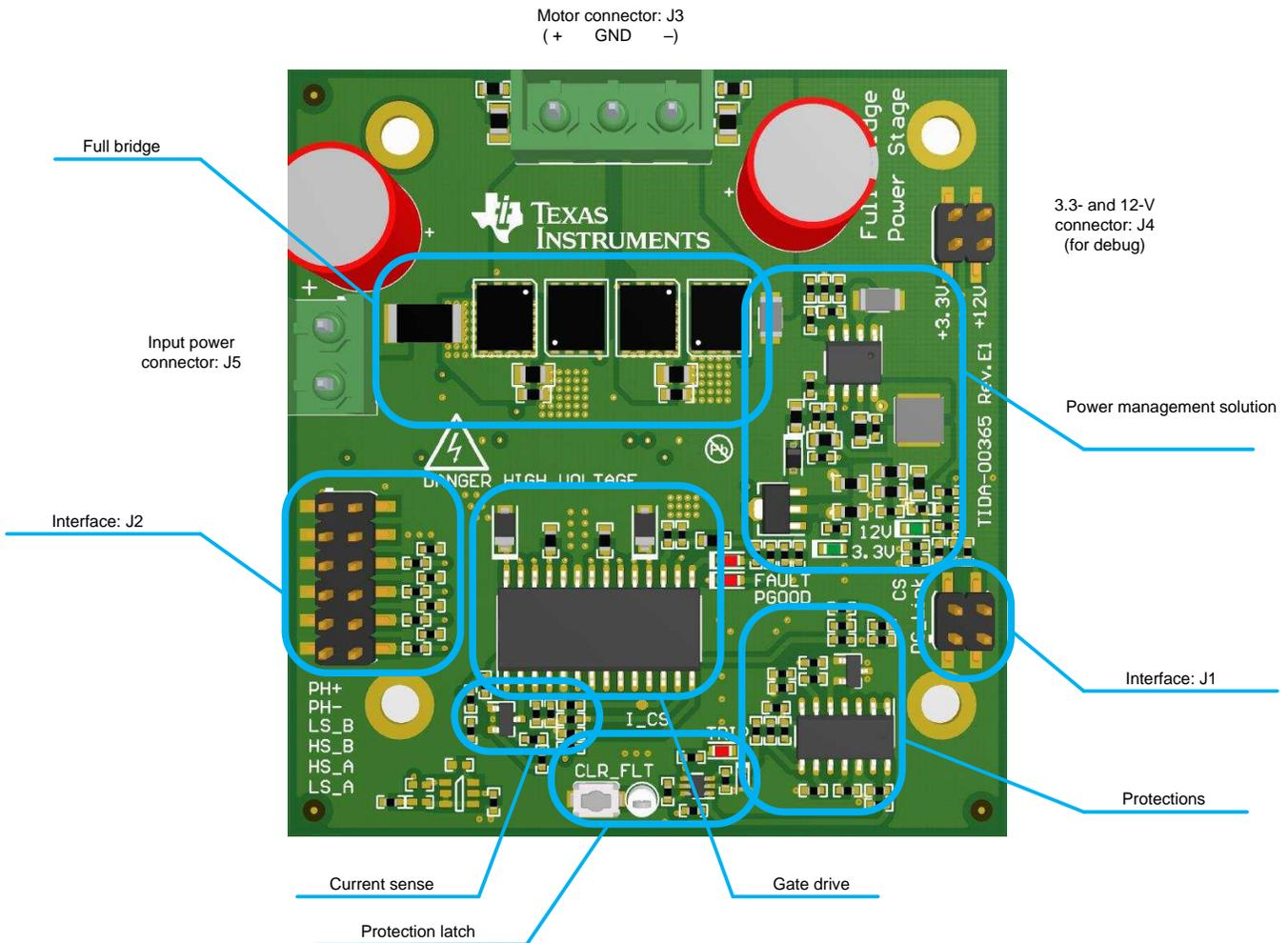
**Figure 15. TIDA-00365 Functional Blocks (Top View)**
