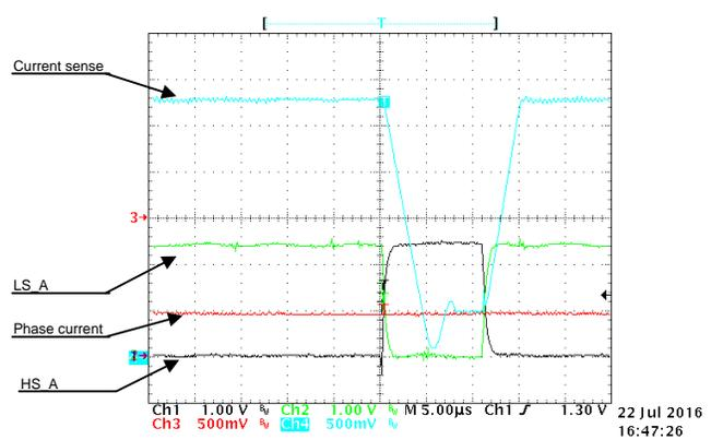
Figure 41. Host Interface Analog Signals, Current Sense Amplifier at J2-2 With  $I_{ref}$  -10 A at 25-kHz PWM, Phase A and Phase B J2
