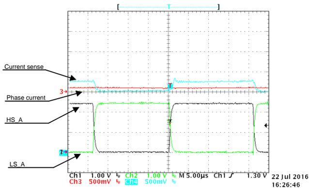
Figure 38. Host Interface Analog Signals, Current Sense Amplifier at J2-2 With  $I_{ref}$  1 A at 25-kHz PWM, Phase A and Phase B J2-2
