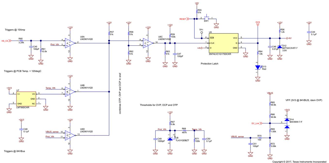
**Figure 13. OVP, OCP, and OTP With Latch, Adjacent Thresholds, and Voltage Feed Forward (VFF) Network**
