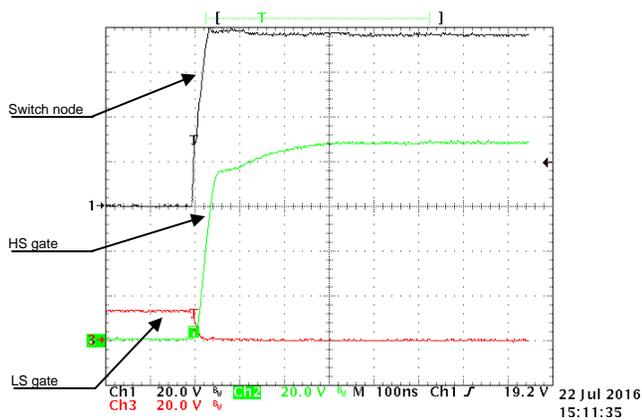
Figure 31. Phase A Rising Switch Node Voltage, High-Side, and Low-Side Gate to GND at -10-A Output Current
