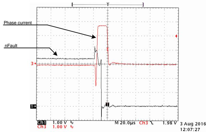
**Figure 51. Short-Circuit Current Between Motor Terminals Phase A to Phase B and SM72295 nFAULT Signal**
