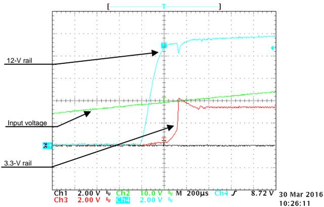
Figure 19. Point-of-Load Power-Up at 50-V DC Input
