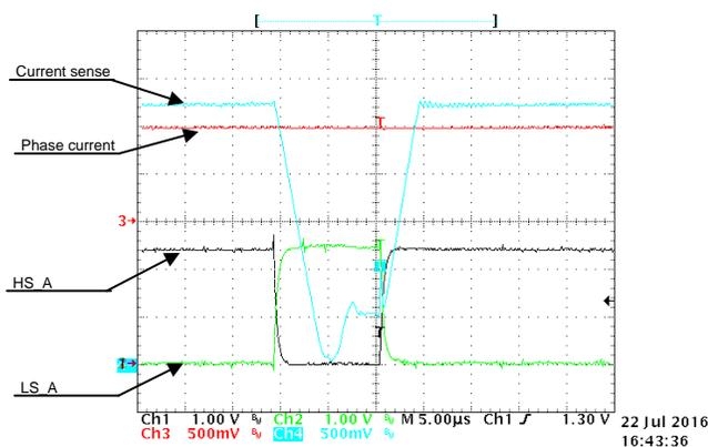
Figure 40. Host Interface Analog Signals, Current Sense Amplifier at J2-2 With  $I_{ref}$  10 A at 25-kHz PWM, Phase A and Phase B J2
