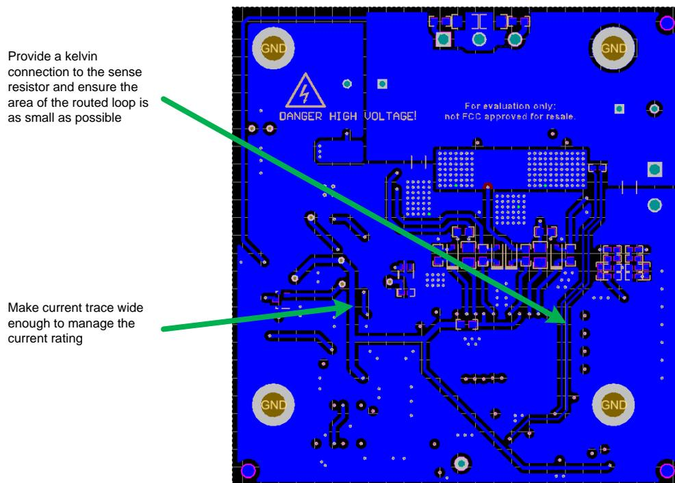
**Figure 57. Bottom Layer (Flip View)**
