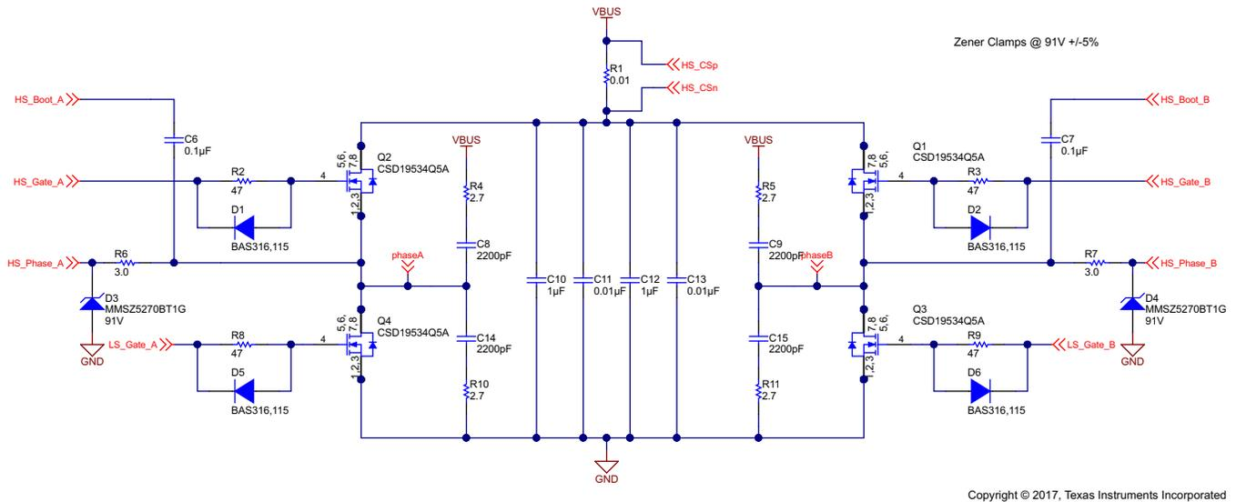
Figure 6. Schematic of Full-Bridge Power Stage
