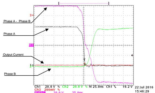
Figure 36. Falling Edge of Output Voltage, Phase A and B Voltage to GND at -10-A Output Current
