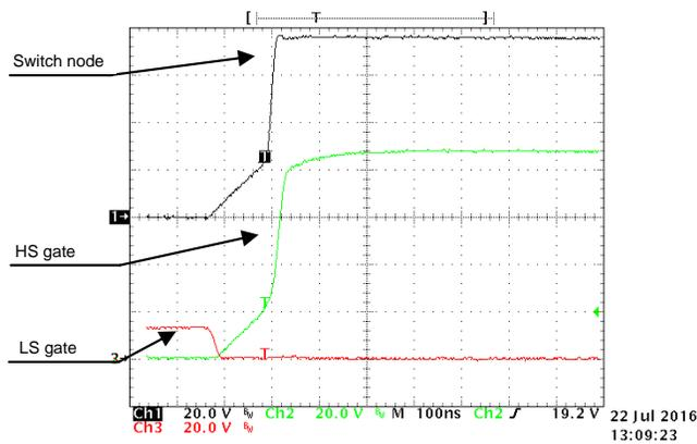
Figure 27. Phase A Rising Switch Node Voltage, High-Side, and Low-Side Gate to GND at -1-A Output Current
