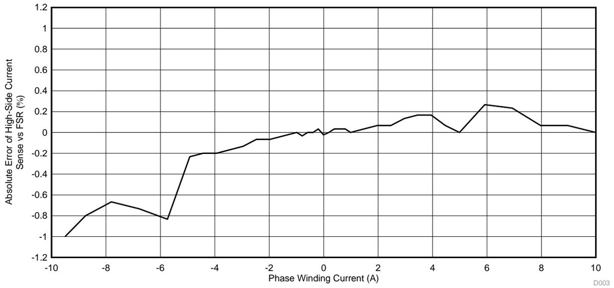
Figure 44. Absolute Error versus Full-Scale Range (–15 to 15 A in %) of SM72295 Current Sense Amplifier Output
