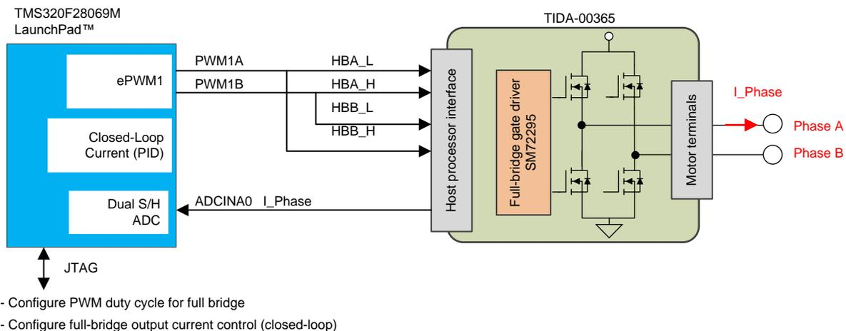
Figure 18. InstaSPIN-MOTION LaunchPad Connection to TIDA-00365 Full-Bridge
