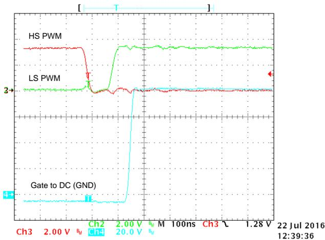
Figure 23. SM72295 High-Side Gate Driver Output Voltage versus GND During Turnon
