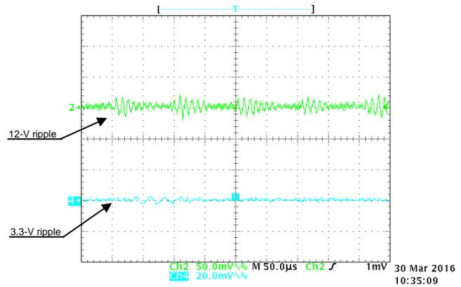
Figure 20. Point-of-Load Voltage Ripple at 3.3-V and 12-V at Nominal Operation
