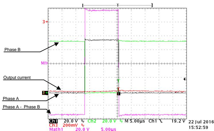
Figure 37. Output Voltage, Phase A and B Voltage to GND at -10-A Output Current Over One PWM Cycle
