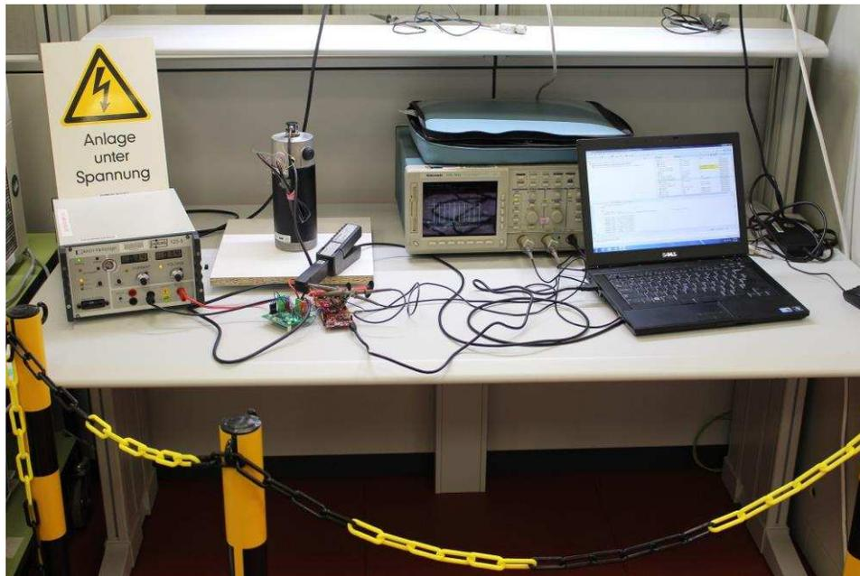
Figure 17. TIDA-00365 Test Setup With Brushed DC Motor
