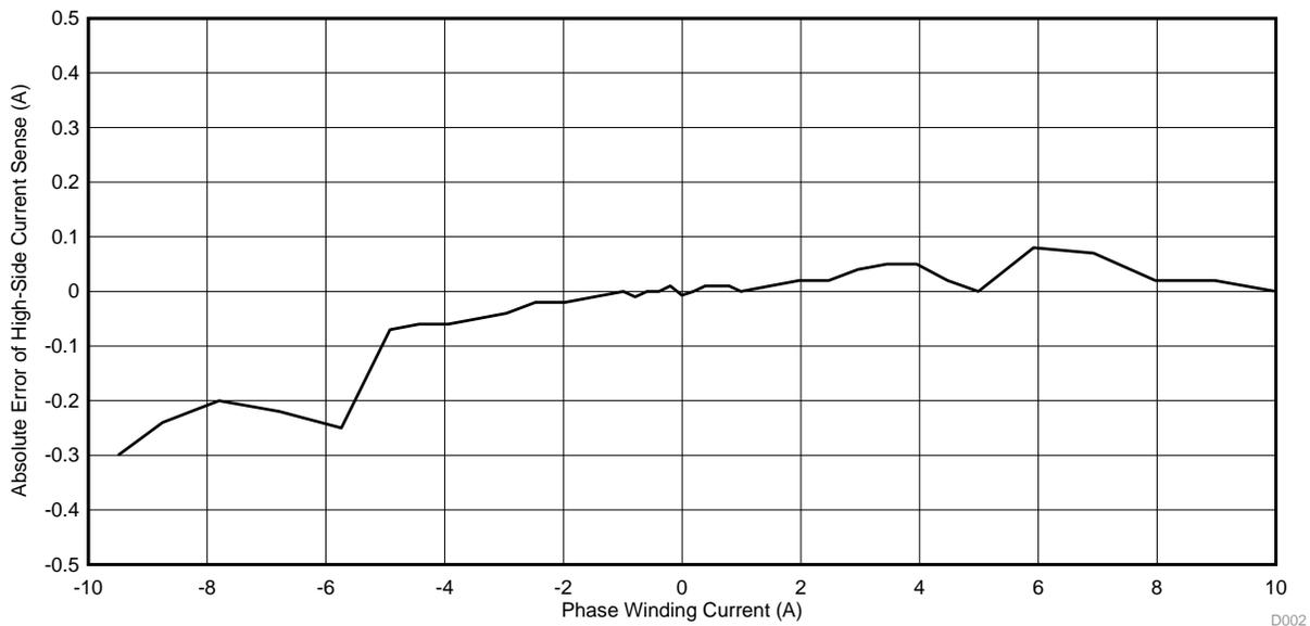
**Figure 43. Absolute Error (in A) of SM72295 Current Sense Amplifier Output**
