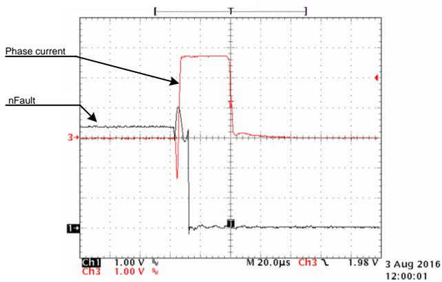
**Figure 52. Short-Circuit Current Between Motor Terminal Phase A to GND and SM72295 nFAULT Signal**
