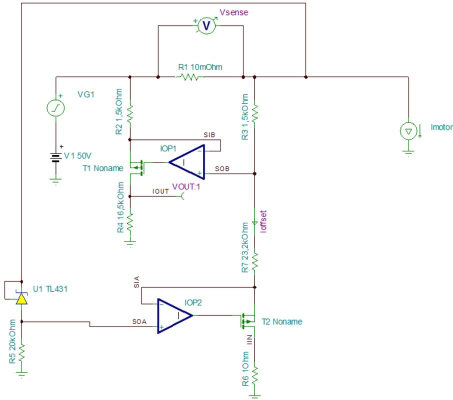
**Figure 11. TI-TINA™ Simulation Circuit of Implement Current Sense Solution**
