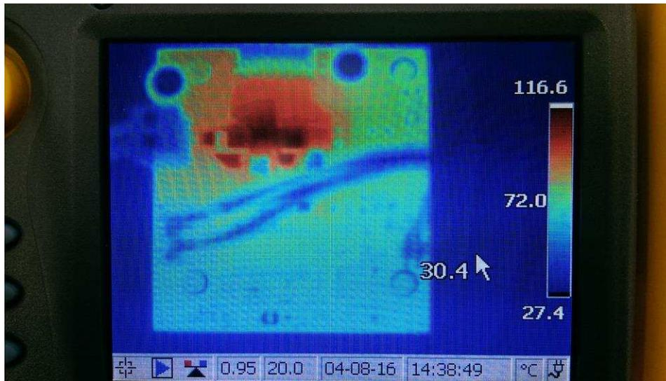
Figure 45. Peak Temperature of TIDA-00210 at 75 V, 10 A, No Air Cooling, No Heat Sink
