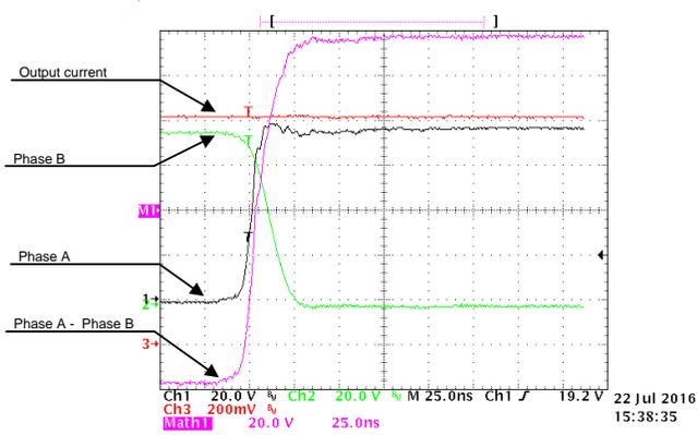
Figure 33. Rising Edge of Output Voltage, Phase A and B Voltage to GND at 10-A Output Current
