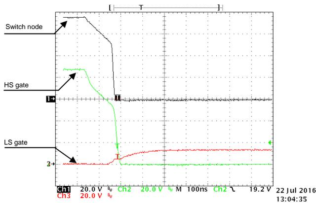
Figure 25. Phase A Falling Switch Node Voltage, High-Side, and Low-Side Gate to GND at 1-A Output Current
