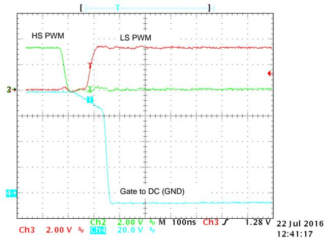
Figure 24. SM72295 High-Side Gate Driver Output Voltage versus GND During Turnoff
