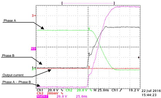
Figure 35. Rising Edge of Output Voltage, Phase A and B Voltage to GND at -10-A Output Current
