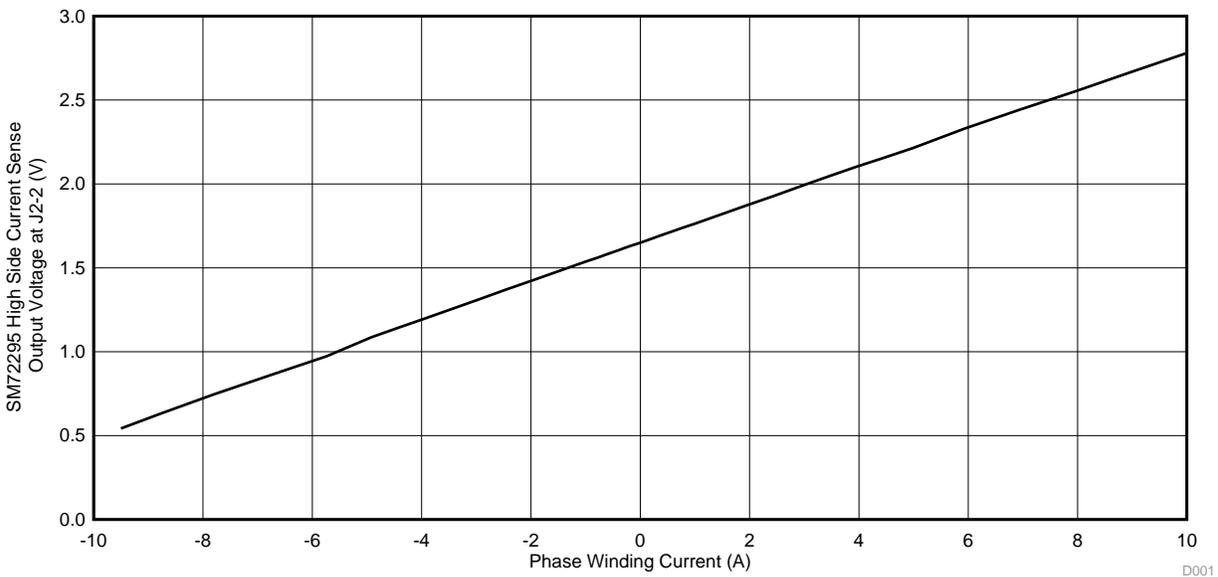
**Figure 42. SM72295 Current Sense Amplifier Output Voltage at J5-2 Sampled at PWM Center versus Measured Phase Winding Current (Fluke Ampere Meter)**
