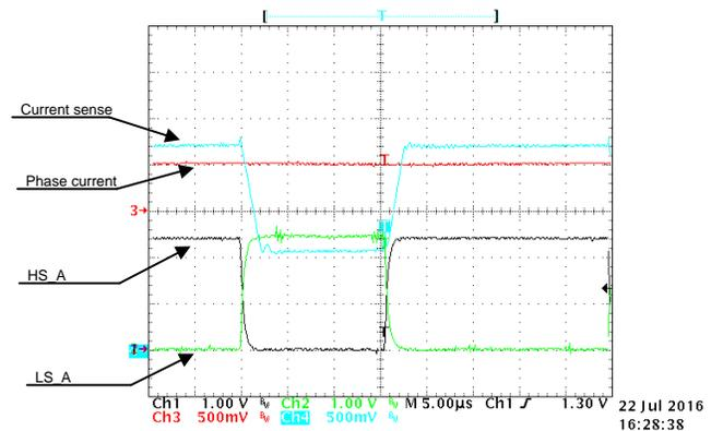
Figure 39. Host Interface Analog Signals, Current Sense Amplifier at J2-2 With  $I_{ref}$  5 A at 25-kHz PWM, Phase A and Phase B J2
