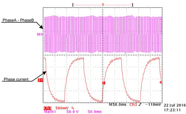
Figure 46. Full-Bridge Output Voltage and Output Current at  $\pm 9.4\text{-A}$  Current Magnitude Toggling at 80 ms
