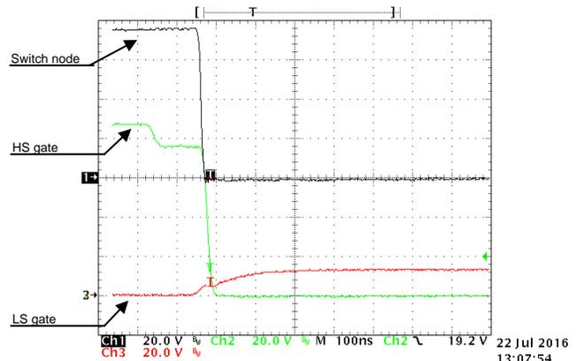
Figure 28. Phase A Falling Switch Node Voltage, High-Side, and Low-Side Gate to GND at -1-A Output Current
