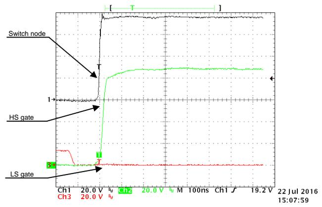
Figure 30. Phase A Rising Switch Node Voltage, High-Side, and Low-Side Gate to GND at 10-A Output Current
