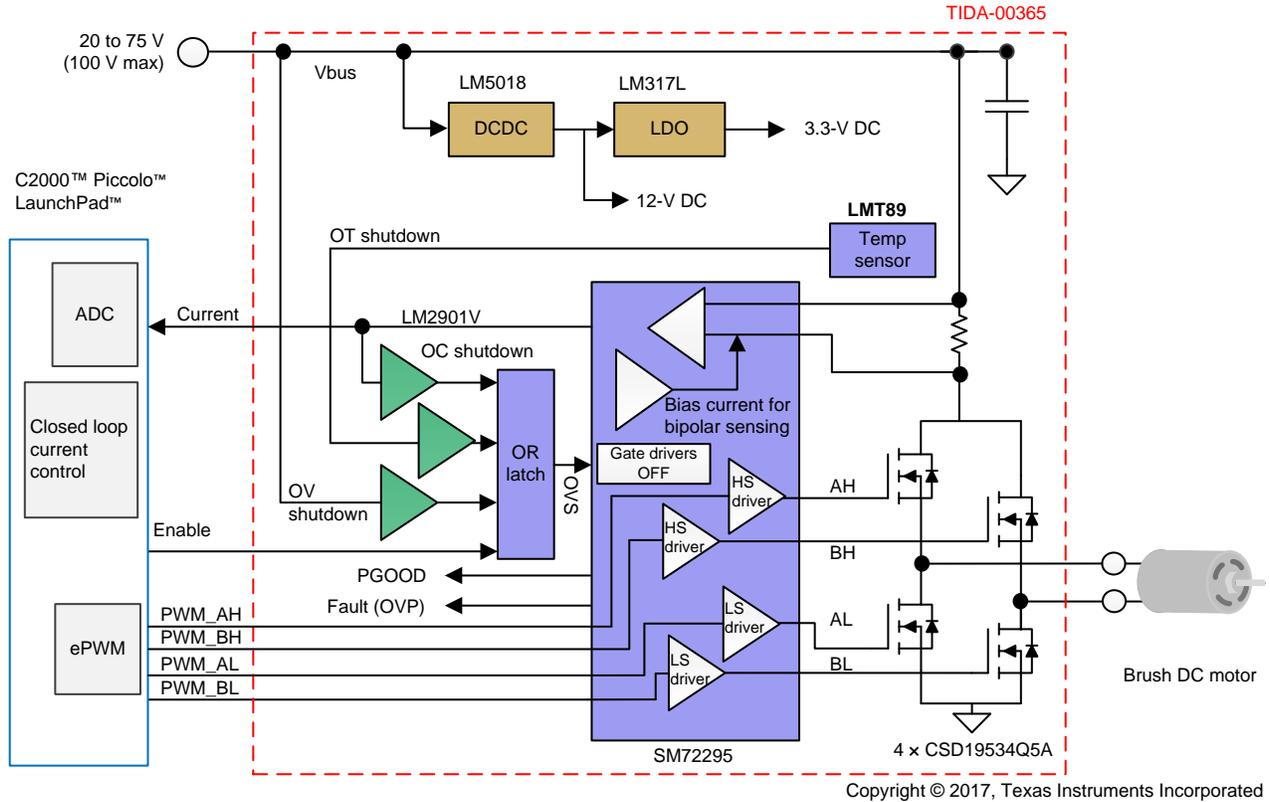
Figure 2. TIDA-00365 Block Diagram
