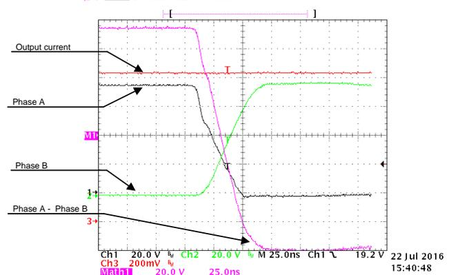
Figure 34. Falling Edge of Output Voltage, Phase A and B Voltage to GND at 10-A Output Current
