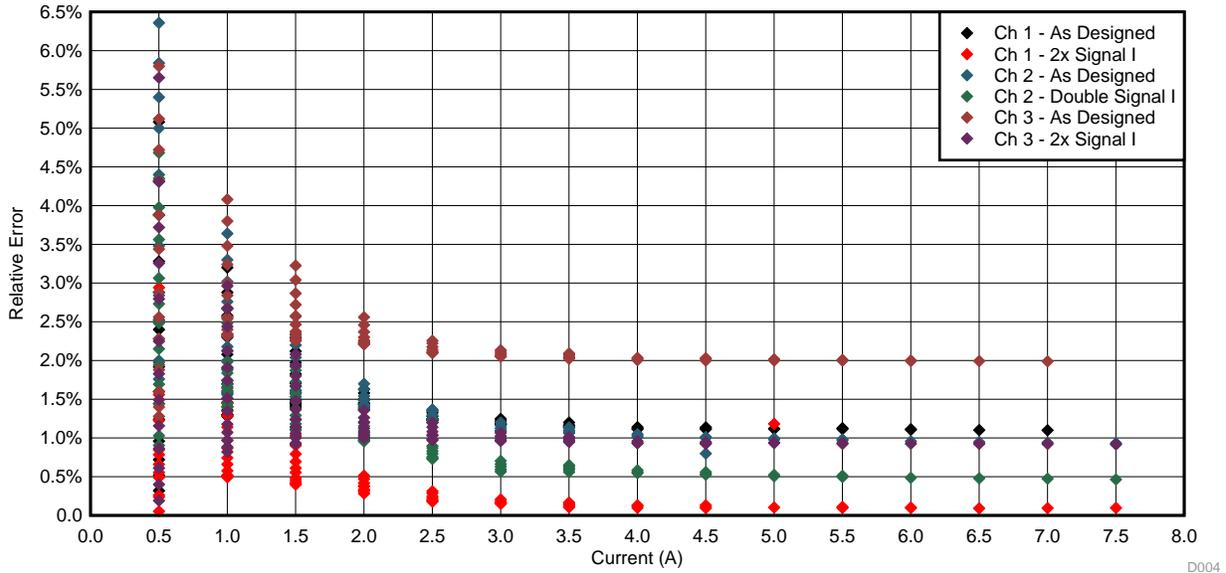
Figure 20. Uncalibrated Relative Error of Current Sense Measurement versus Current
