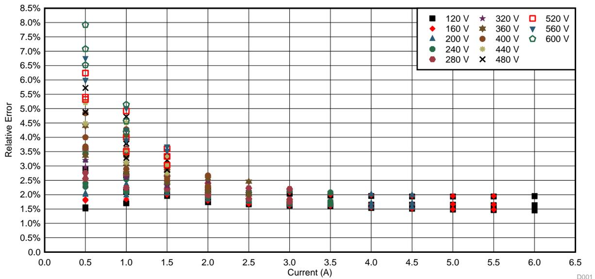
Figure 17. Uncalibrated Relative Error of Current Sense Measurement versus Current
