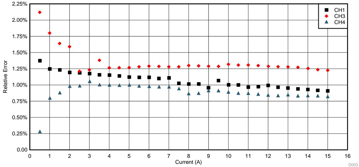
Figure 19. Uncalibrated Relative Error versus Current for 95-V DC Bus
