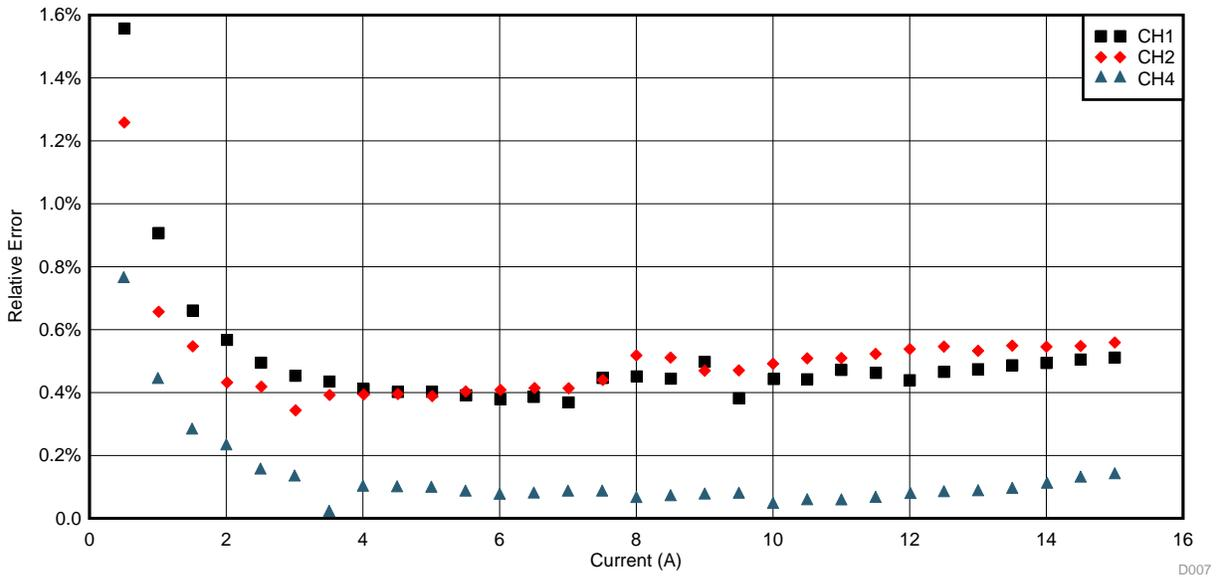
Figure 23. Relative Error versus Current With Calibration Across Full Current Range
