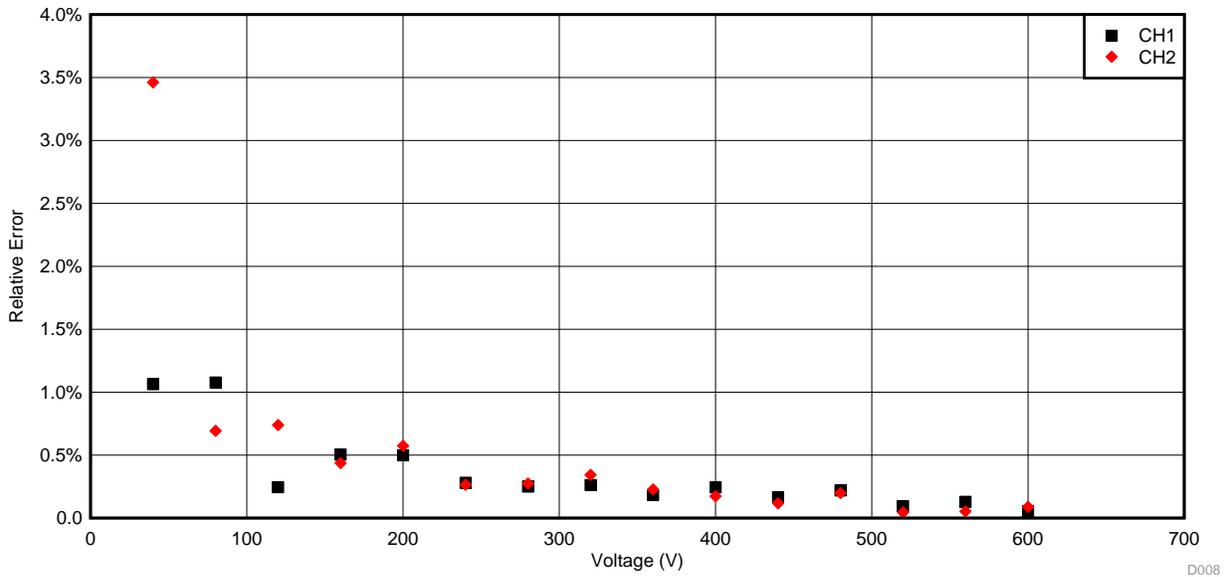
Figure 24. Relative Error of Voltage Sense Measurement versus Voltage
