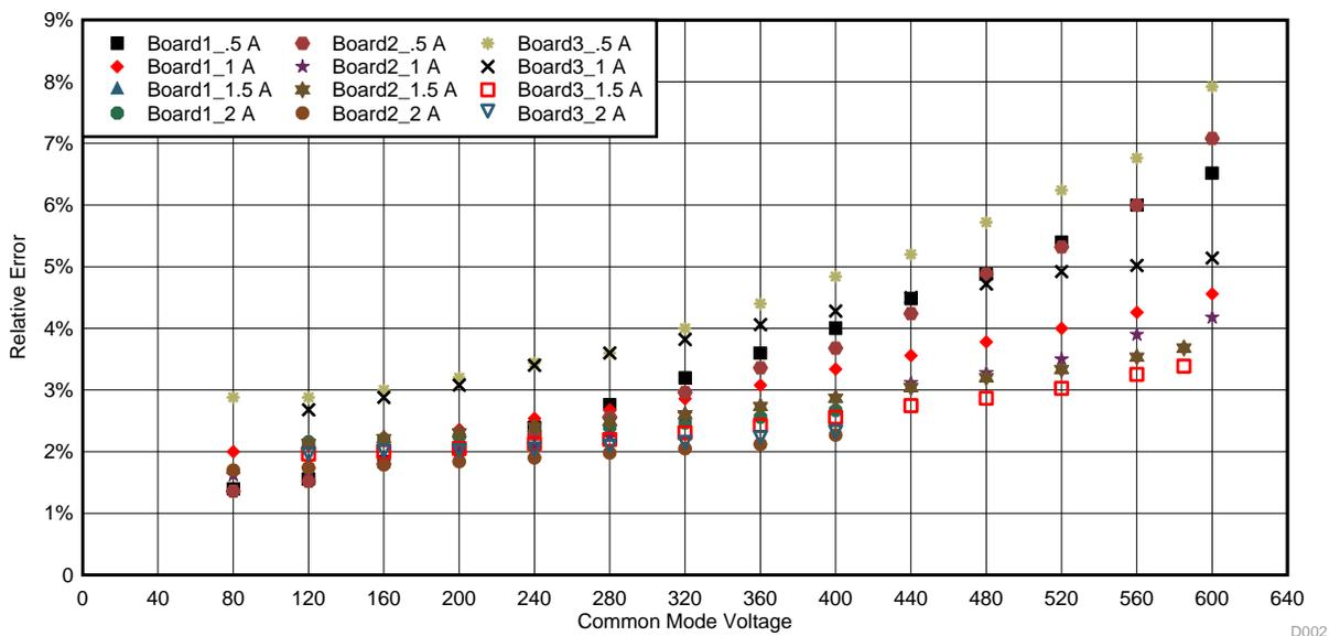
Figure 18. Uncalibrated Relative Error versus Common-Mode Voltage
