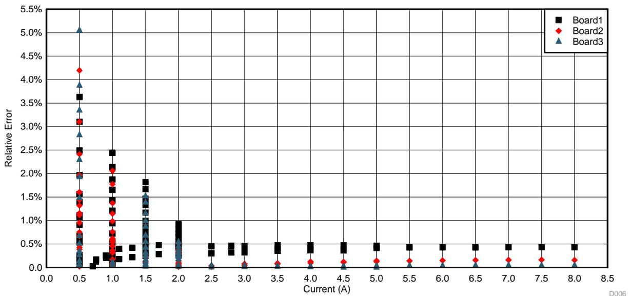
Figure 22. Relative Error versus Current With Calibration Across Full Voltage Range
