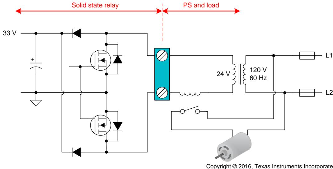
**Figure 10. Power Supply of SSR in HVAC System**
