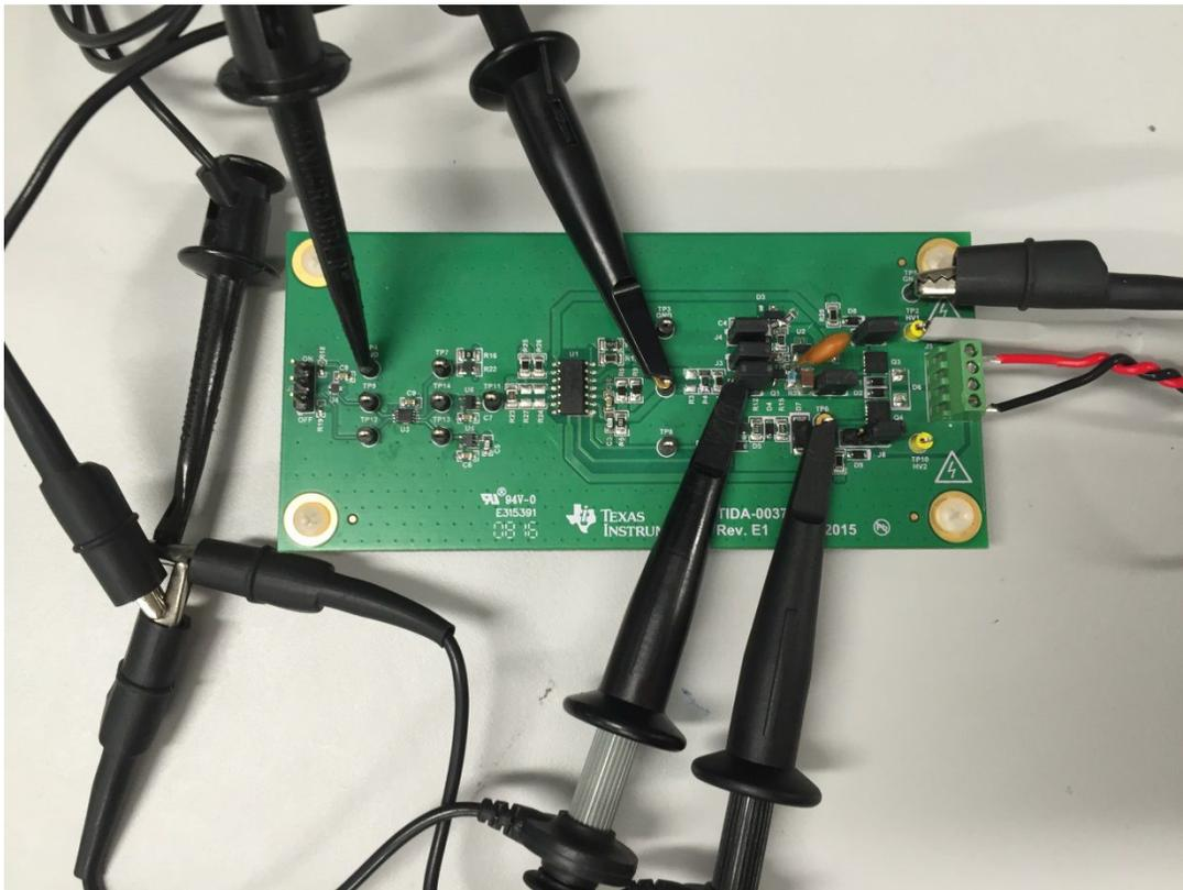
**Figure 25. Probe Connections for Signal Chain Waveforms**
