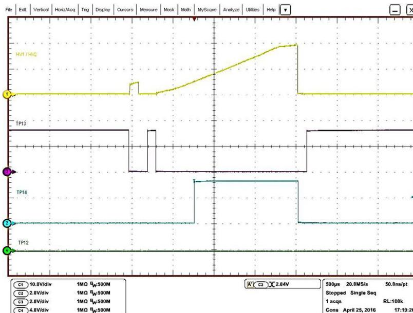
Figure 31. OCP Waveform During Charging Time in Reference to HV1/HV2 (Yellow), TP13 (Purple), TP14 (Blue), and TP12 (Green)
