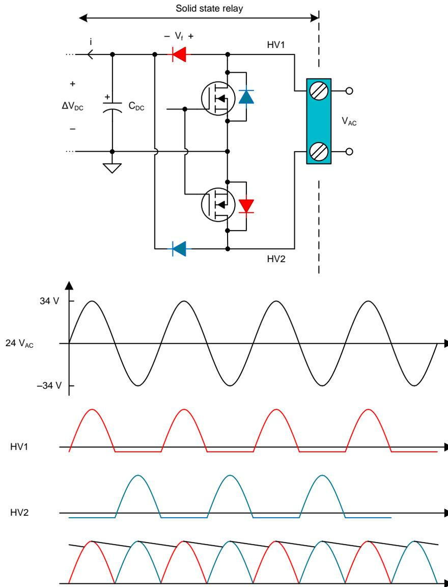
**Figure 11. Full-Wave Rectification Circuitry and Waveforms**
