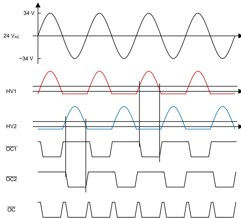
Figure 18. Resulting Output Waveforms of OCP When MOSFETs are Off
