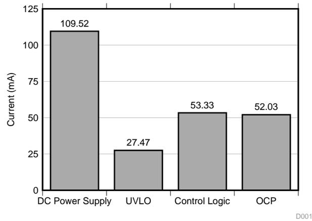
**Figure 26. Steady-State Current Consumption During ON Time**
