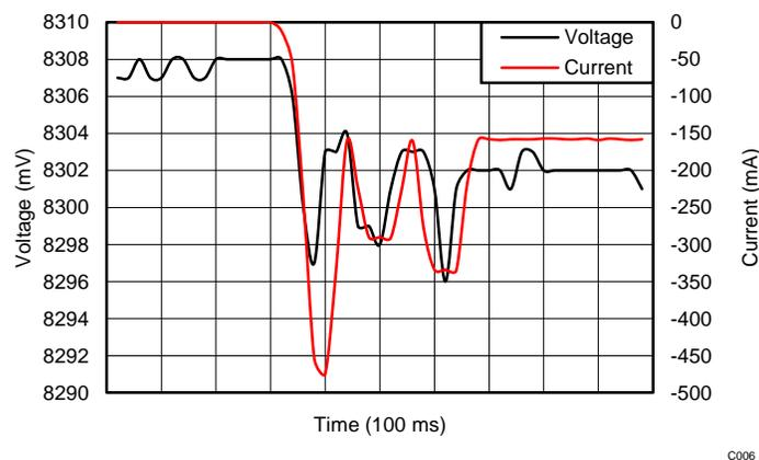
Figure 17. TIDA-00982 Initial Power Up of the Drone
