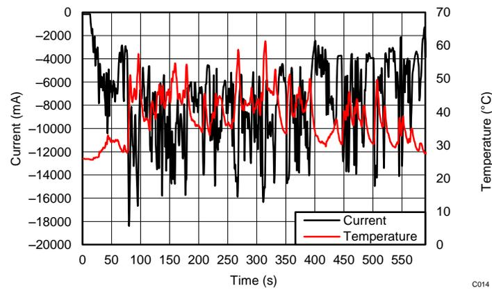
**Figure 25. TIDA-00982 Drone Current vs Chg\_Dschg\_Mosfet Temperature**
