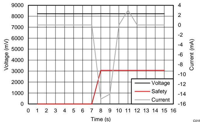
**Figure 26. TIDA-00982 Safety Alert Short Circuit**
