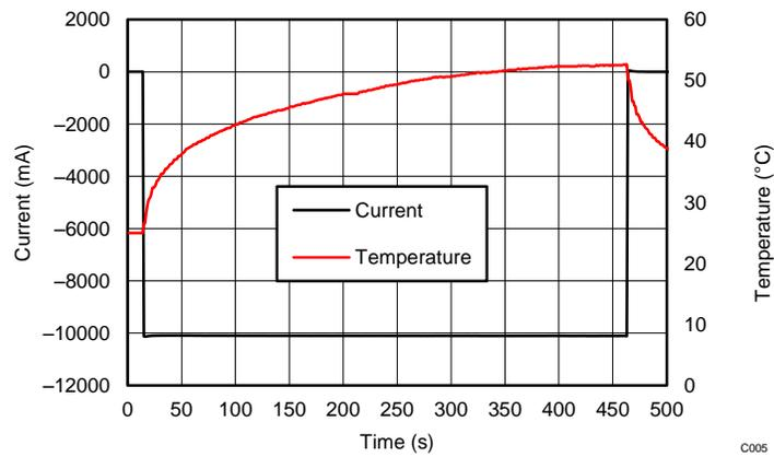
Figure 16. TIDA-00982 10 A Discharge Mosfet Current vs Temperature
