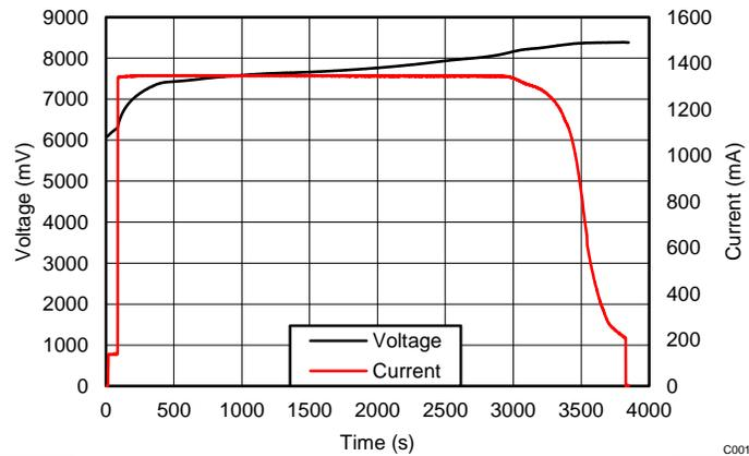
Figure 12. TIDA-00982 1.3 A Charge Cycle
