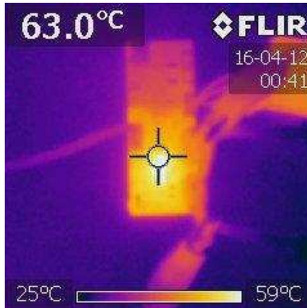
**Figure 31. TIDA-00982 Maximum Temperature During All Rotors Full On**
