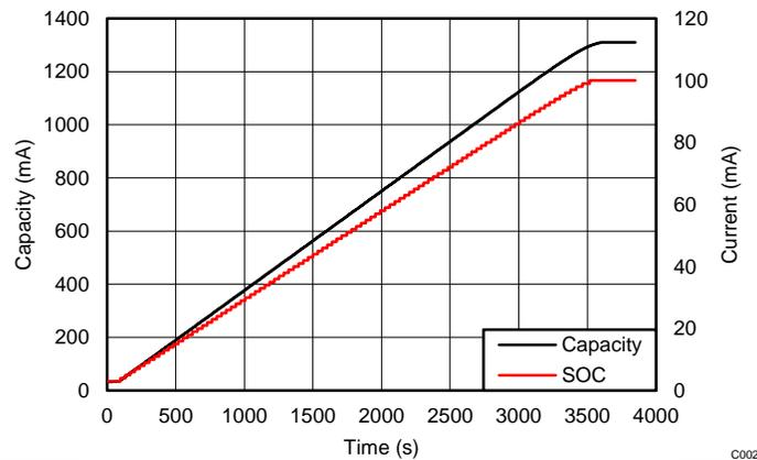
Figure 13. TIDA-00982 1.3 A Charge Capacity vs SOC
