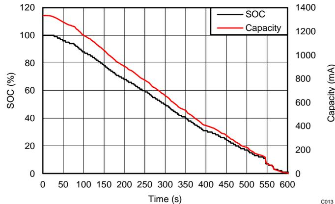
Figure 23. TIDA-00982 Drone in Flight Discharge
