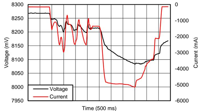
**Figure 19. TIDA-00982 Drone Low Speed Run**
