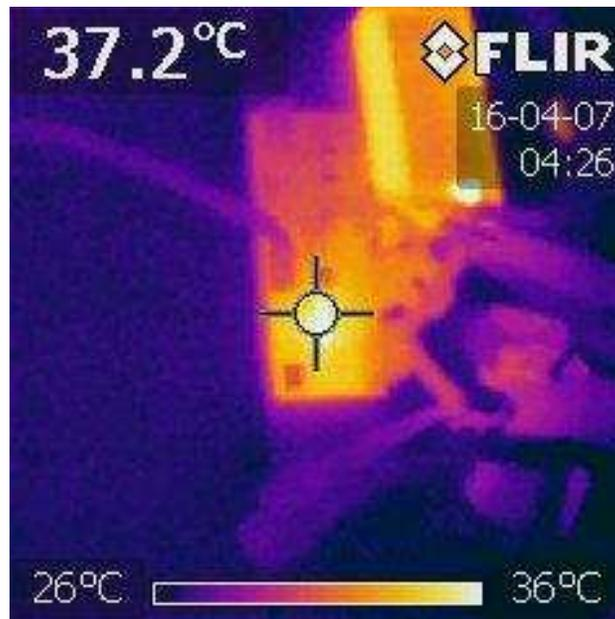
**Figure 29. TIDA-00982 Temperature During 1C Discharge**
