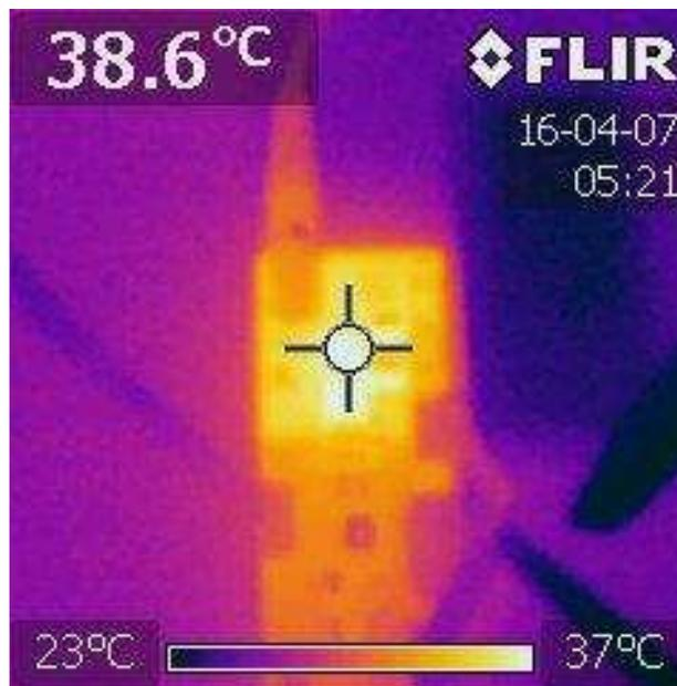
Figure 28. TIDA-00982 Temperature During a 1C Charge
