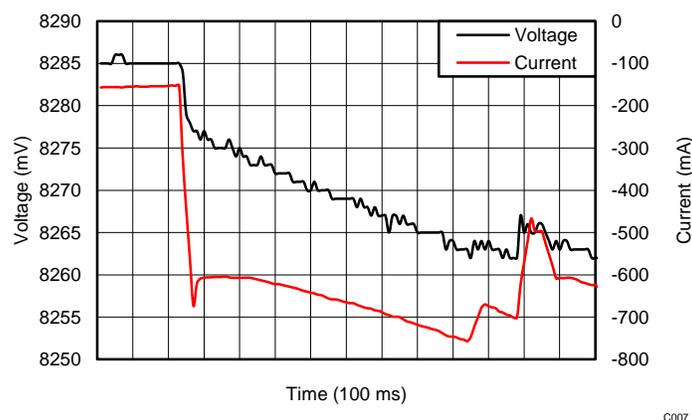
Figure 18. TIDA-00982 Drone Rotor Start Up
