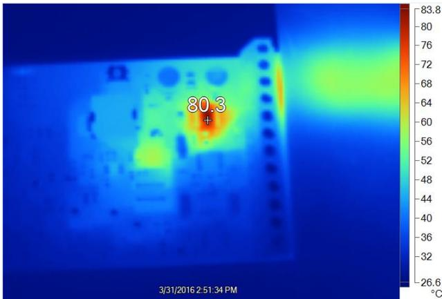
Figure 32. TPS92630-Q1 Linear LED Driver-Temperature at Three Strings of 100-mA LEDs
