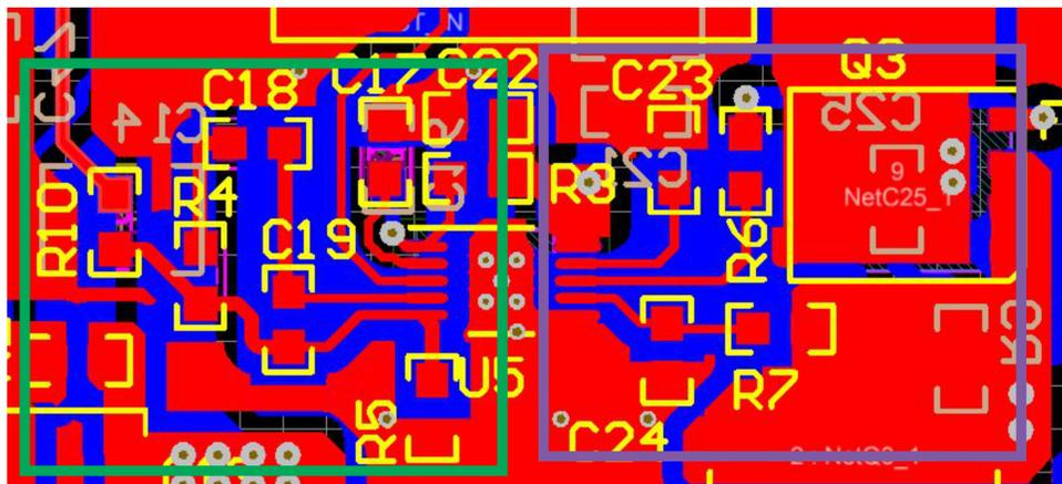
Figure 57. Switching-Converter Routing
