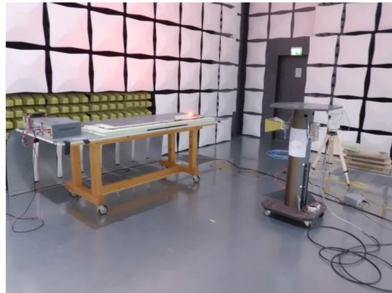
**Figure 51. Radiated Emissions Setup With a Horn Antenna: 1.447 GHz to 1 GHz**
