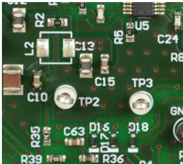
Figure 27. Resistors R2 and R35
