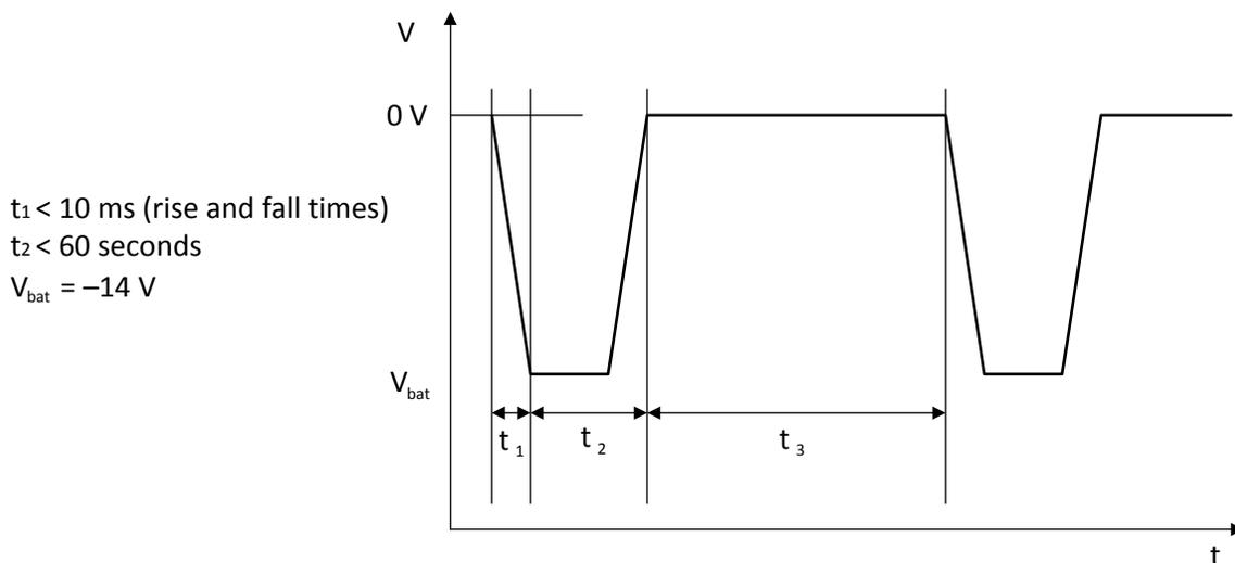
**Figure 10. Reverse-Battery Pulse**
