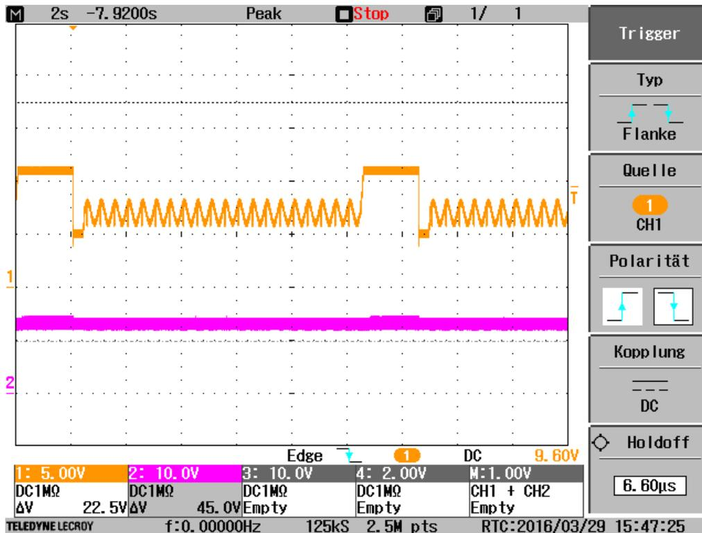
Figure 44. Cold-Crank Test
