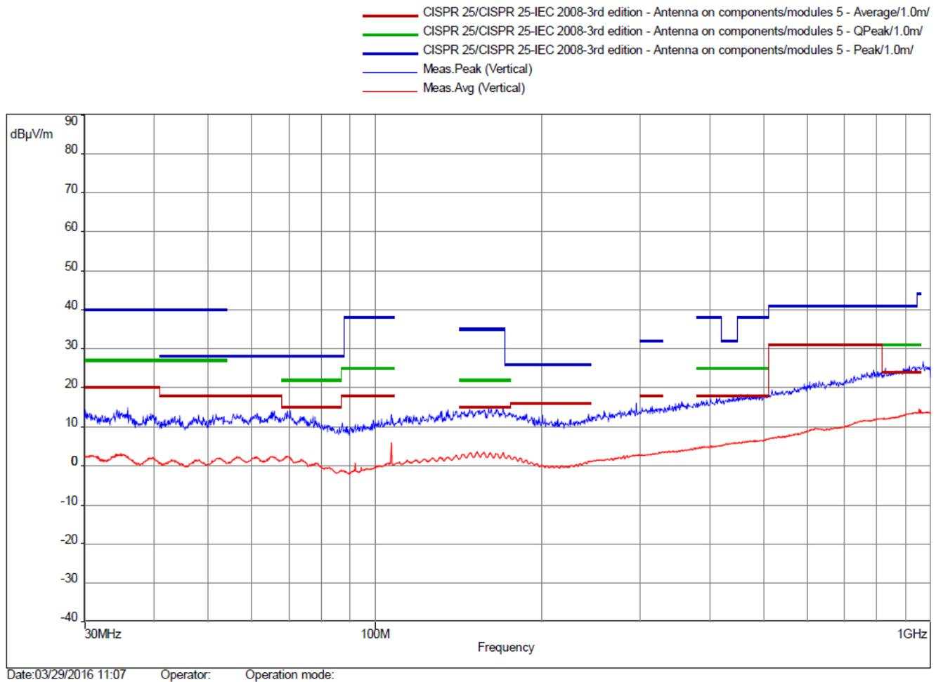
**Figure 52. Ambient-Noise Level of Radiated Emissions: Line Side 30 MHz to 1 GHz**
