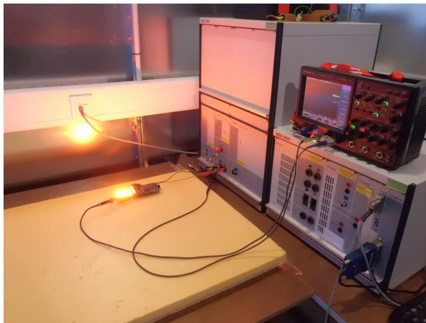
Figure 29. Setup for Transient Tests With LED Board and NSG 5500 Transient Generator
