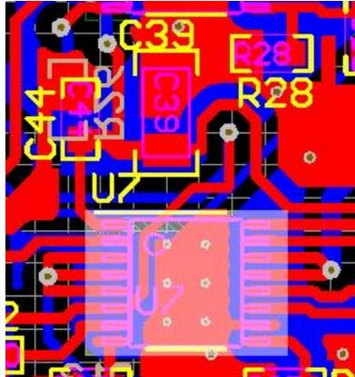
Figure 59. Input and Output Capacitor Placement
