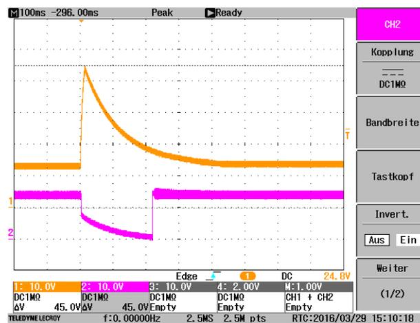
Figure 39. Load Dump and Output of TPS92630-Q1: Turned Off at > 17 V then Turned On
