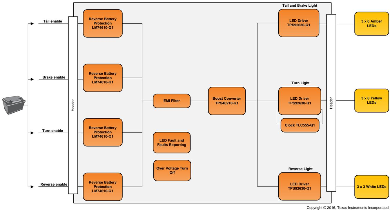
**Figure 1. Tail-Light System Driven Off of a Battery**
