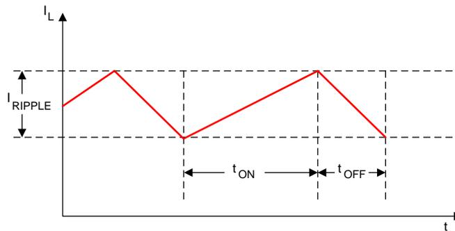
Figure 17. Input-Current Waveform
