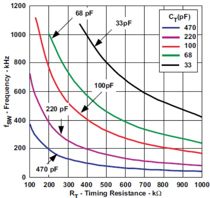
Figure 15. Switching Frequency versus Timing Resistance
