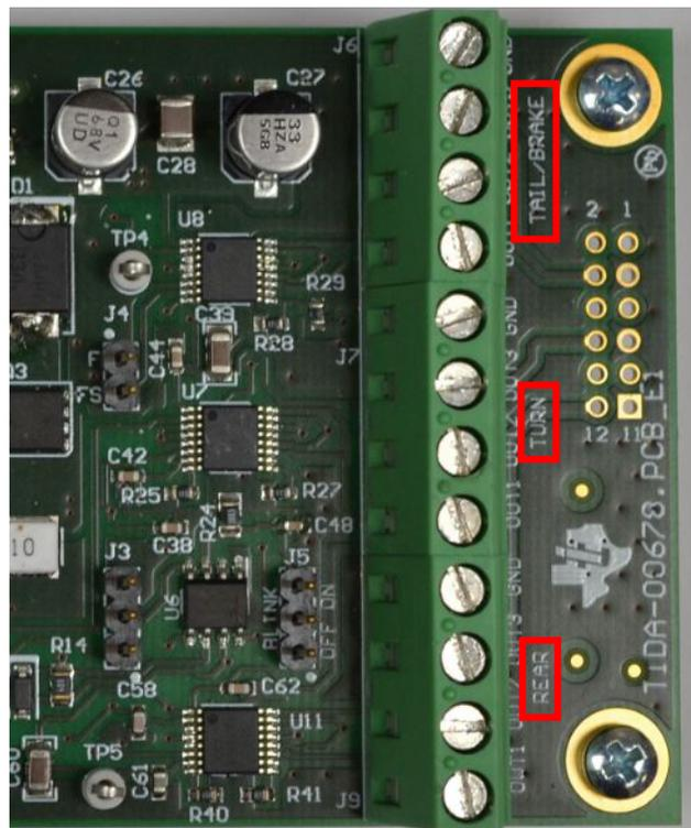
**Figure 22. Screw Terminals for LED-String Outputs (100 mA and 150 mA, Maximum of 9 Strings, Maximum Output Voltage of 16.5 V)**
