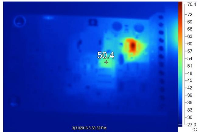
Figure 33. TPS40210-Q1 Boost-Converter Temperature Above 50°C at Three Strings of LEDs at 100 mA
