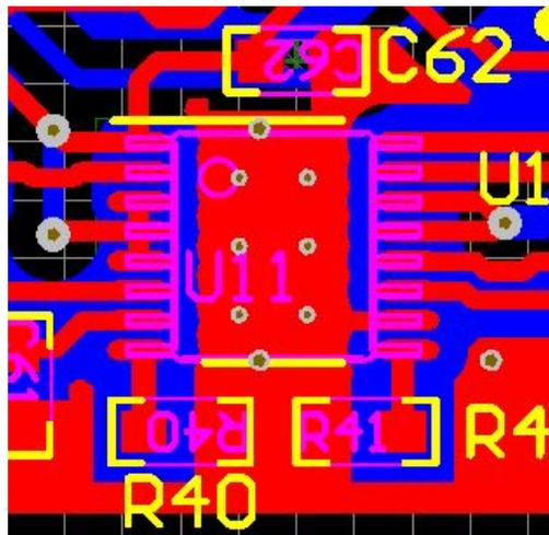
**Figure 55. TPS92630-Q1 Thermal Vias Under LED Driver**
