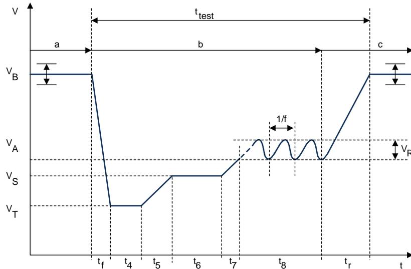
Figure 43. Cold-Crank Wave Shape
