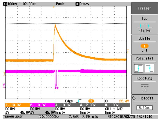
Figure 38. Load Dump and Output of TPS92630-Q1: With Thermal Toggling and No Turnoff
