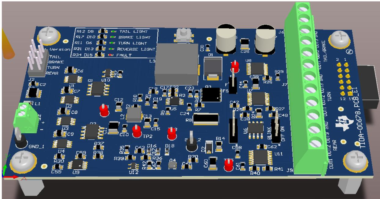
**Figure 12. 3D Render of the TIDA-00678 Board**
