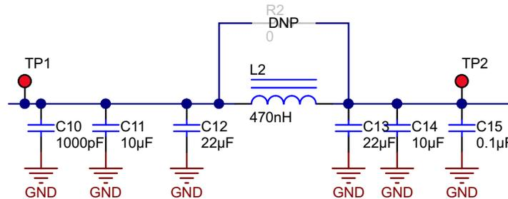
Figure 16. Input Voltage-Noise Filtering (R2 is Optional)
