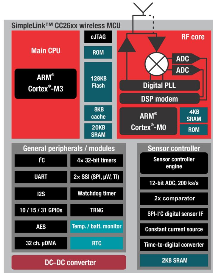
Figure 3. CC2650 Internal Block Diagram
