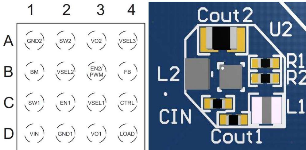
Figure 7. TPS62770 Device Pinout and Layout
