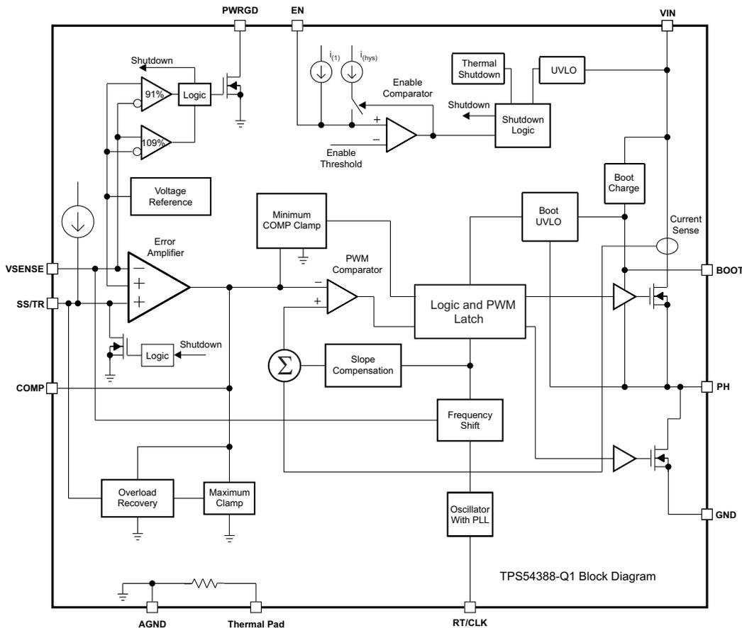
Figure 7. TPS5488-Q1 Functional Block Diagram
