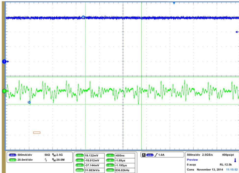
Figure 35. LM26420-Q1 3.3V Output Voltage Ripple with a 1 A Load
