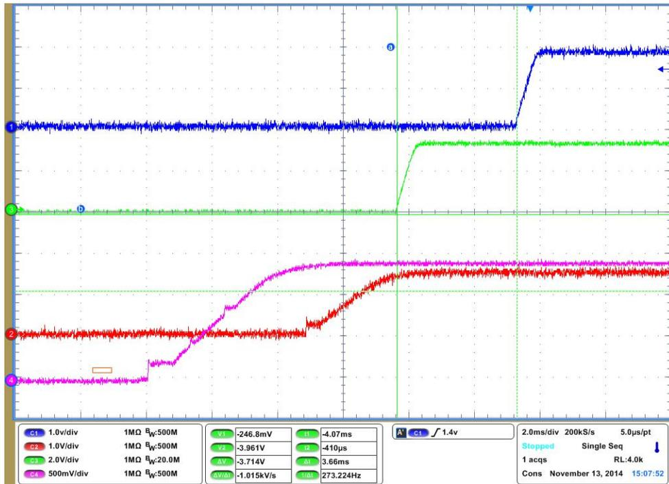
Figure 42. Power-Up Relationships of the 1.8 V, 1.5 V, 3.3V and 1.425 V supplies
