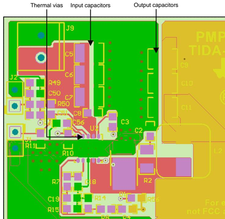
**Figure 48. TPS54561-Q1 Input and Output Capacitor Placement Ground = Green, +5 V = Yellow**
