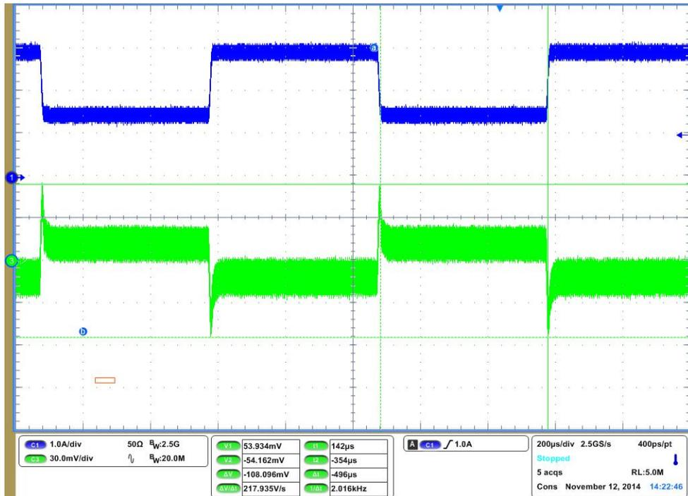
Figure 22. TPS54388 Load Step Response, 1.5 A to 3 A
