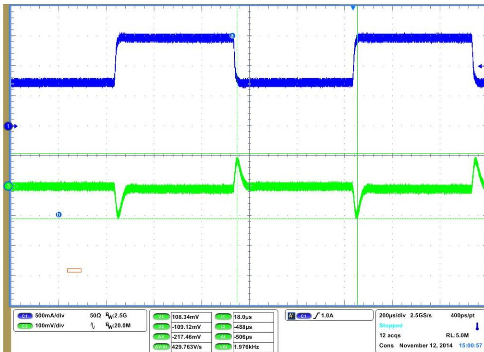
Figure 37. LM26420-Q1 3.3 V Load Step Response, 0.75 A to 1.5 A
