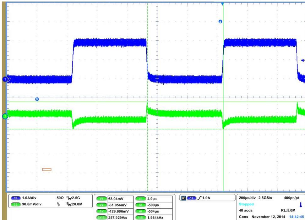
Figure 26. TPS57114-Q1 Load Step Response, 0 A to 2 A
