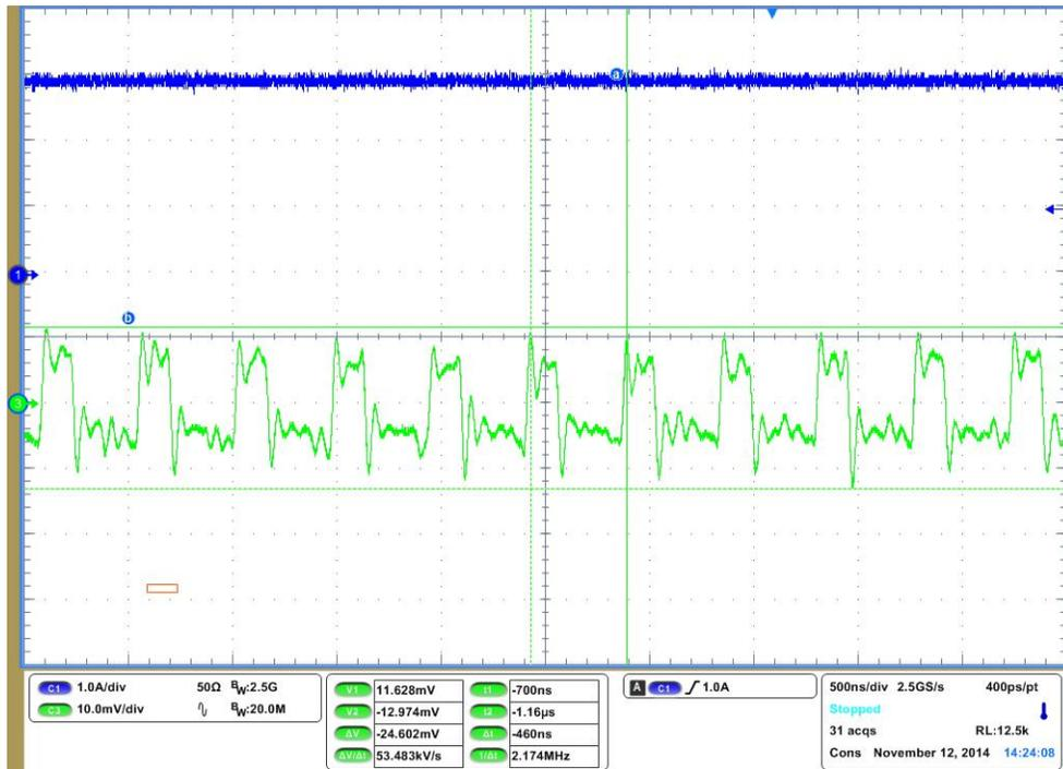
**Figure 20. TPS54388-Q1 Output Voltage Ripple**
