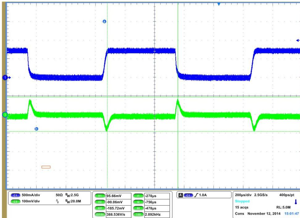
Figure 36. LM26420-Q1 3.3 V Load Step Response, 0 A to 0.75 A
