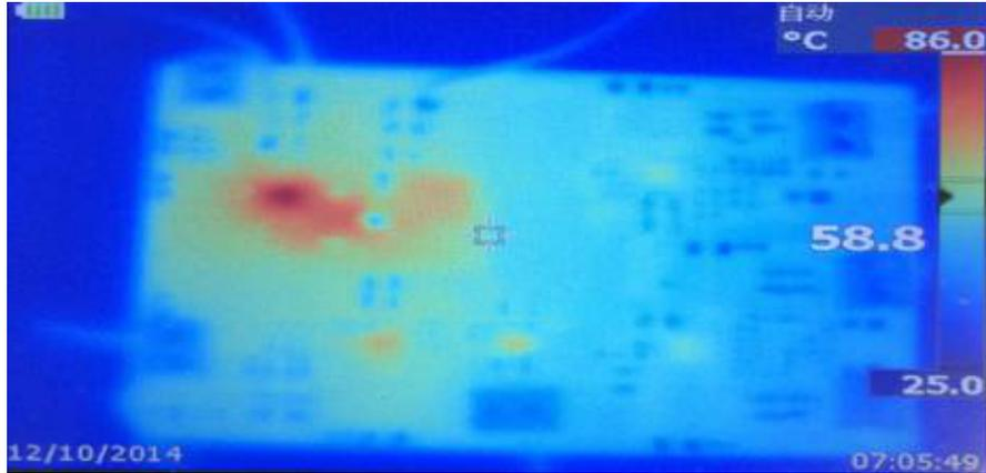
Figure 43. Thermal image of the TIDA-00804 board with maximum loads
