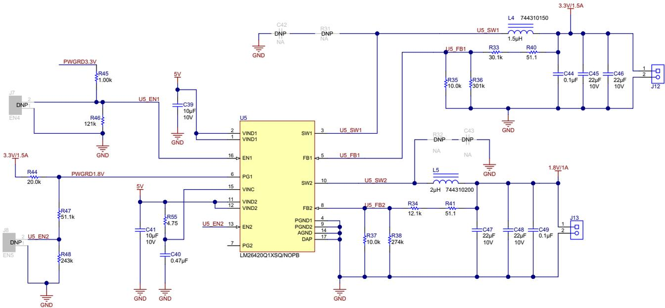
Figure 13. LM26420-Q1 Circuit
