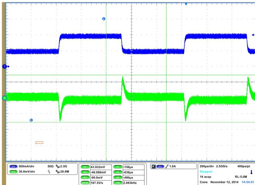
Figure 32. LM26420-Q1 Load Step Response, 0.5 A to 1 A
