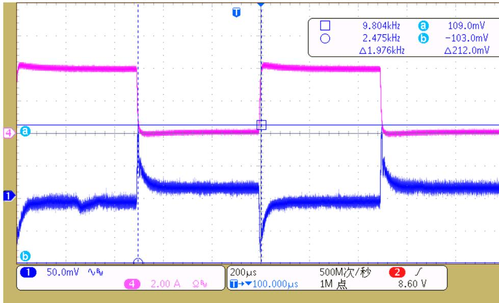
Figure 28. TPS57114-Q1 Load Step Response, 0 A to 4 A
