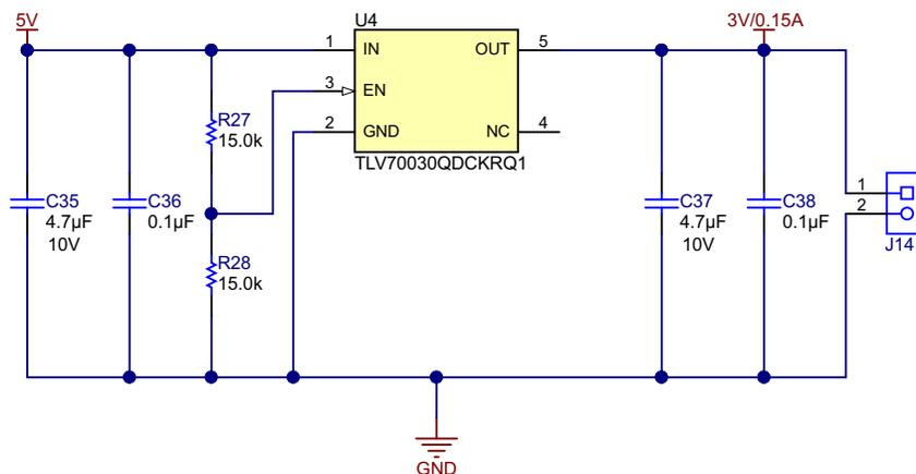
Figure 10. TLV70030-Q1 Circuit
