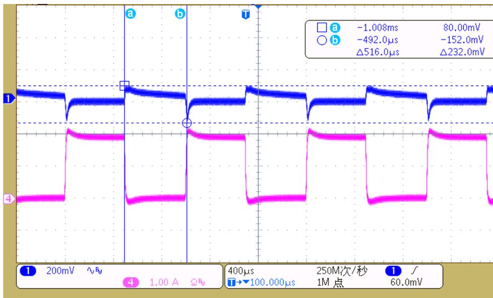
Figure 16. TPS54561-Q1 Load Step Response, 0 A to 2 A
