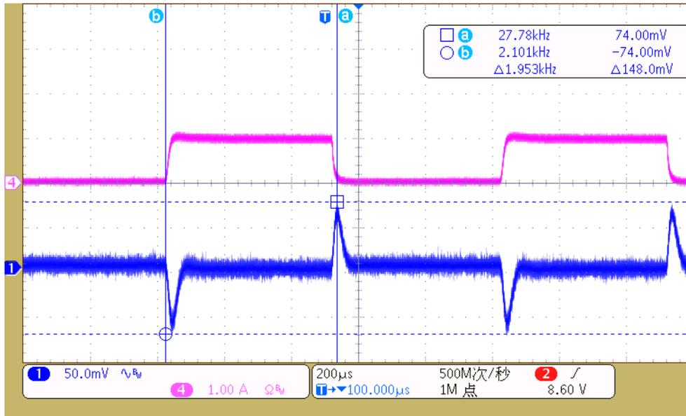
Figure 33. LM26420-Q1 Load Step Response, 0 A to 1 A
