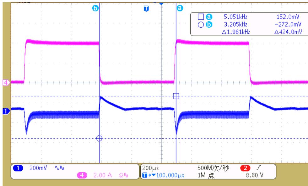
Figure 18. TPS54561-Q1 Load Step Response, 0 A to 4 A
