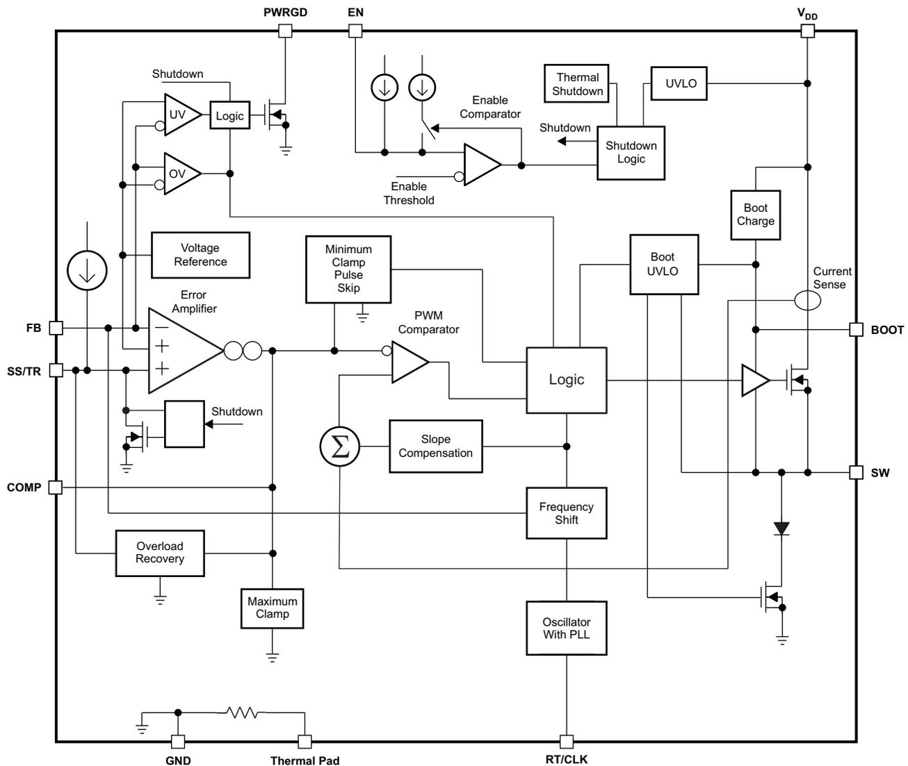
Figure 4. TPS54561-Q1 Functional Block Diagram
