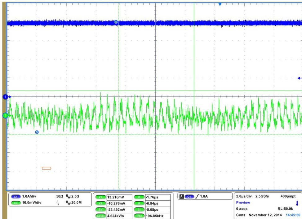
Figure 25. TPS57114-Q1 Output Voltage Ripple With a 4-A Load
