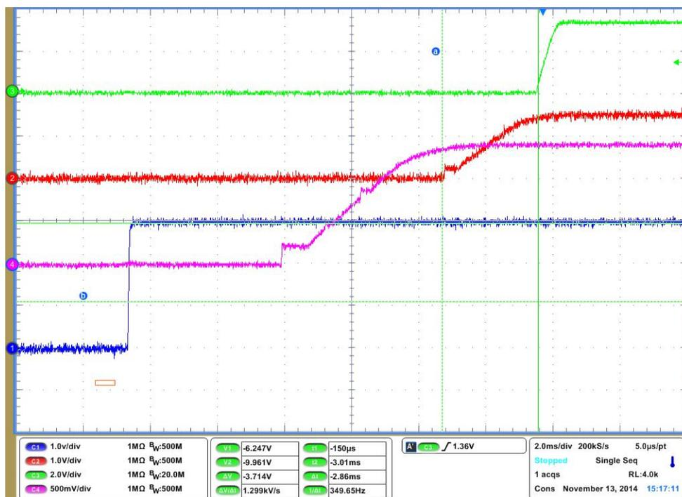
Figure 41. Power-Up Relationships of the 3 V, 1.5 V, 3.3V and 1.425 V Supplies
