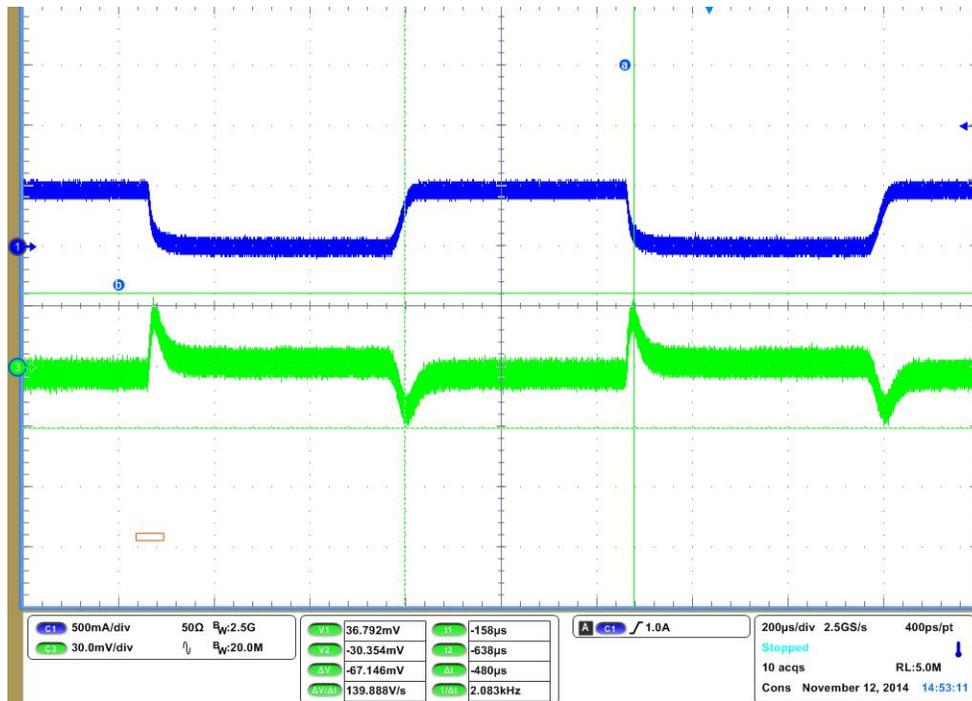
Figure 31. LM26420-Q1 Load Step Response, 0 A to 0.5 A
