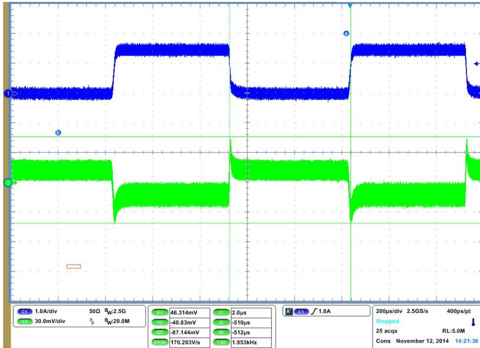
Figure 21. TPS54388 Load Step Response, 0 A to 1.5 A
