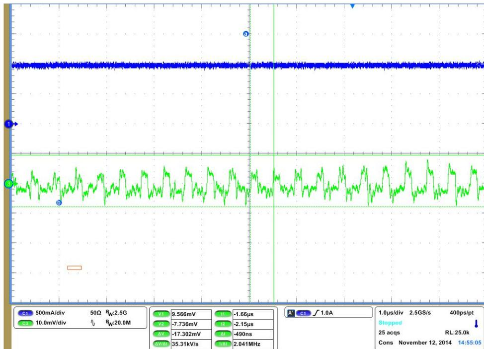
Figure 30. LM26420-Q1 1.8V Output Voltage Ripple with a 1 A Load
