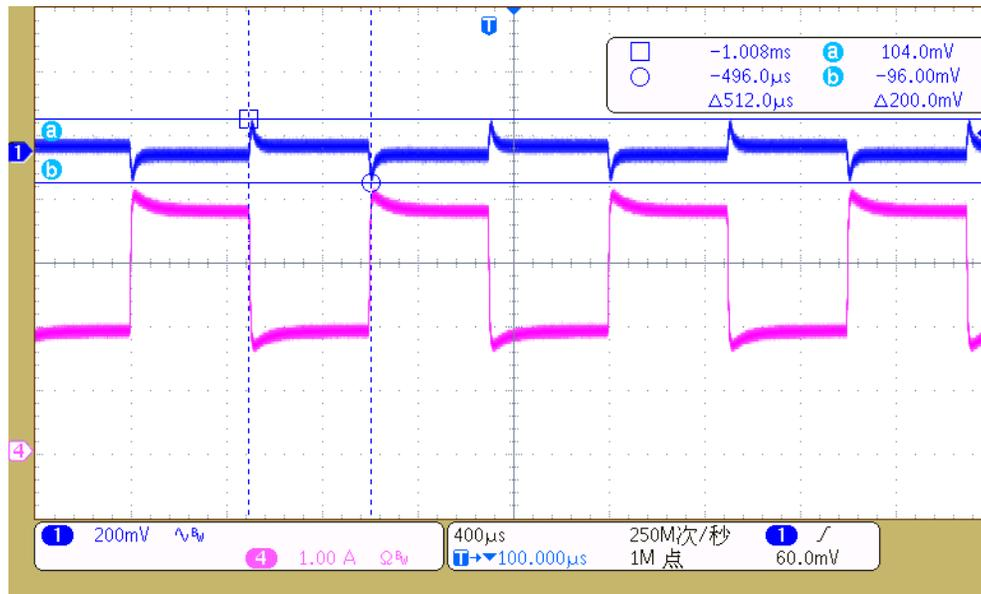
Figure 17. TPS54561-Q1 Load Step Response, 2 A to 4 A
