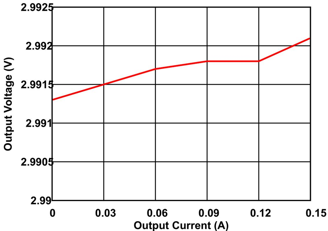
**Figure 39. TLV70030-Q1 Load Regulation**
