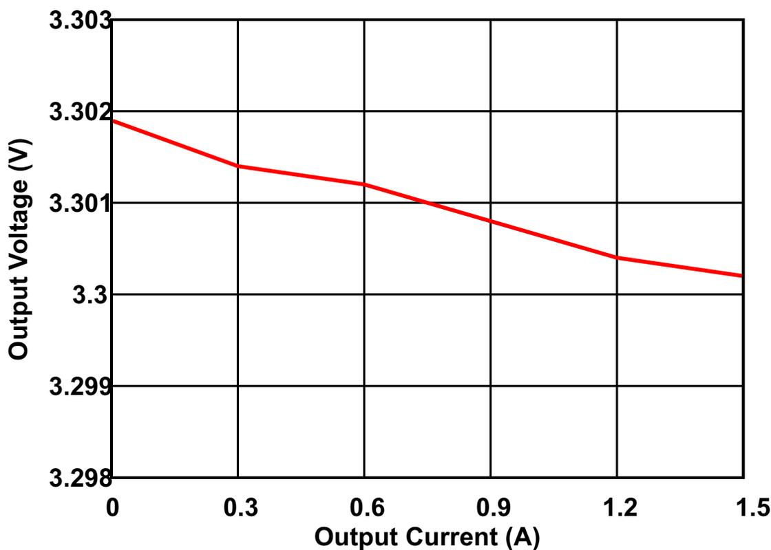
**Figure 34. LM26420-Q1 Load Regulation**
