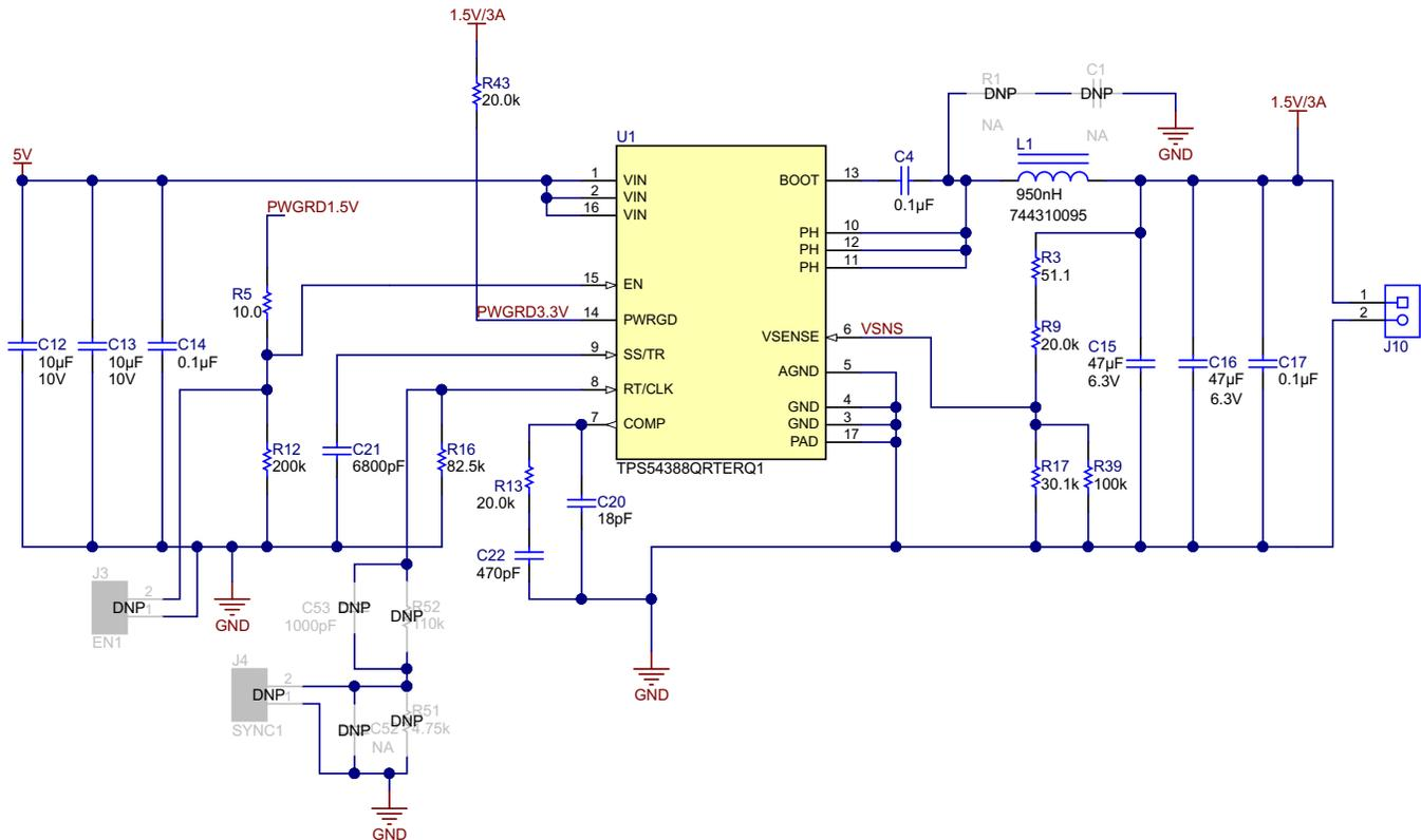
Figure 12. TPS54388-Q1 Circuit
