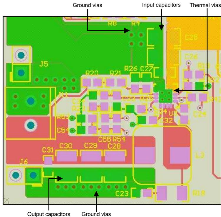
**Figure 49. TPS57114-Q1 Input and Output Capacitor Placement Ground = Green, +5V = Yellow**
