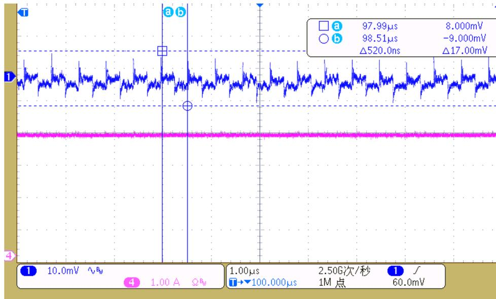
Figure 15. TPS54561-Q1 Output Ripple Voltage
