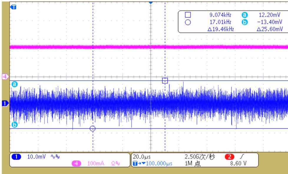
Figure 40. TLV70030-Q1 Output Voltage Ripple With a 0.15 A Load
