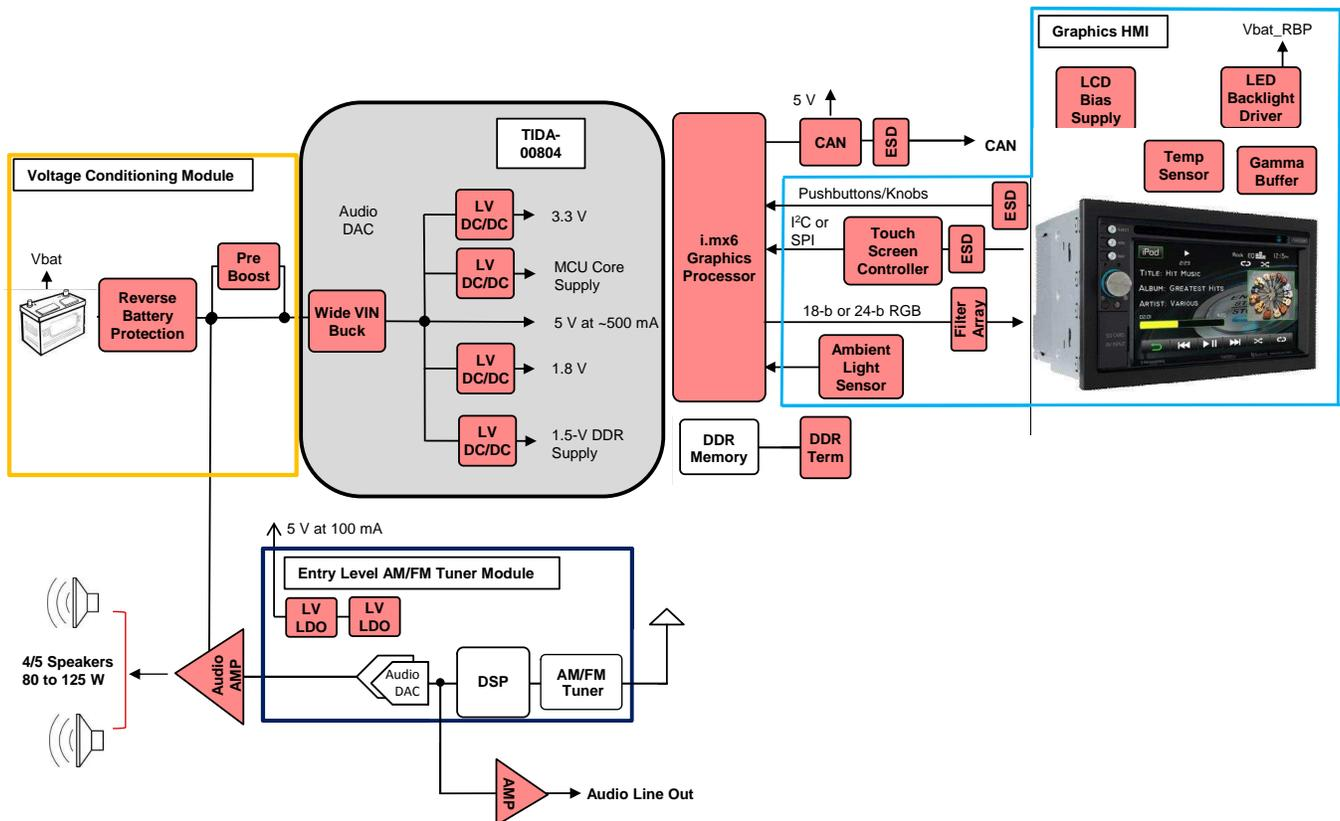
Figure 2. System Level Block Diagram of a Head Unit With a Graphics Display
