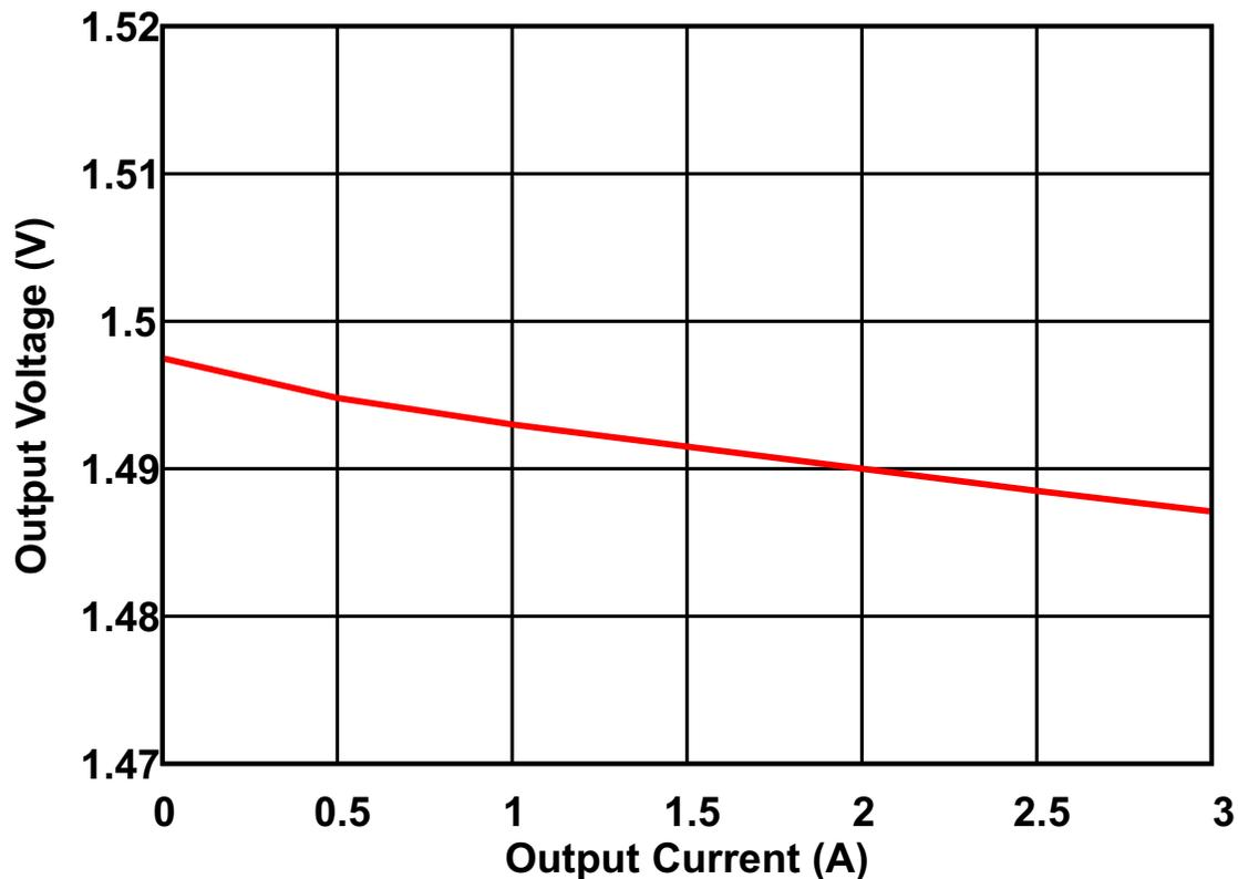
**Figure 19. TPS54388-Q1 Load Regulation**
