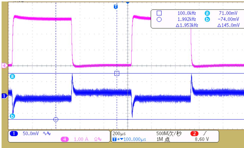
Figure 23. TPS54388 Load Step Response, 0 A to 3 A.
