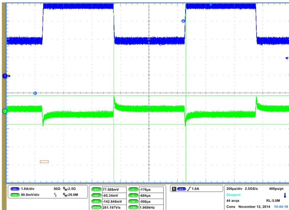
Figure 27. TPS57114-Q1 Load Step Response, 2 A to 4 A.
