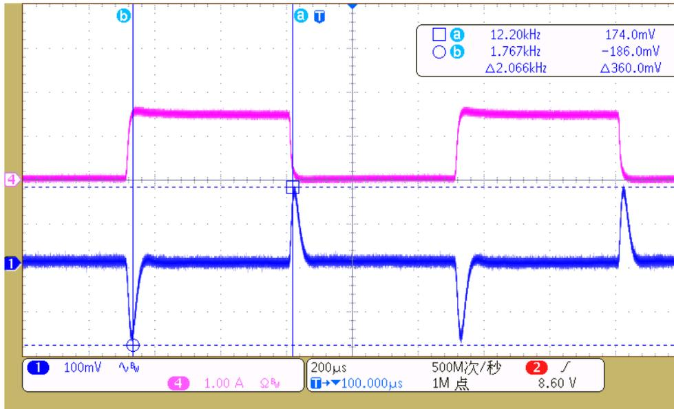
Figure 38. LM26420-Q1 3.3 V Load Step Response, 0 A to 1.5 A
