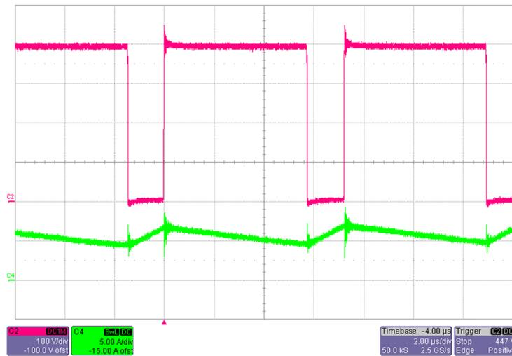
Figure 12. SW Node Waveform and MOSFET Current at  $V_{INAC} = 230\text{-V AC}$ , Full Load
