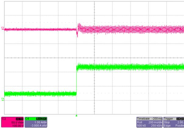
**Figure 21. Output Voltage Waveform at  $V_{INAC} = 230\text{ V}$ , Load Transient From 0.5 to 2.56 A**
