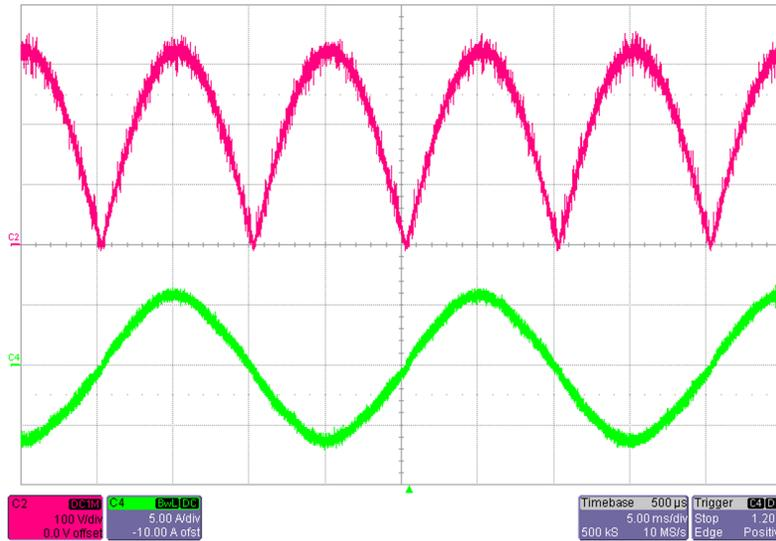
Figure 15. Input Voltage and Input Current at  $V_{INAC} = 230\text{-V AC}$ , Full Load
