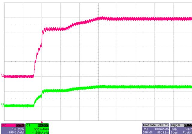
Figure 19. Output Turn-on Waveform at  $V_{INAC} = 230\text{ V}$  With Light Load of 0.5 A
