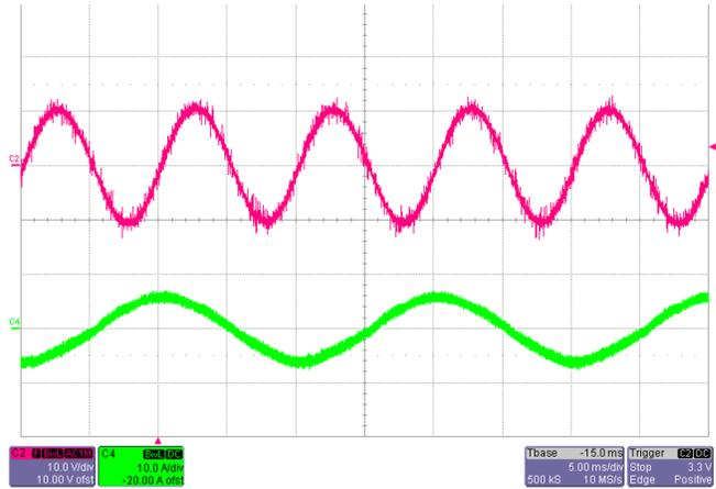
Figure 18. Output Voltage Ripple at  $V_{INAC} = 230\text{ V}$ , Full Load, Only 50-Hz Component
