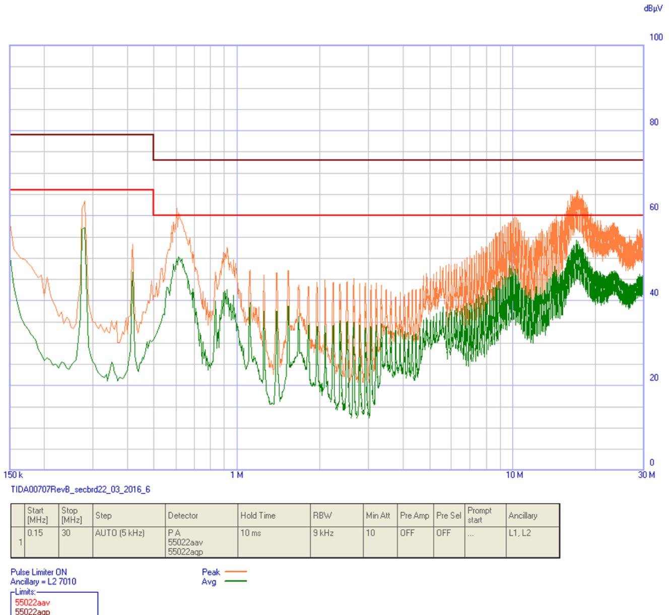
Figure 23. Conducted Emissions as per EN55011 Class A
