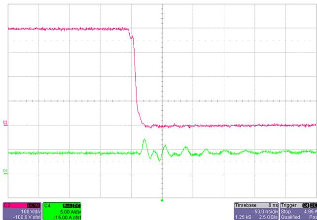
Figure 13. SW Node Waveform Turn-on Cycle at  $V_{INAC} = 230\text{-V AC}$ , Full Load
