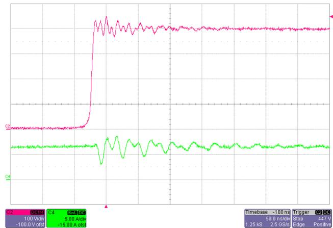
Figure 14. SW Node Waveform Turn-off Cycle at  $V_{INAC} = 230\text{-V AC}$ , Full Load
