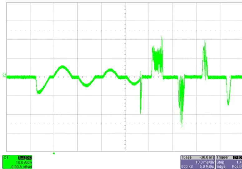
Figure 16. Output Voltage and Input Inrush Current at  $V_{INAC} = 230\text{ V}$ , Full Load
