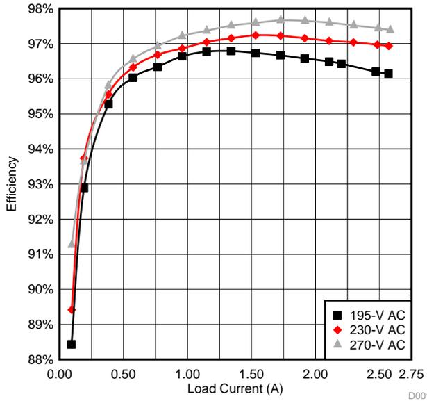
Figure 8. Efficiency versus Output Load Current ( $I_{OUT}$ )
