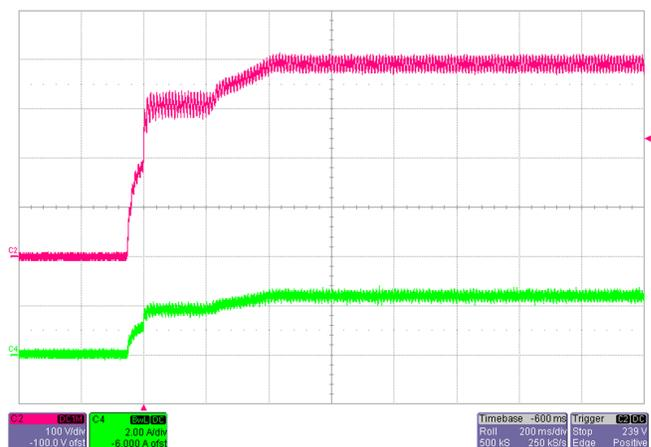
Figure 20. Output Turn-on Waveform at  $V_{INAC} = 230\text{ V}$  With Full Load of 2.56 A
