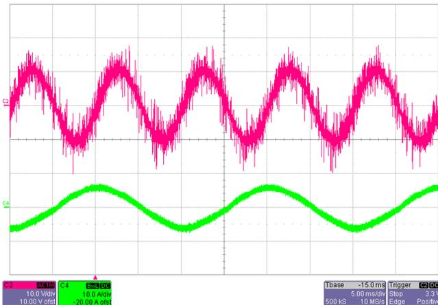
Figure 17. Output Voltage Ripple at  $V_{INAC} = 230\text{ V}$ , Full Load
