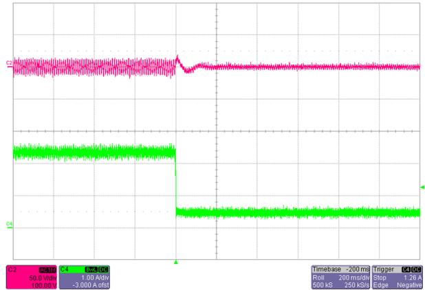
**Figure 22. Output Voltage Waveform at  $V_{INAC} = 230\text{ V}$ , Load Transient From 2.56 to 0.5 A**
