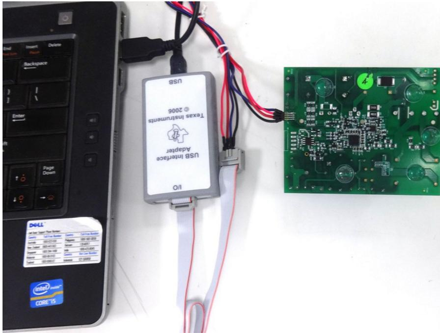
**Figure 5. TIDA-00707 Setup for Programming UCD3138A**
