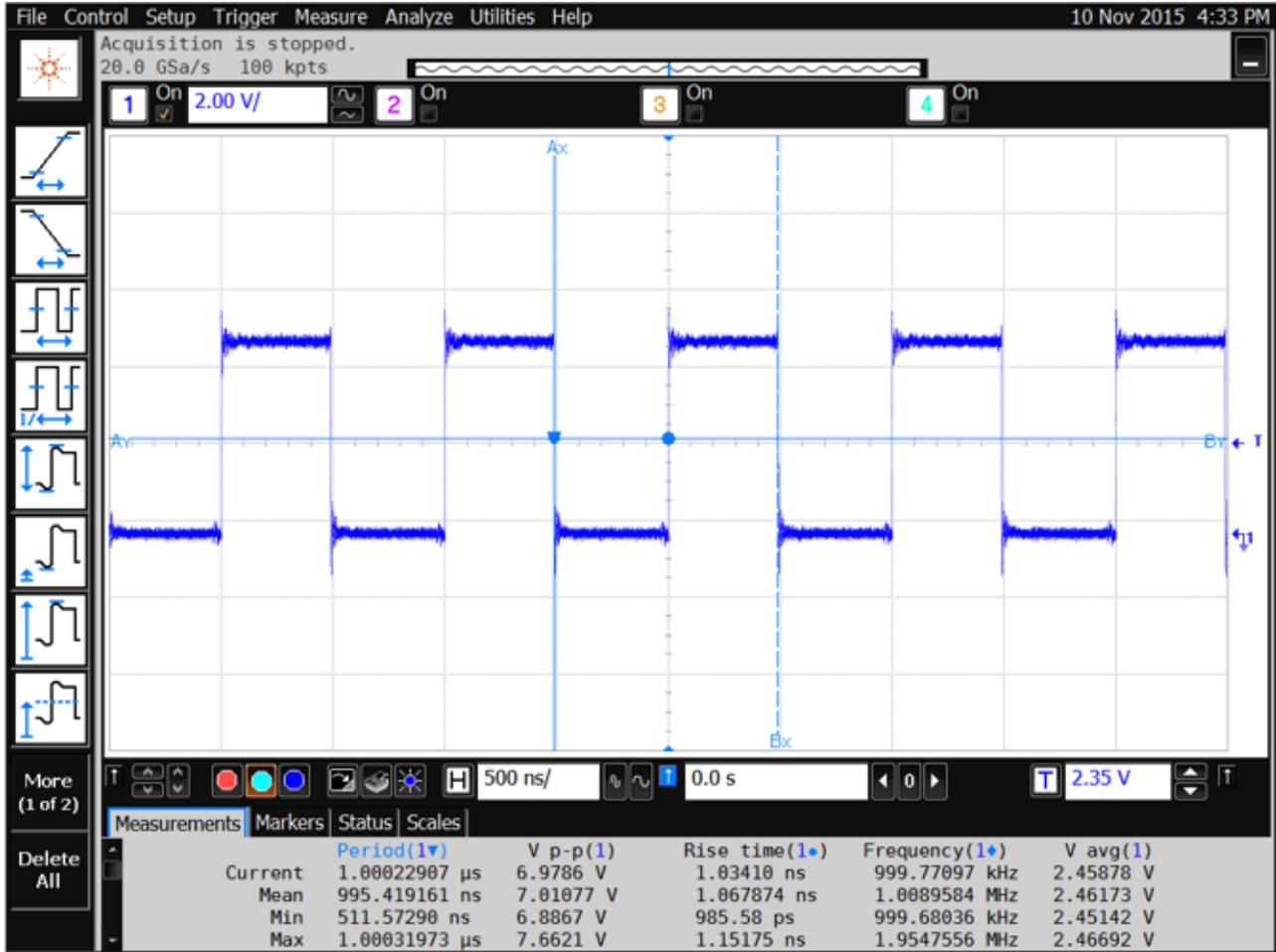
Figure 14. GaN Driver Output With 1-MHz Input
