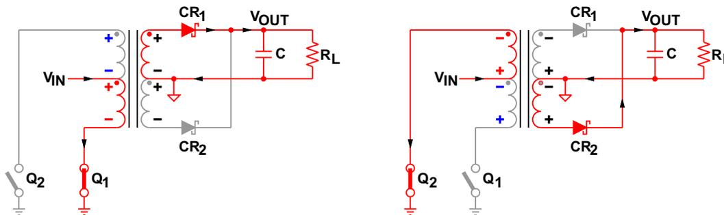
Figure 3. Push-Pull Converter Theory of Operation
