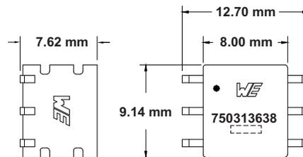
Figure 9. Transformer Dimensions in mm
