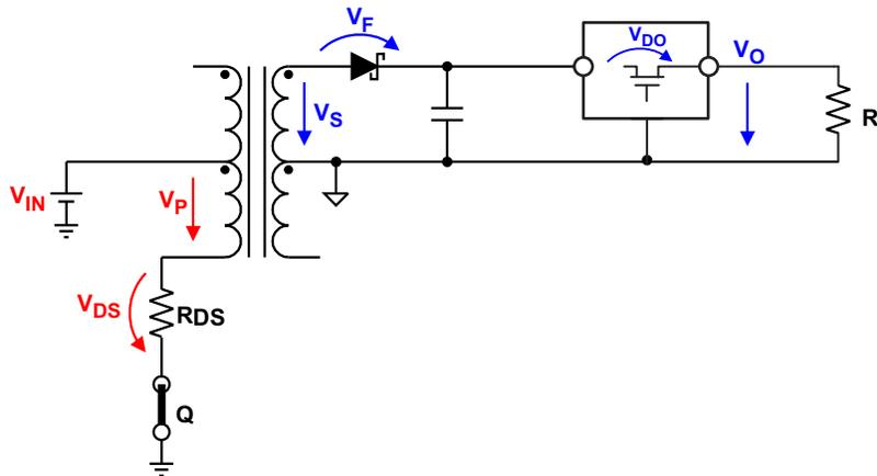
Figure 7. Establishing the Required Minimum Turns Ratio Through  $n_{min} = 1.031 \times V_{S\_min} / V_{P\_min}$
