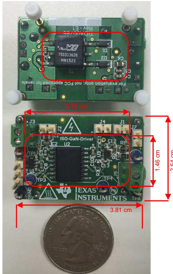
Figure 11. Complete PCB Board Size and Solution Size
