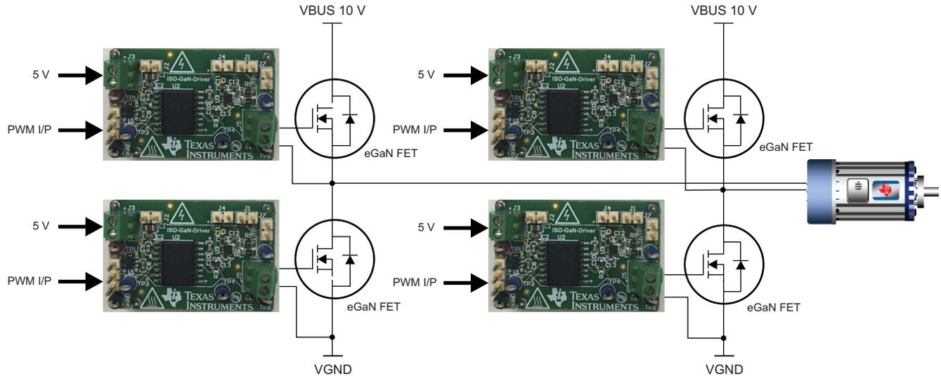
Figure 13. Test Setup
