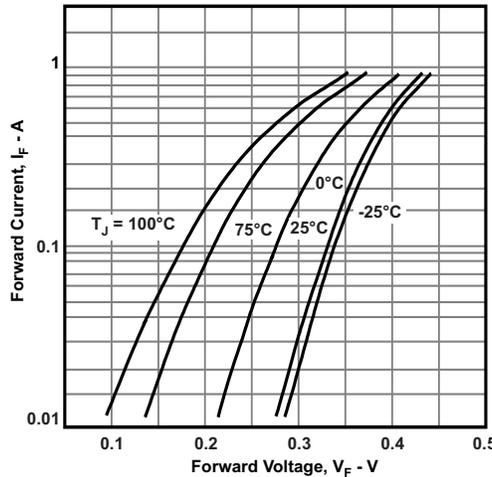
Figure 6. Diode Forward Characteristics for MBR0520L
