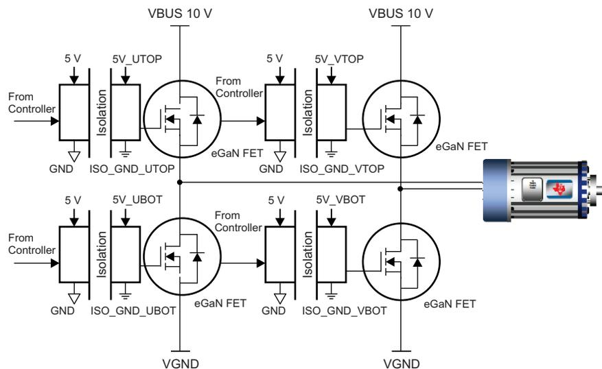
**Figure 1. TIDA-00785 System Block Diagram**
