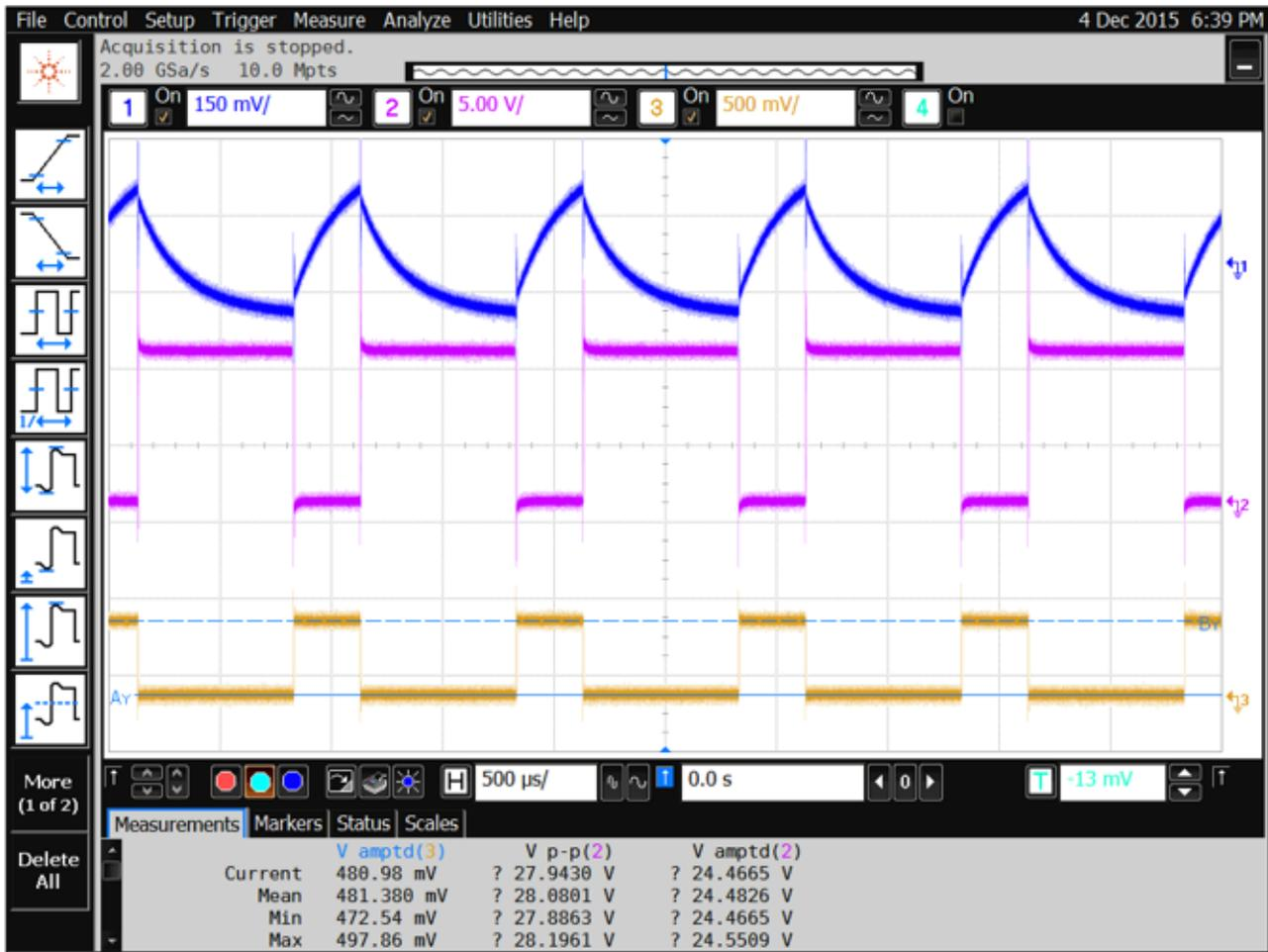
Figure 17. H-Bridge Configuration With 70% Duty Cycle Input
