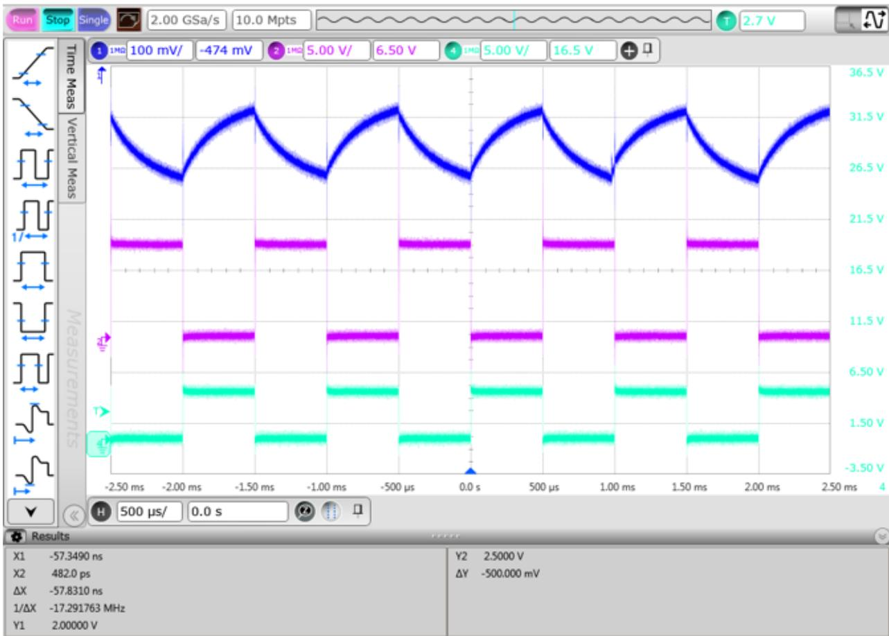
Figure 15. Half-Bridge Configuration With PWM Signal 1 kHz at 50% Duty Cycle
