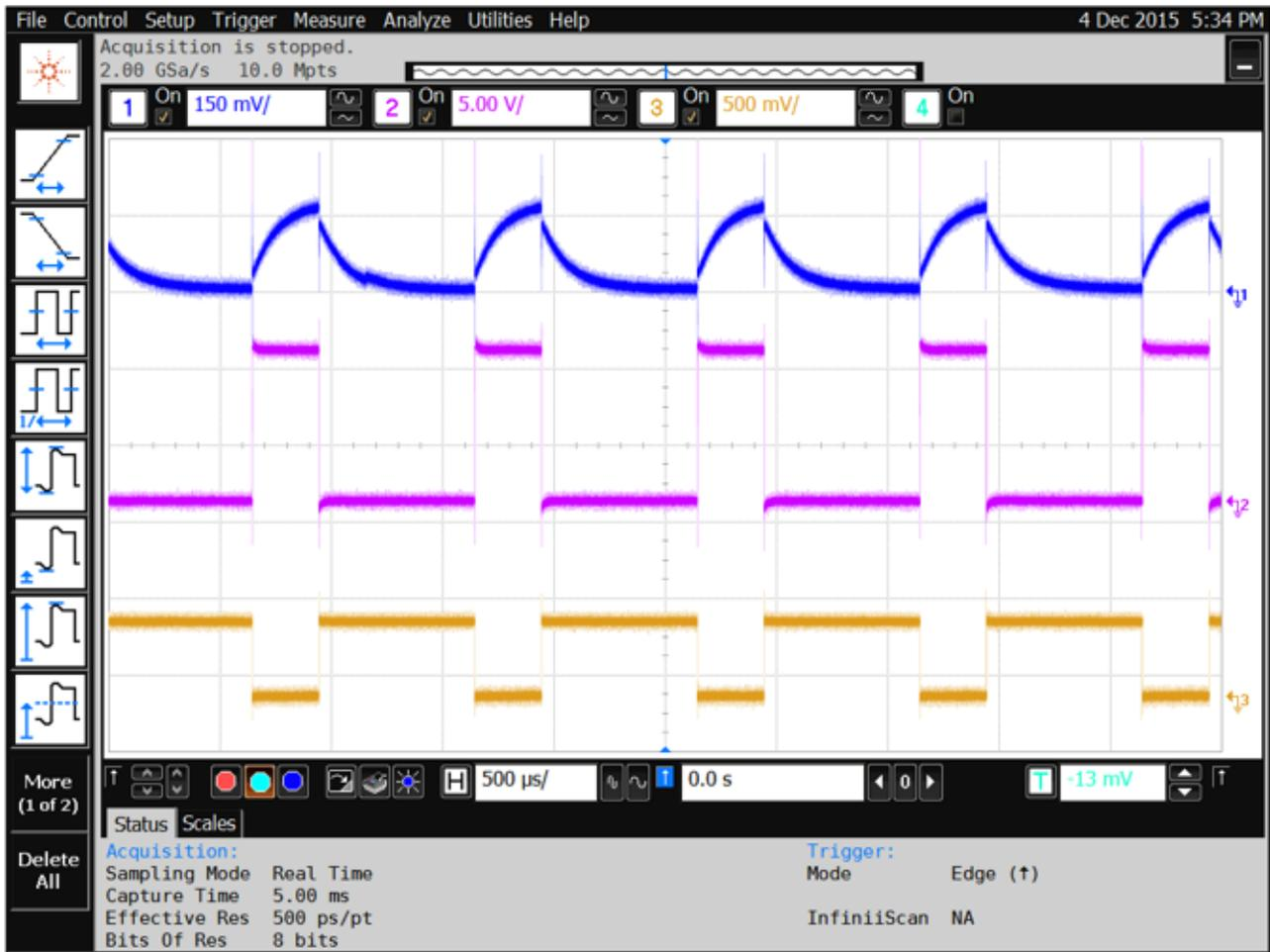
Figure 16. H-Bridge Configuration With 30% Duty Cycle Input
