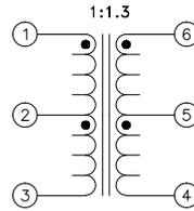
Figure 8. Push-Pull Transformer - 750313638 (Würth Electronics)
