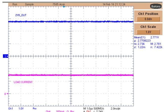
Figure 63. TPS71728-Q1 2.8-V Rail With 150-mA Load
