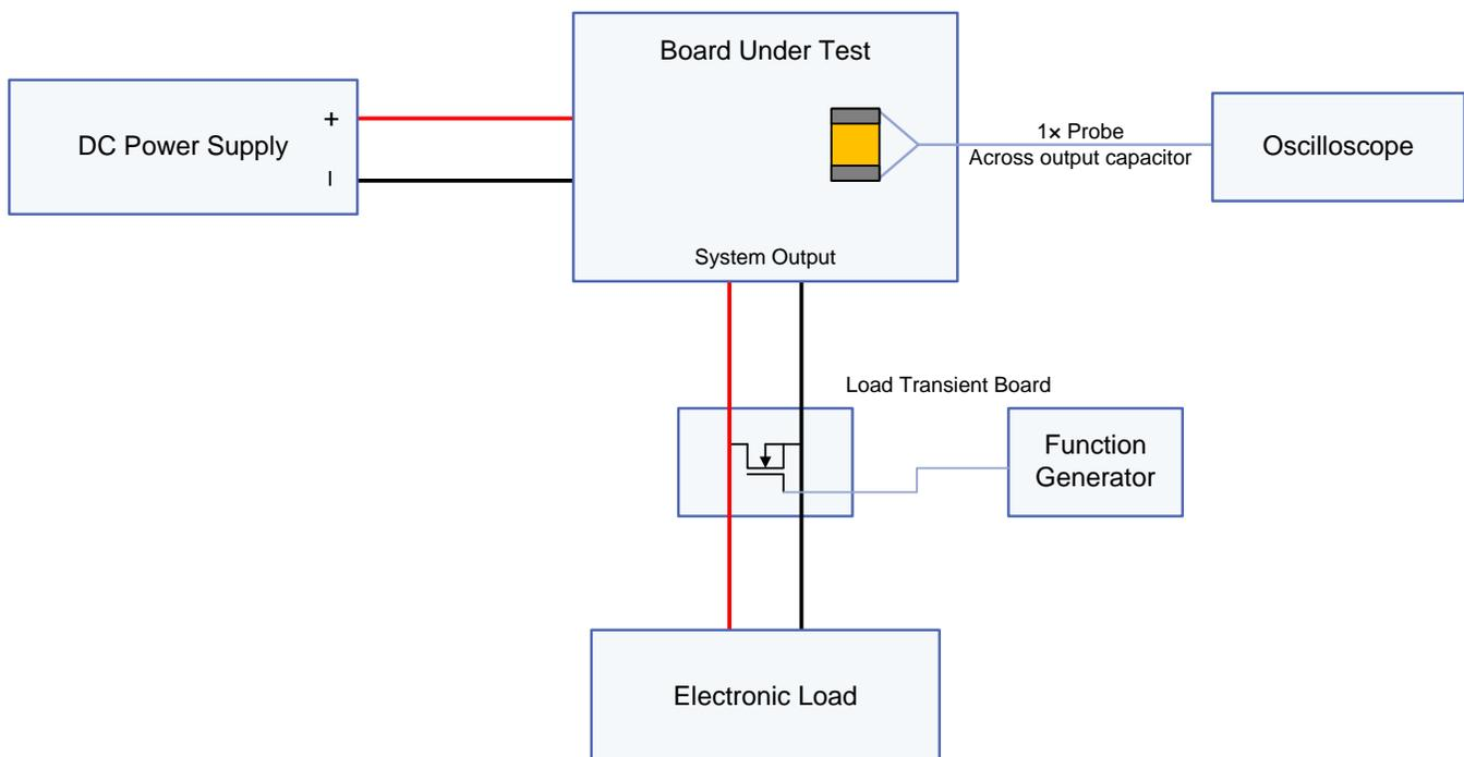
**Figure 31. Setup for Measuring Load Transients on Voltage Rails**
