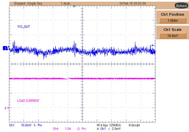
Figure 48. TPS57114-Q1 1.2-V Rail Ripple Voltage With 2-A Load
