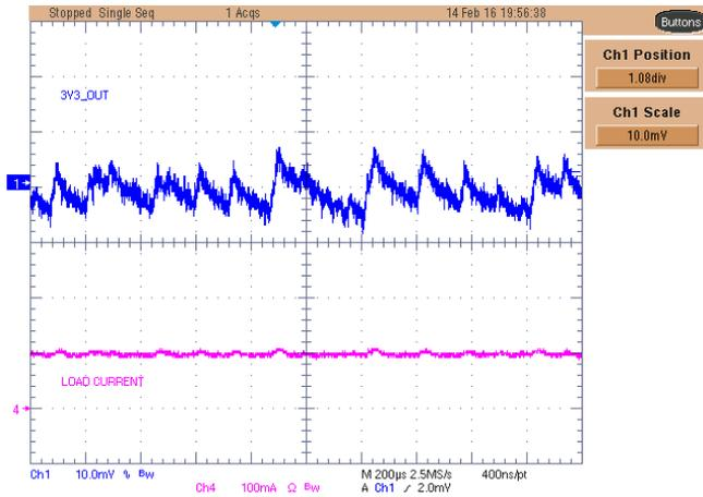
Figure 35. TPS54362-Q1 3.3V-Main Rail Ripple Voltage With 100-mA Load
