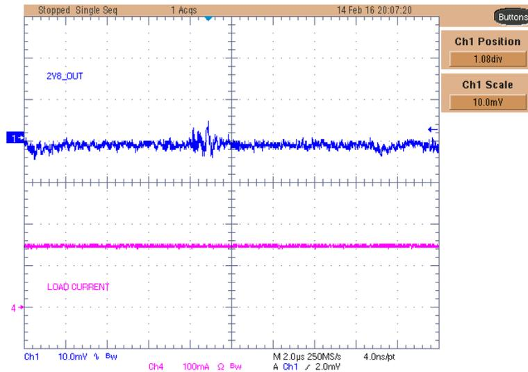
Figure 64. TPS71728-Q1 2.8-V Rail Ripple Voltage With 150-mA Load
