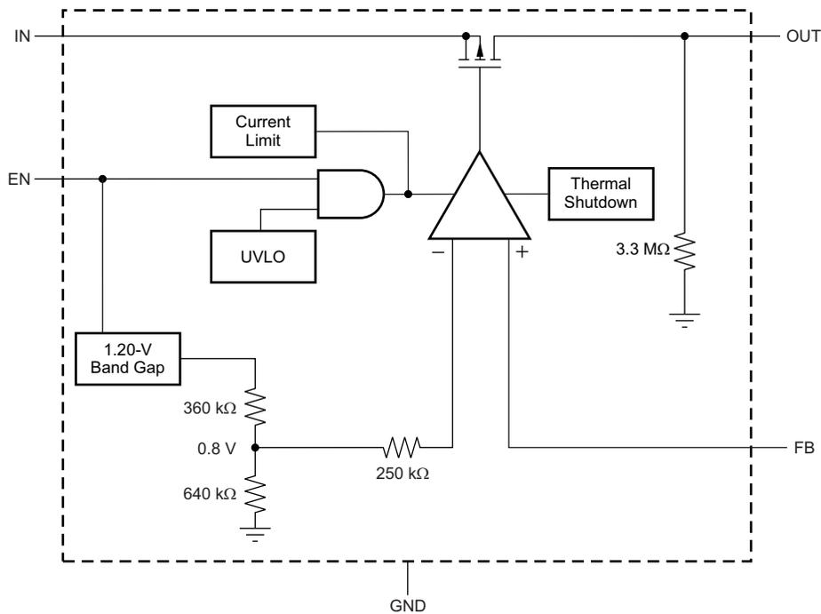
**Figure 16. Adjustable Voltage Version Block Diagram**
