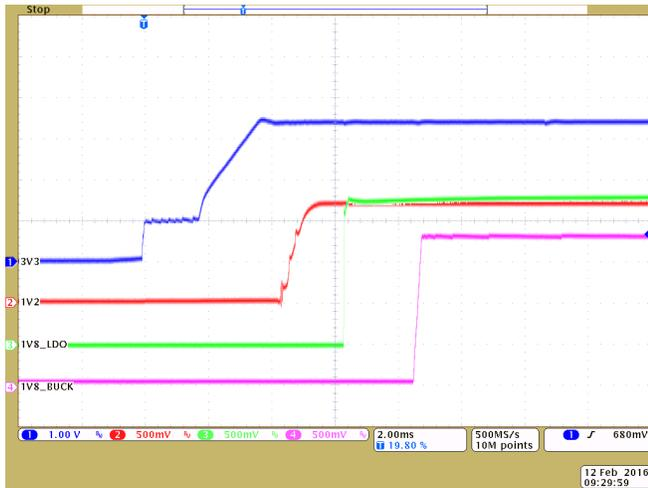
Ignition Switch is ON when VIN applied
