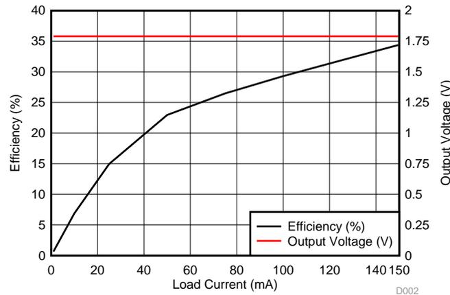
Figure 61. Efficiency of TPS71718-Q1 1V8\_LDO Rail
