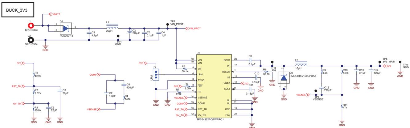
Figure 20. Wide- $V_{IN}$  Buck Pre-Regulator Schematic
