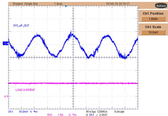
**Figure 72. TPS22966-Q1 3V3\_uP Rail Ripple Voltage with 1-A Load**
