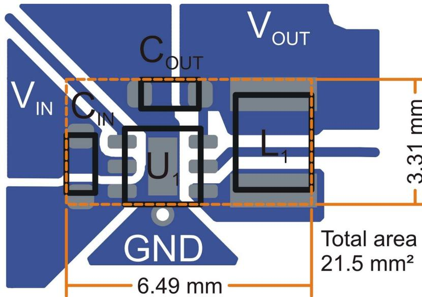
Figure 88. Suggested Layout for Fixed Output Voltage Options
