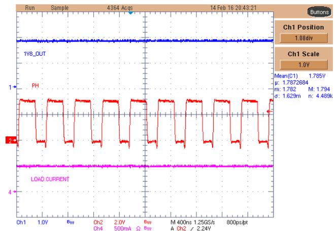
Figure 40. TPS62261-Q1 1V8\_BUCK Rail With 500-mA Load
