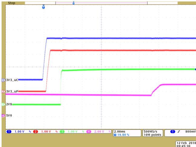
NOTE: Because 5V0 is a Boost regulator rail, the 5V0 is already 3.3 V before becoming enabled and rising to 5.0 V
