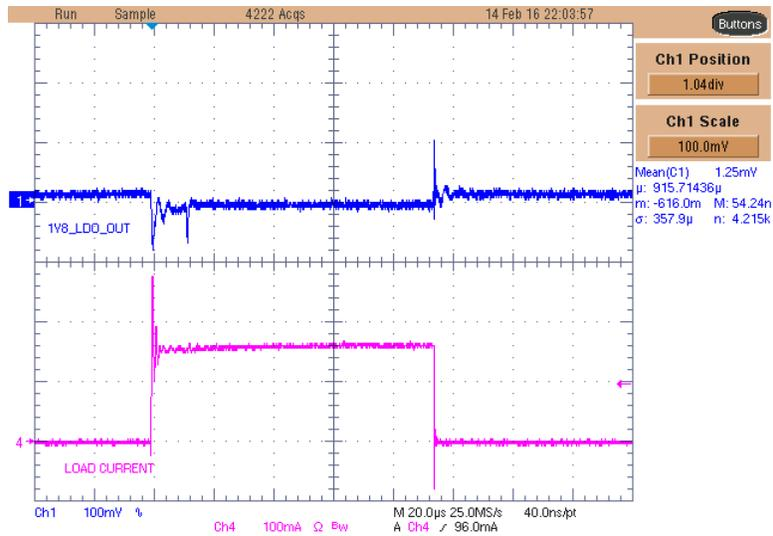
Figure 60. TPS71718-Q1 1V8\_LDO Rail Voltage With 150-mA Load Transient
