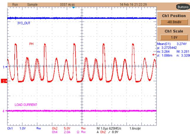
Figure 33. TPS54362-Q1 3.3-V Main Rail With No Load
