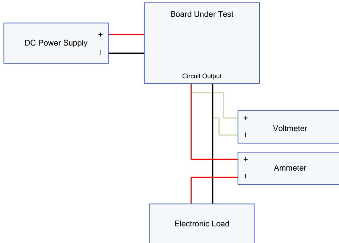
Figure 32. Setup for Measuring System Efficiency of Voltage Rails
