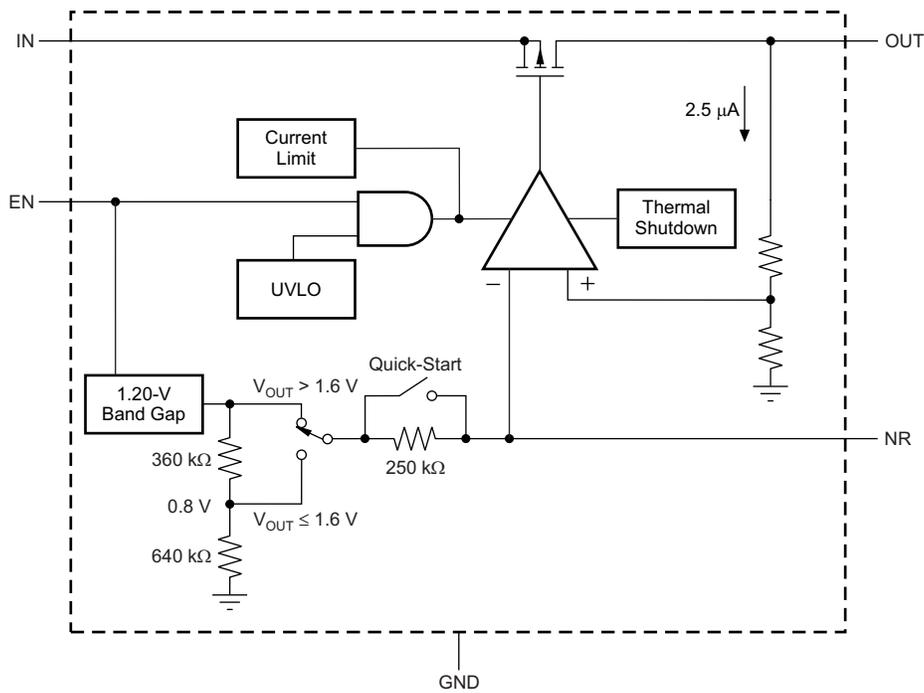
**Figure 15. Fixed Voltage Versions Block Diagram**
