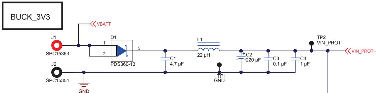
Figure 19. Input Protection and EMI and EMC Input Filter Schematic
