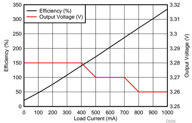
Figure 76. Efficiency of TPS22966-Q1 3V3\_uP Rails
