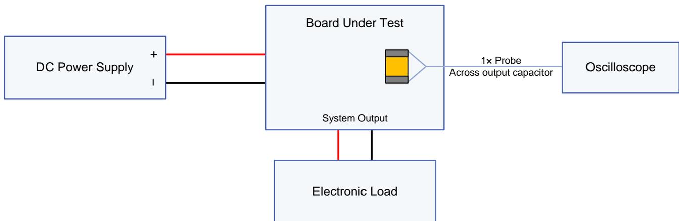
**Figure 30. Setup for Measuring Output Ripple Voltage of Voltage Rails**
