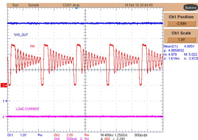
Figure 51. TPS61170-Q1 5.0-V Rail With No Load
