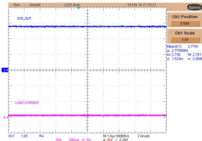
Figure 62. TPS71728-Q1 2.8-V Rail With No Load
