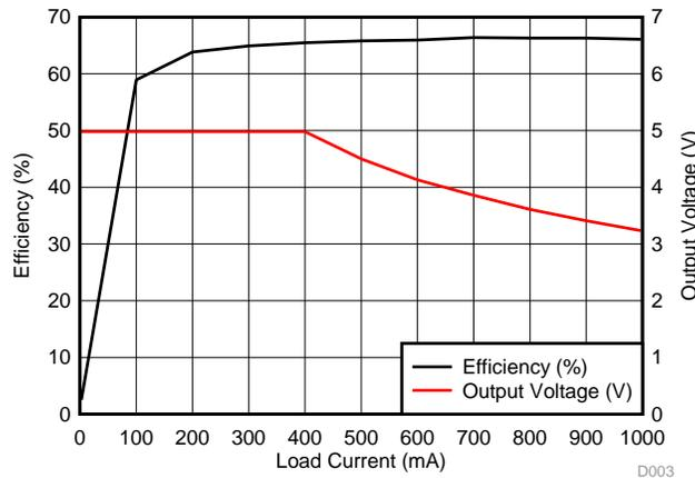
Figure 56. Efficiency of TPS61170-Q1 5.0-V Rail
