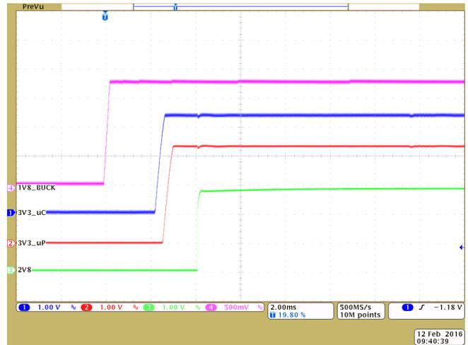
**Figure 78. Startup Behavior of 1V8\_BUCK, 3V3\_uC, 3V3\_uP, and 2V8 Rails**
