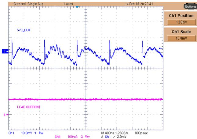
Figure 53. TPS61170-Q1 5.0-V Rail Ripple Voltage With 100-mA Load
