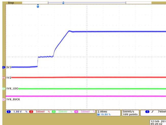
Figure 81. Startup Behavior of Main 3V3 Rail With Ignition Switch OFF
