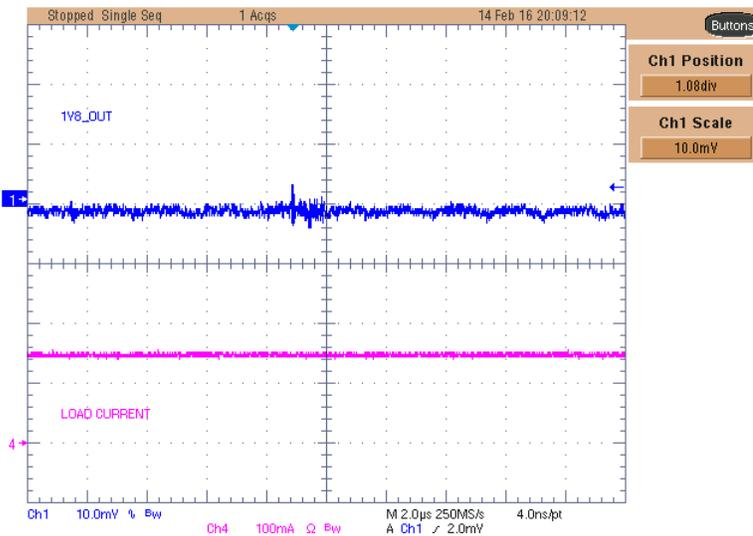
Figure 59. TPS71718-Q1 1V8\_LDO Rail Ripple Voltage With 150-mA Load
