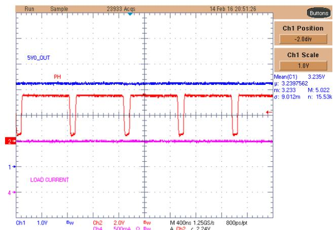
Figure 52. TPS61170-Q1 5.0-V Rail Ripple Voltage With 1-A Load
