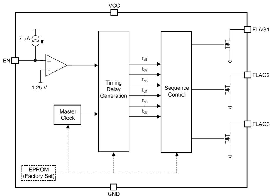
**Figure 9. LM3880-Q1 Block Diagram**
