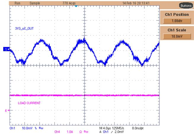
**Figure 70. TPS22966-Q1 3V3\_uC Rail Ripple Voltage With 1-A Load**
