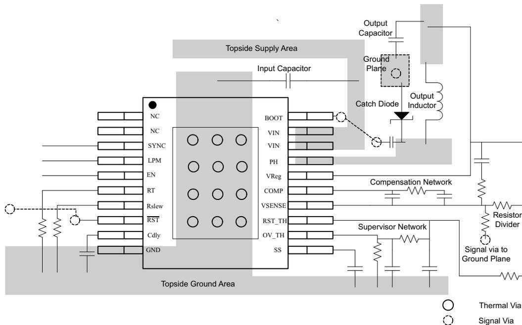
**Figure 85. TPS22966-Q1 PCB Layout Example**
