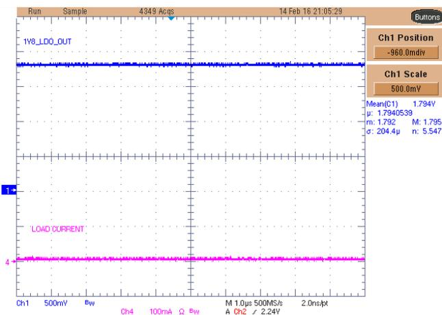
Figure 57. TPS71718-Q1 1V8\_LDO Rail With No Load
