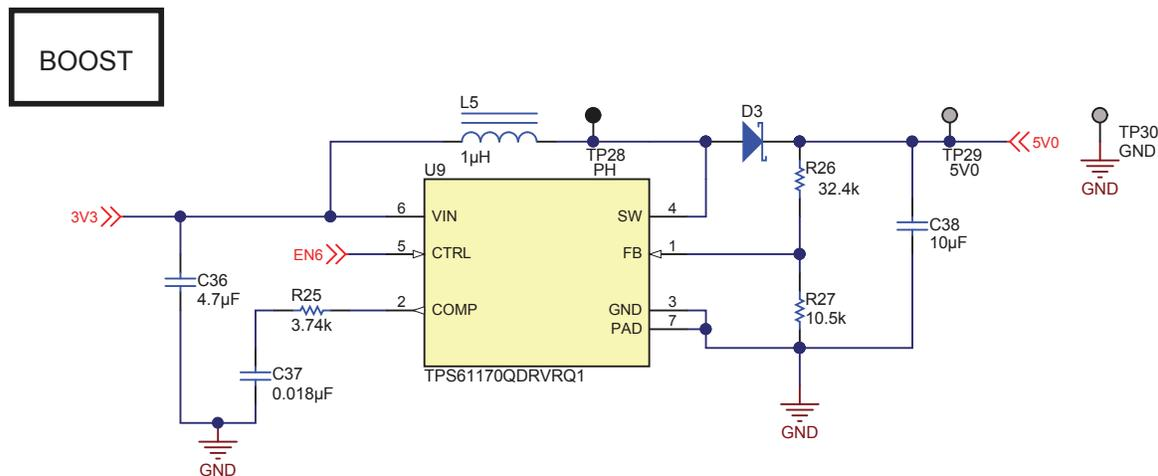
Figure 23. TPS61170-Q1 Buck Converter Schematic
