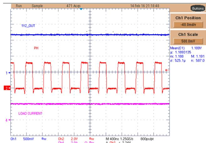
Figure 46. TPS57114-Q1 1.2-V Rail With 2-A Load
