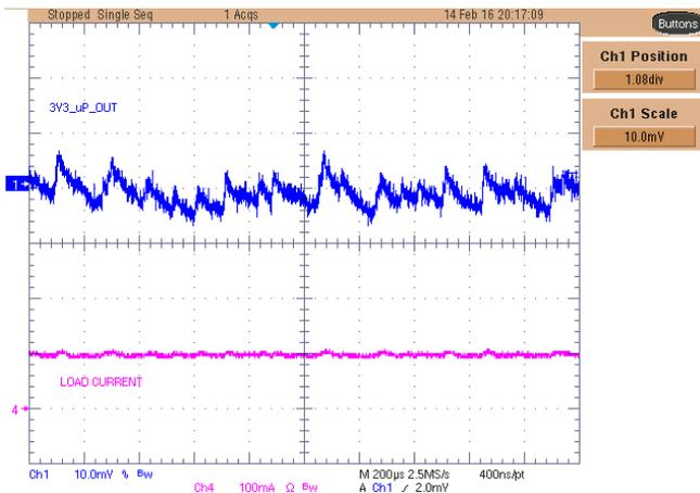
**Figure 71. TPS22966-Q1 3V3\_uP Rail Ripple Voltage With 100-mA Load**
