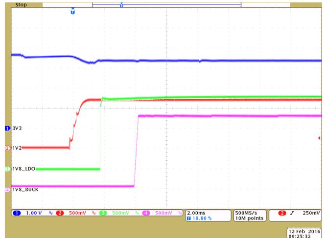
**Figure 80. Startup Behavior of 1V2, 1V8\_LDO, and 1V8\_BUCK When Activated By Ignition Switch With 3V3 Main Rail Already Powered On**
