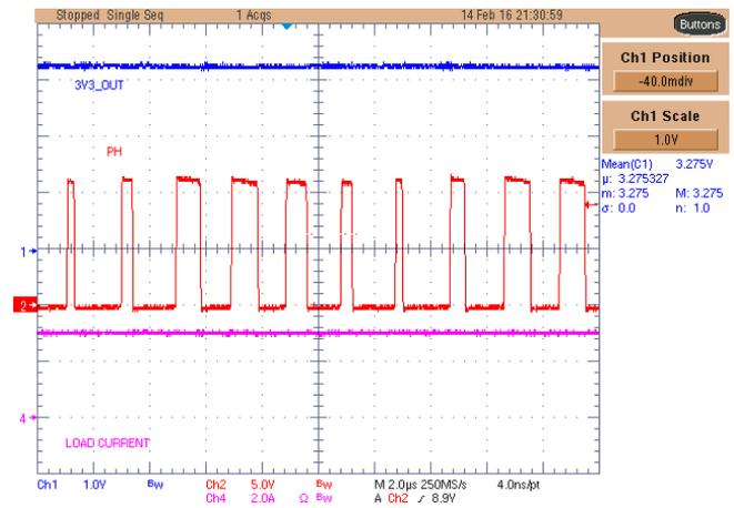
Figure 34. TPS54362-Q1 3.3-V Main Rail With 3-A Load
