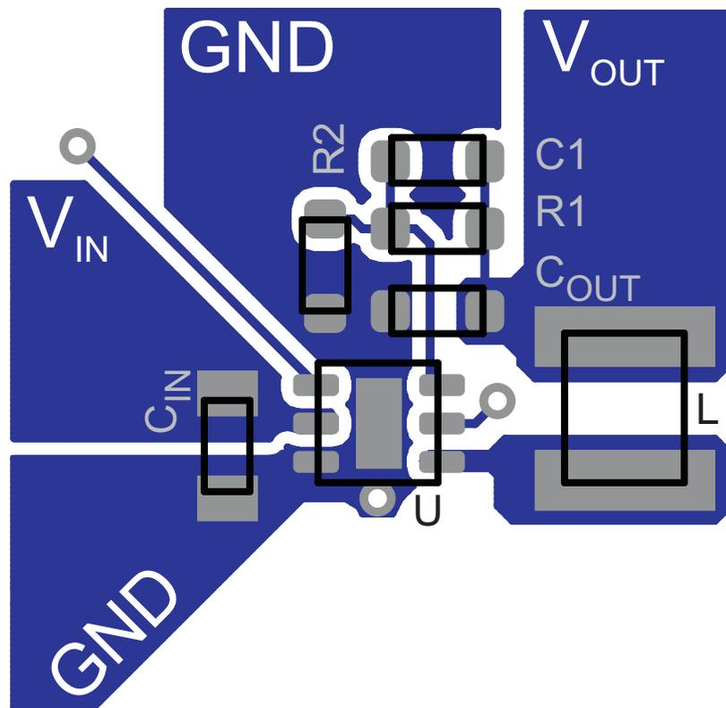
Figure 89. Suggested Layout for Adjustable Output Voltage Version
