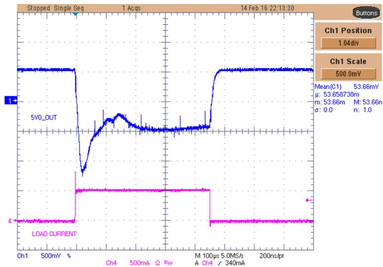
Figure 55. TPS61170-Q1 5.0-V Rail Voltage With 500-mA Load Transient
