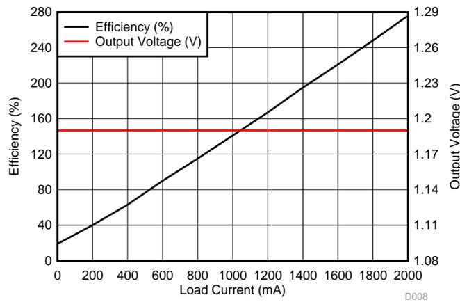
Figure 50. Efficiency of TPS57114-Q1 1.2-V Rail
