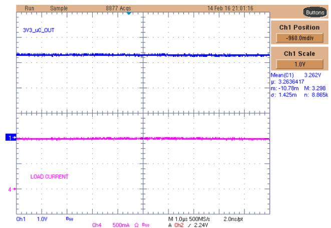
Figure 68. TPS22966-Q1 3V3\_uC Rail With 1-A Load
