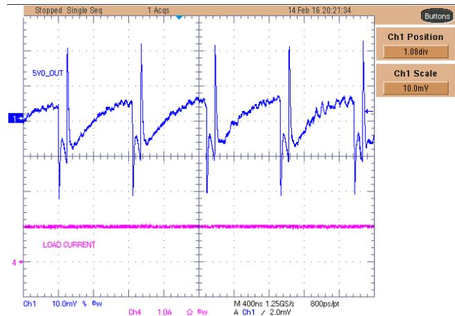
Figure 54. TPS61170-Q1 5.0-V Rail Ripple Voltage With 1-A Load
