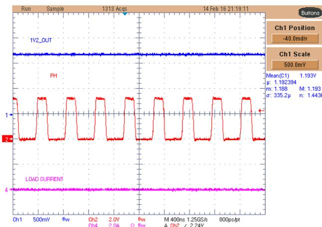
Figure 45. TPS57114-Q1 1.2-V Rail With No Load
