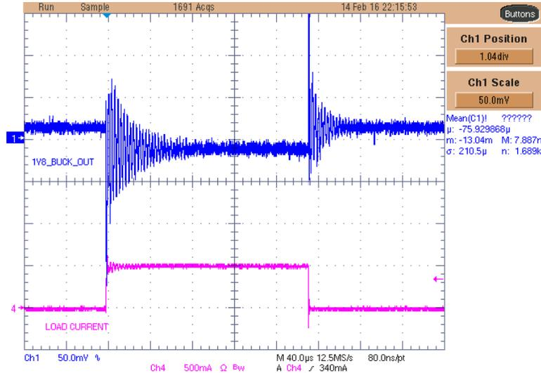
Figure 43. TPS62261-Q1 1V8\_BUCK Rail Voltage With 500-mA Load Transient
