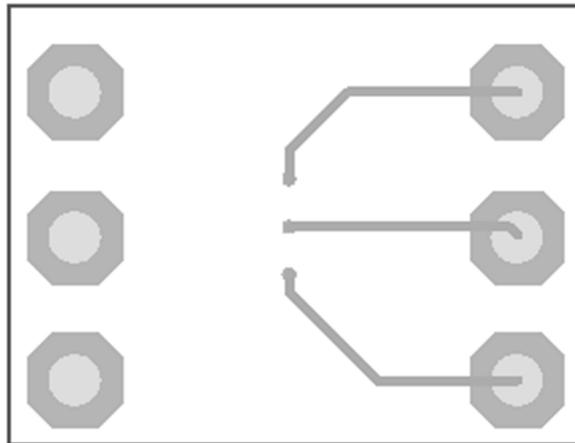
**Figure 83. LM3880-Q1 Bottom**
