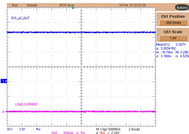
Figure 67. TPS22966-Q1 3V3\_uC Rail With No Load
