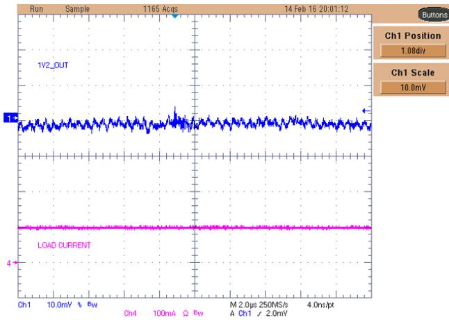
Figure 47. TPS57114-Q1 1.2-V Rail Ripple Voltage With 100-mA Load
