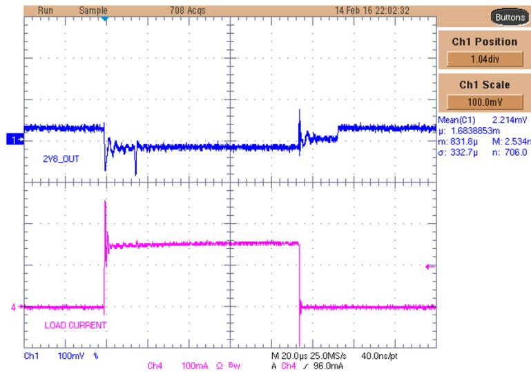
Figure 65. TPS71728-Q1 2.8-V Rail Voltage With 150-mA Load Transient
