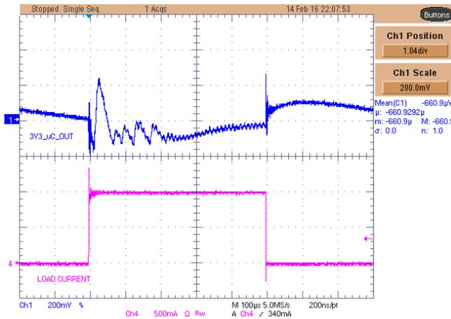
Figure 73. TPS22966-Q1 3V3\_uC Rail Voltage With 1-A Load Transient
