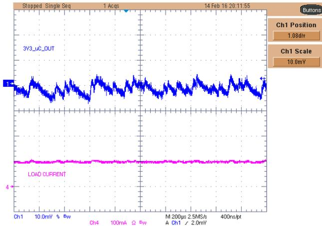
**Figure 69. TPS22966-Q1 3V3\_uC Rail Ripple Voltage With 100-mA Load**
