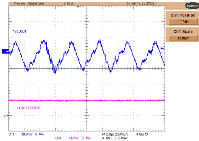
Figure 41. TPS62261-Q1 1V8\_BUCK Rail Ripple Voltage With 100-mA Load
