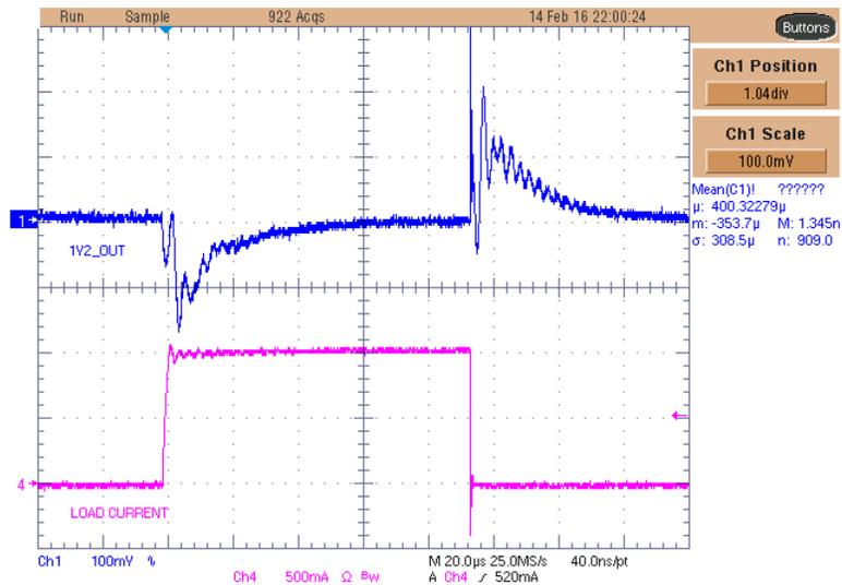
Figure 49. TPS57114-Q1 1.2-V Rail Voltage With 2-A Load Transient
