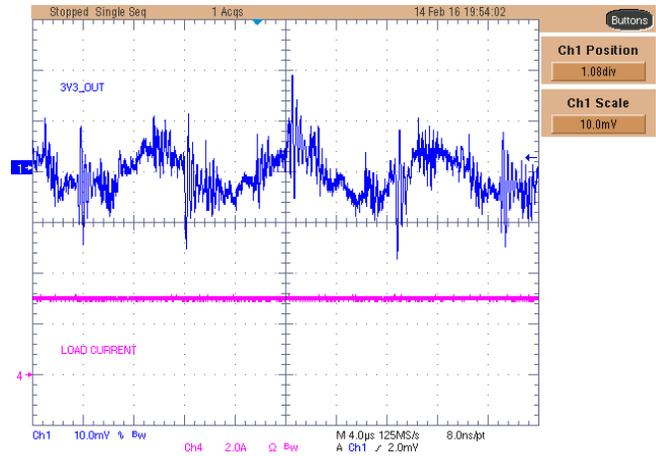
Figure 36. TPS54362-Q1 3.3V-Main Rail Ripple Voltage With 3-A Load
