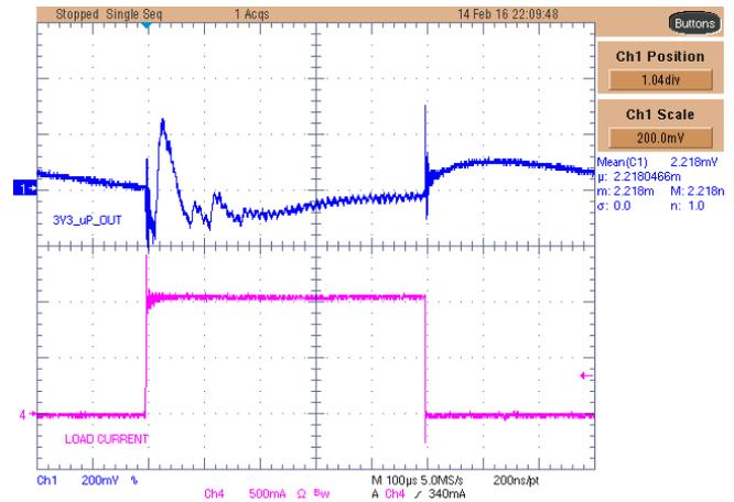
Figure 74. TPS22966-Q1 3V3\_uP Rail Voltage With 1-A Load Transient
