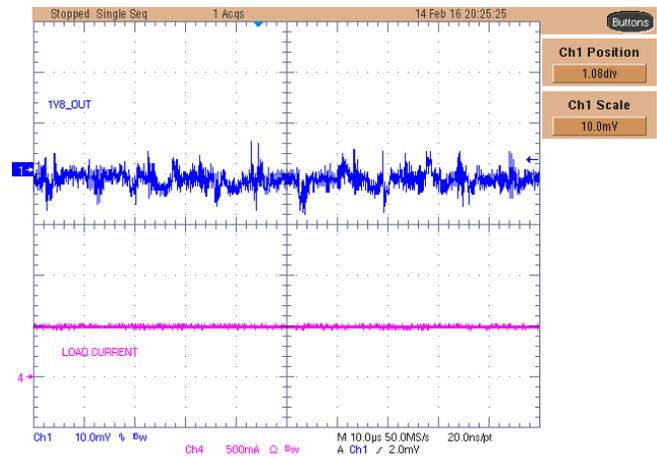
Figure 42. TPS62261-Q1 1V8\_BUCK Rail Ripple Voltage With 500-mA Load
