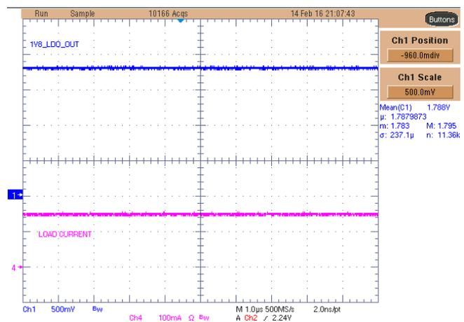
Figure 58. TPS71718-Q1 1V8\_LDO Rail With 150-mA Load
