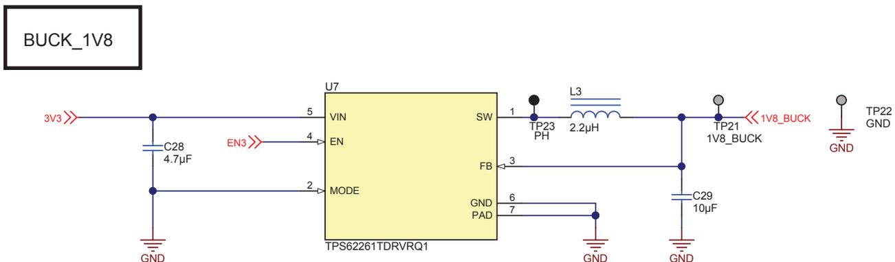
Figure 21. TPS62261-Q1 Buck Converter Schematic
