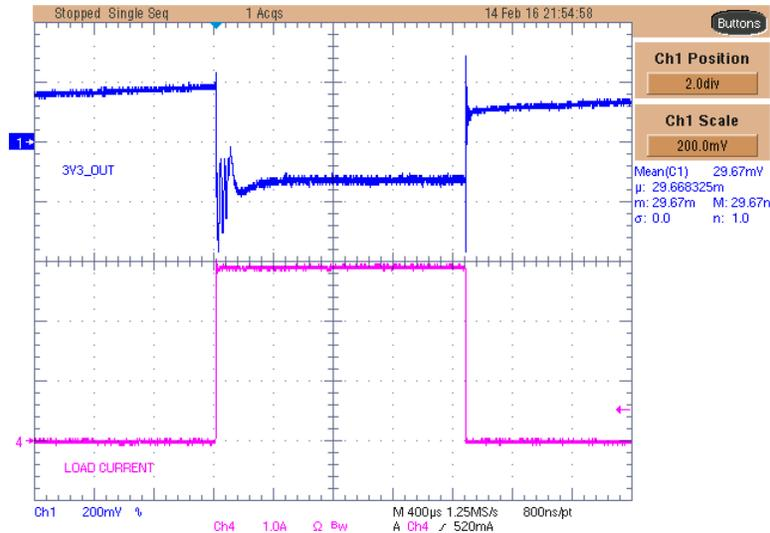
Figure 37. TPS54362-Q1 3.3-V Main Rail Voltage With 3-A Load Transient
