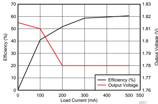
Figure 44. Efficiency of TPS62261-Q1 1V8\_BUCK Rail
