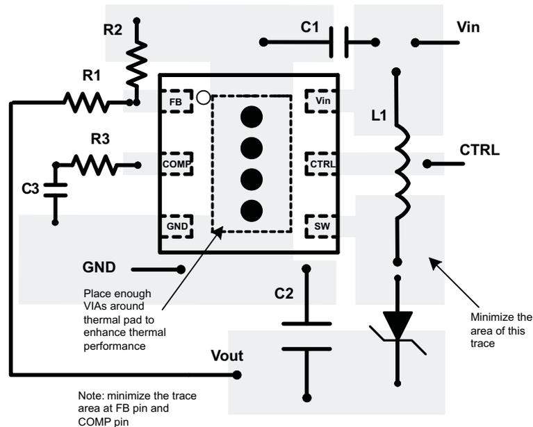
Figure 87. TPS61170-Q1 PCB Layout Recommendation
