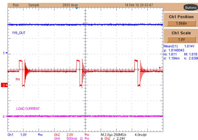
Figure 39. TPS62261-Q1 1V8\_BUCK Rail With No Load
