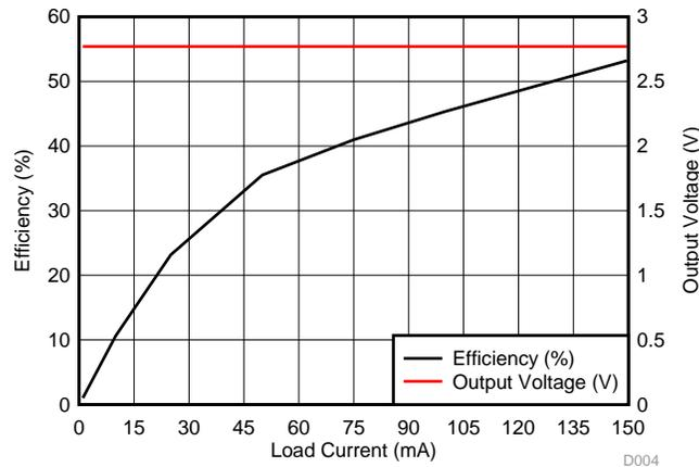
Figure 66. Efficiency of TPS71728-Q1 2.8-V Rail
