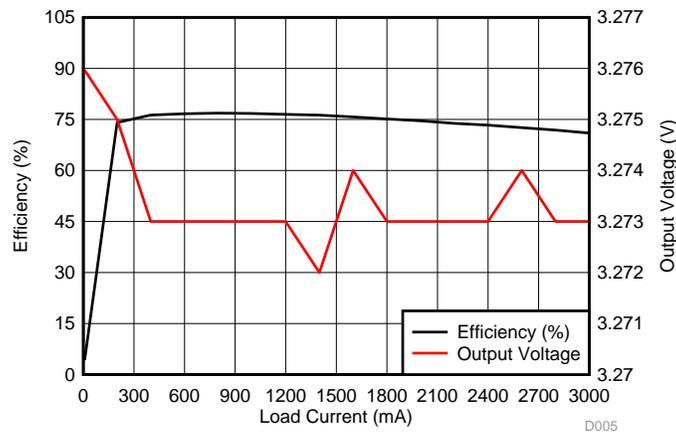
Figure 38. Efficiency of TPS54362-Q1 Main 3.3-V Rail
