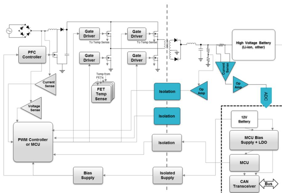
**Figure 1: Complete Analog On-Board Charger System**
