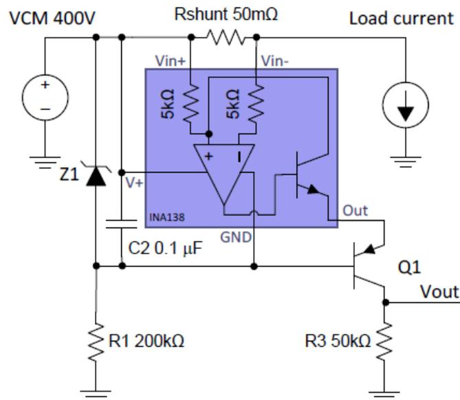
**Figure 3: Schematic of INA138-Q1 in a High Common Mode Voltage Application**
