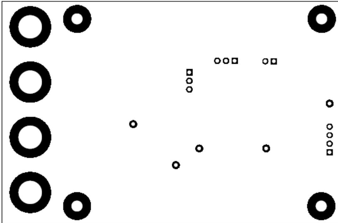
Figure 20: Bottom Solder Mask
