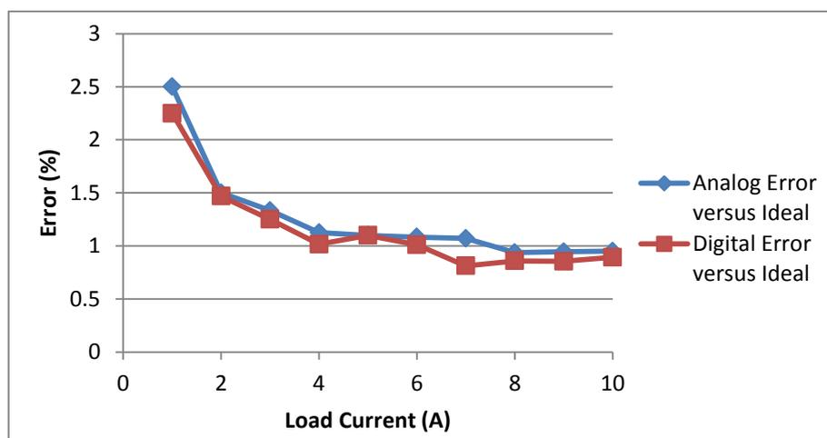
**Figure 8: Analog and Digital Error vs Load Current, Battery Voltage = 160V**
