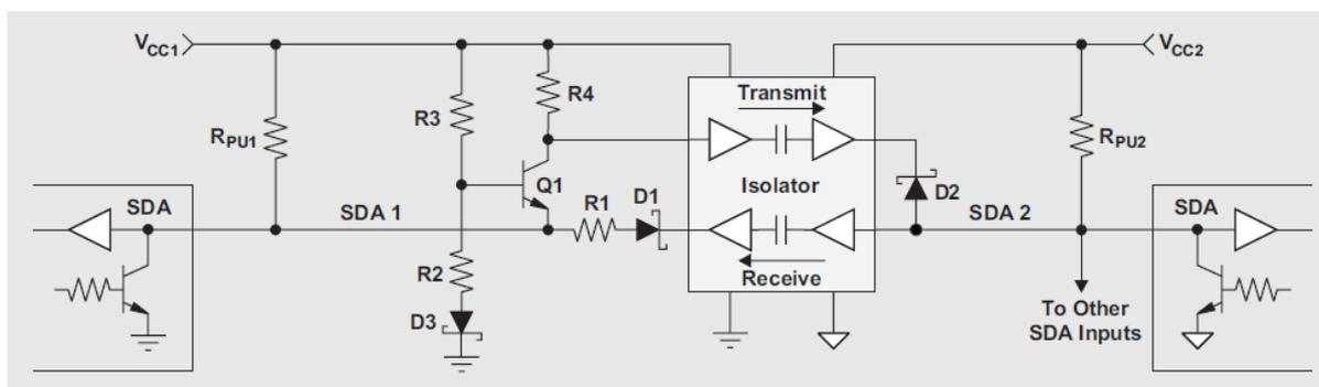
**Figure 5: Bidirectional Communication with Digital Isolator**
