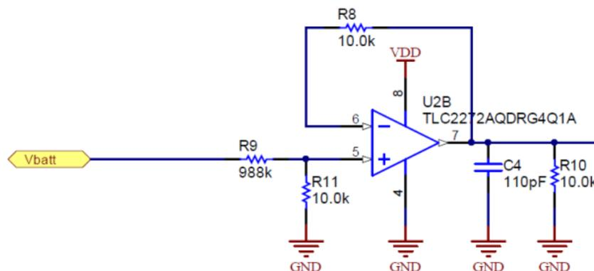
Figure 4: Battery Voltage Measurement Circuit
