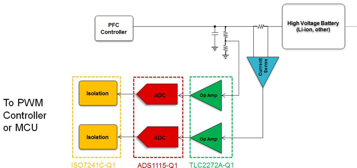
Figure 2: On-Board Charger Load Feedback Subsystem
