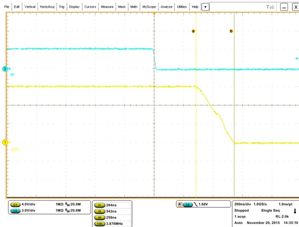
Figure 4: Falling Slew Rate (258 ns)
