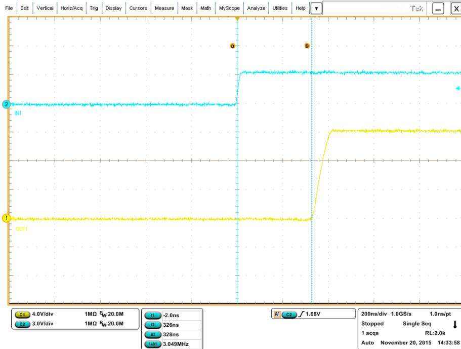
Figure 1: Rising Propagation Delay (328 ns)
