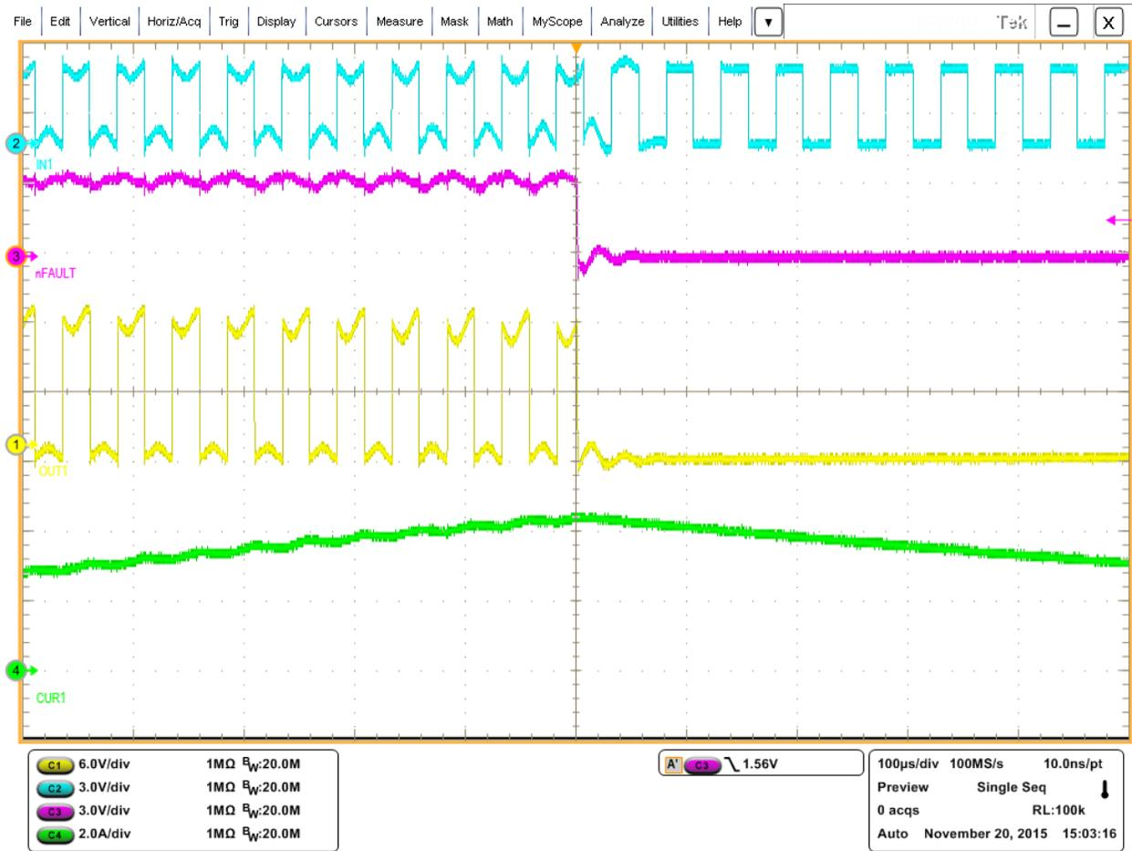
Figure 7: DRV8313 Overcurrent Protection
