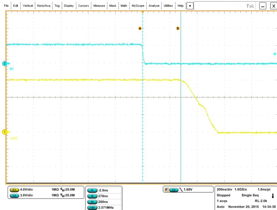
Figure 2: Falling Propagation Delay (280 ns)
