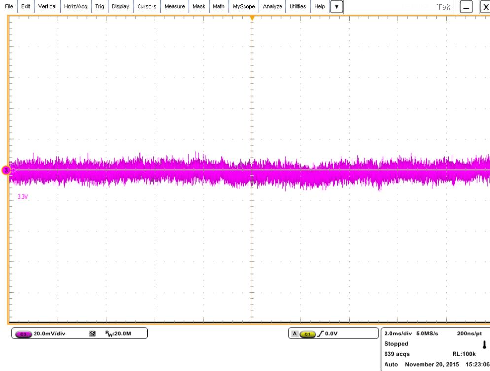
**Figure 8: 3.3 V Output Ripple (+/- 10 mV)**
