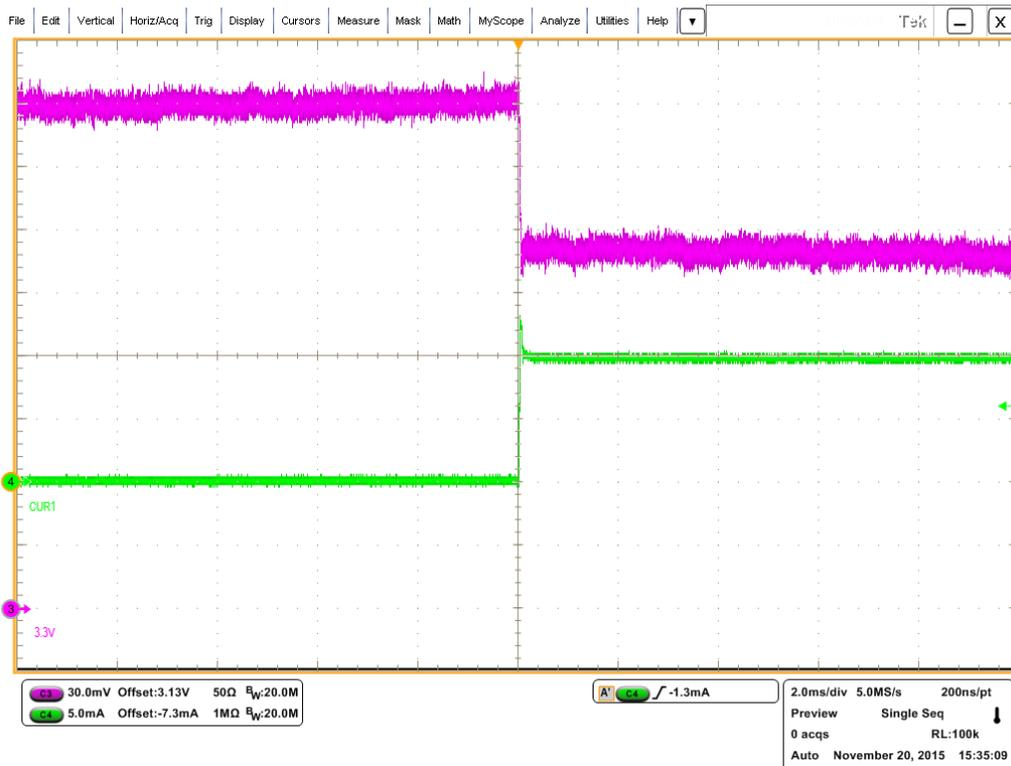
**Figure 9: 3.3 V Load Response (10 mA Step)**
