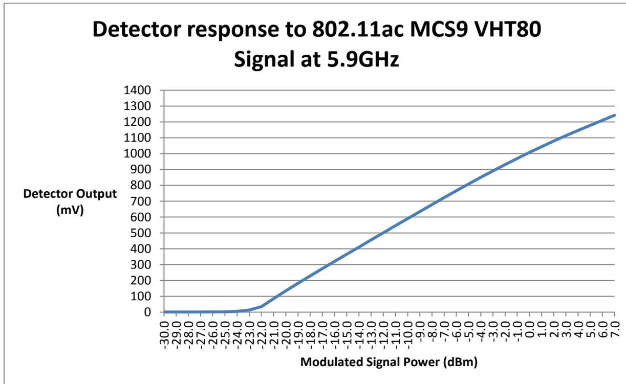
Figure 11: Detector Response at 5.9GHz
