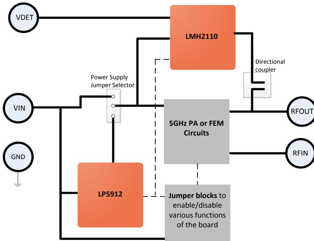
Figure 1 TIDA-00897 Design High Level Block Diagram
