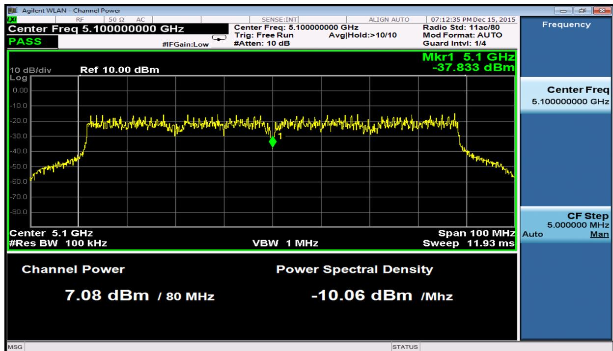
Figure8: 802.11ac Signal 5.1GHz
