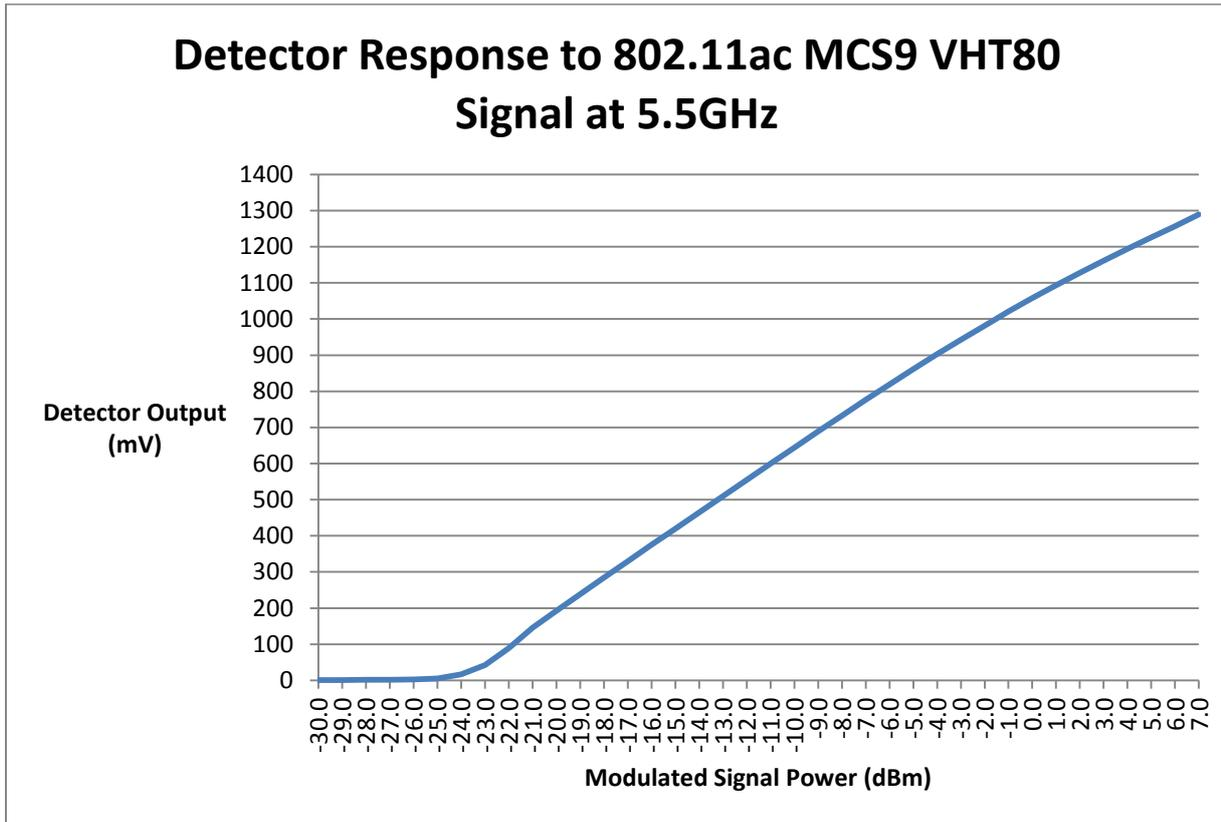
Figure 9: Detector Response at 5.5GHz
