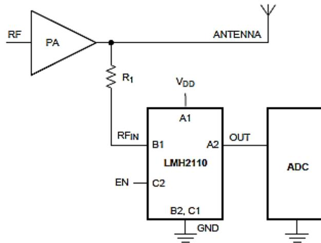
**Figure 5 Application schematic**
