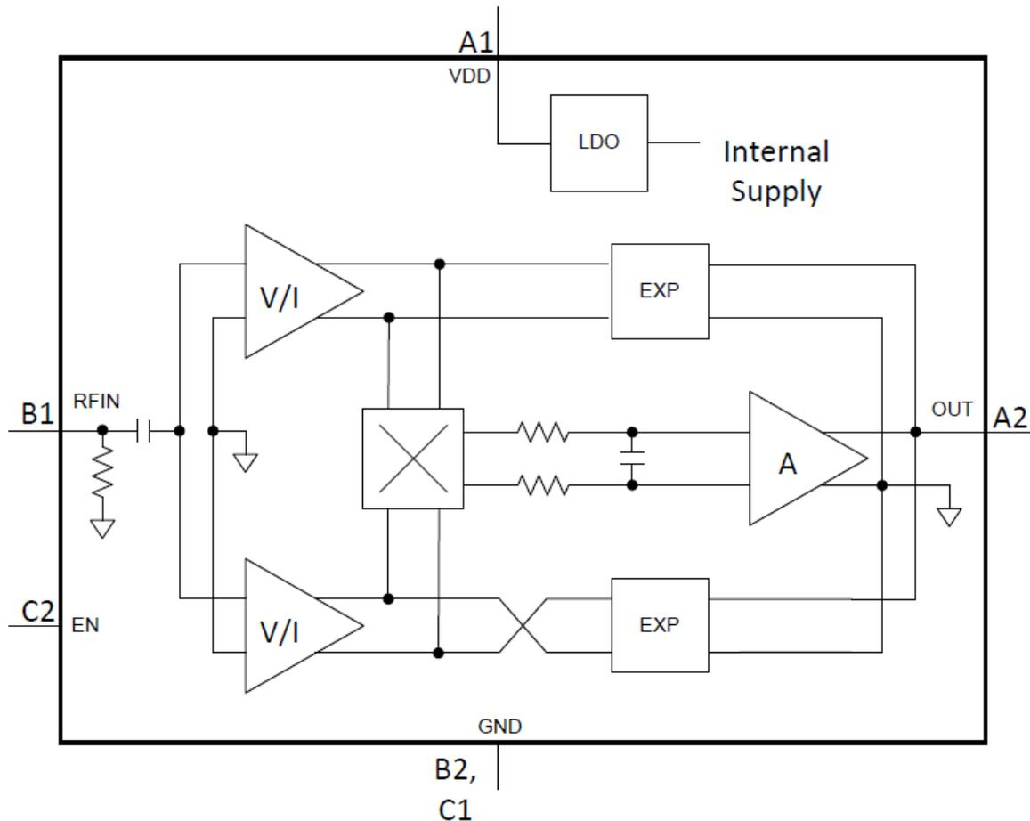
Figure 2 LMH2110 Functional Block Diagram
