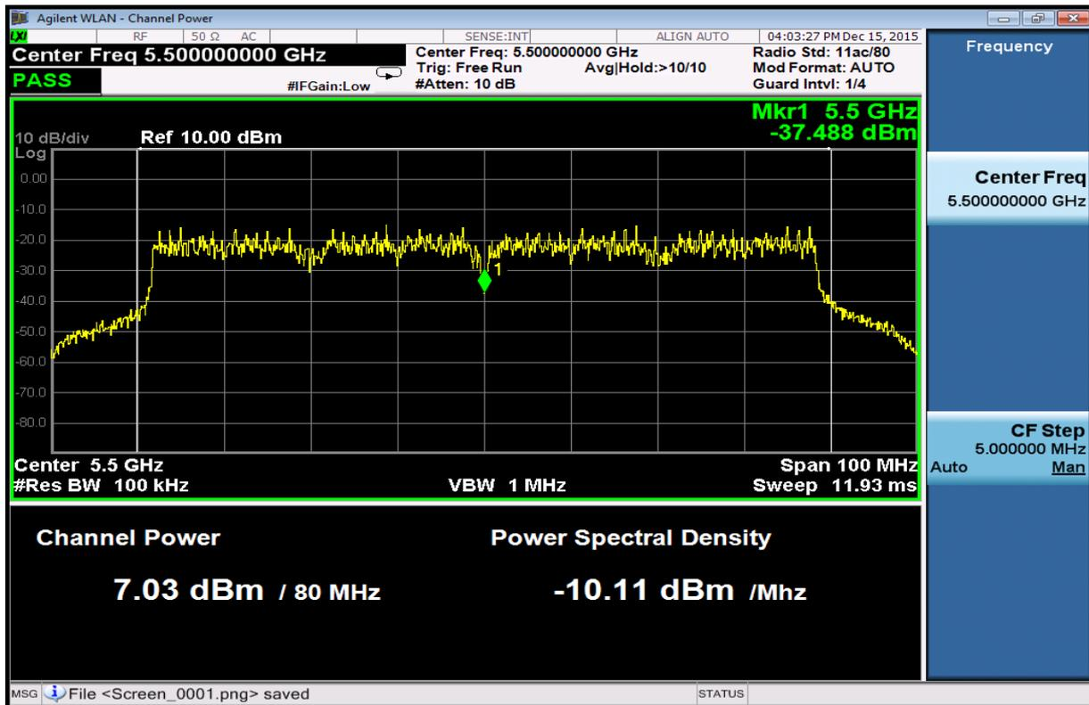
Figure 10: 802.11ac Signal 5.5GHz
