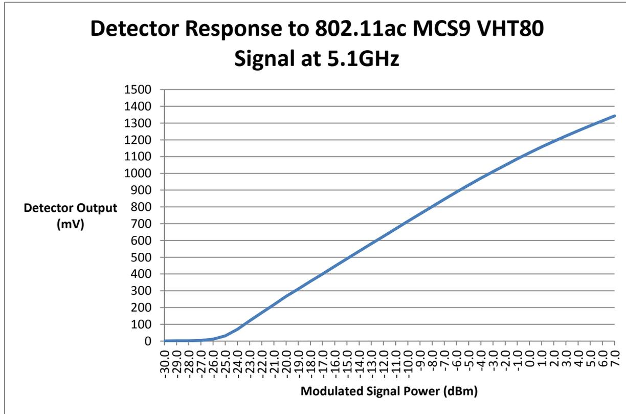
Figure 7: Detector Response at 5.1GHz
