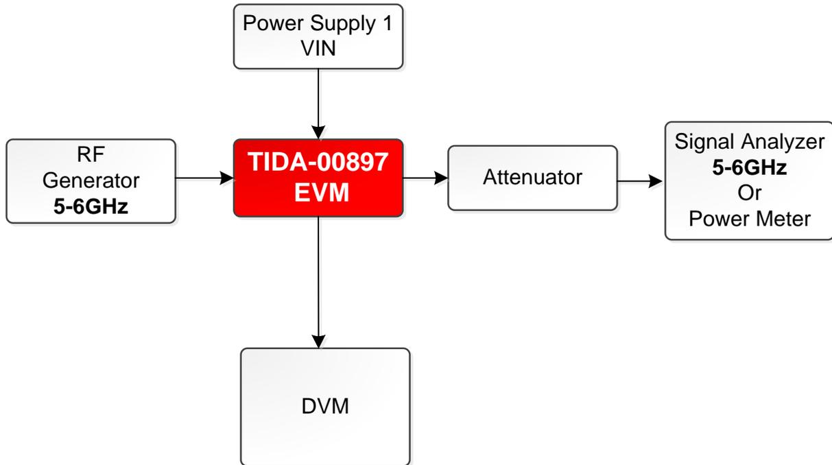
Figure 6 Test Setup Block Diagram
