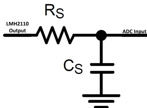
Figure 4: Optional filter configuration at output of LMH2110
