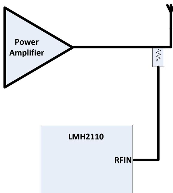
Figure 15: Coupling Resistor Placement
