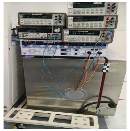
Figure 16. Test Setup for Testing Across Temperature Range
