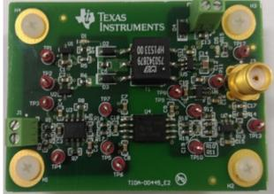
Shunt-Based 200-A Peak Current Measurement Reference Design Using
