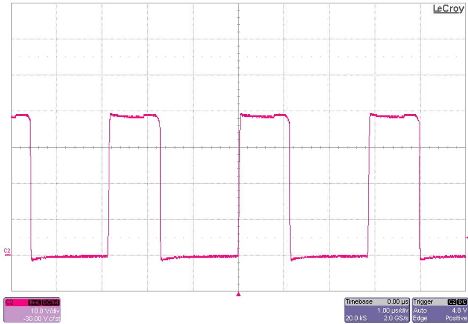
The photo below shows the FET switching voltage. The input voltage is 28V and the output is loaded to 0.29A. The converter is just starting DCM operation. (10V/DIV, 1uS/DIV)
