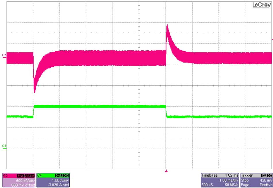
The photo below shows the output voltage (ac coupled) when the load current is stepped between 1A and 2A.  $V_{in} = 24V$ . (1V/DIV, 1A/DIV, 1mS/DIV)
