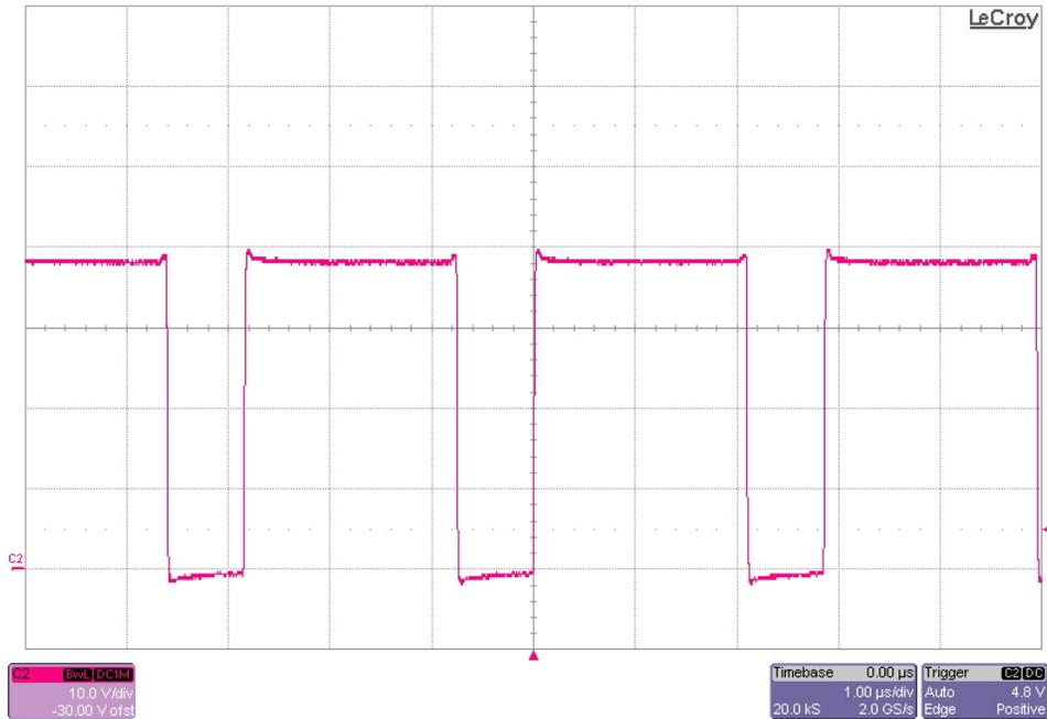
The photo below shows the FET switching voltage. The input voltage is 15V and the output is loaded to 0.17A. The converter is just starting DCM operation. (10V/DIV, 1uS/DIV)
