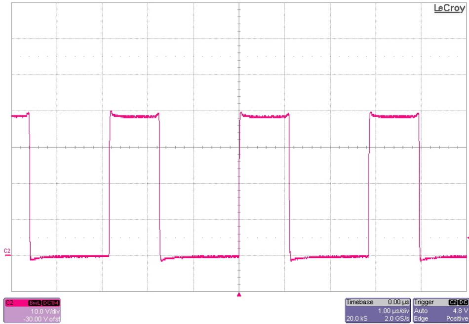
The photo below shows the FET switching voltage. The input voltage is 28V and the output is loaded to 2A. (10V/DIV, 1uS/DIV)
