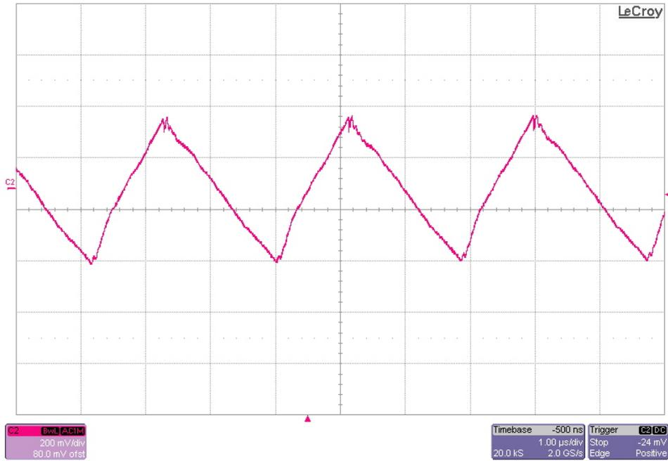
The 38V output ripple voltage is shown in the figure below. The image was taken with the output loaded to 2A. The input voltage is set to 24V. (100mV/DIV, 1uS/DIV)
