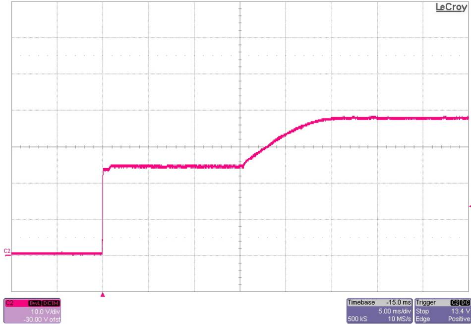
The photo below shows the output voltage startup waveform after the application of 24V in. The 38V output was loaded to 2A. (2V/DIV, 5mS/DIV)
