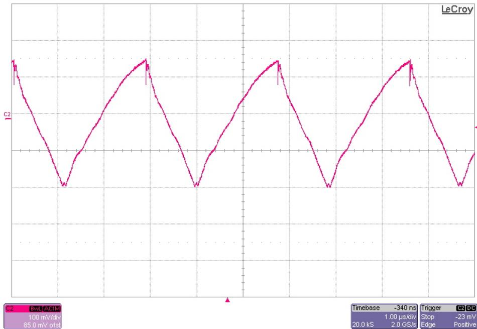
The 38V output ripple voltage is shown in the figure below. The image was taken with the output loaded to 2A. The input voltage is set to 28V. (100mV/DIV, 1uS/DIV)
