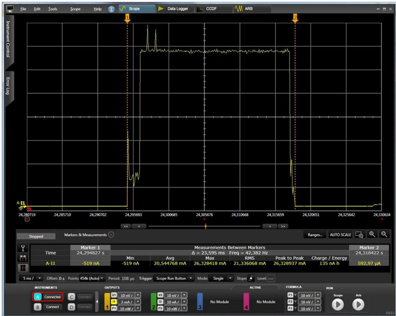
Figure 19. 20.54-mA Average Current During RF Transmission Pulse at 12.5 dBm; MSP430FR4133 is in LPM3; LCD BTL002 is Off
