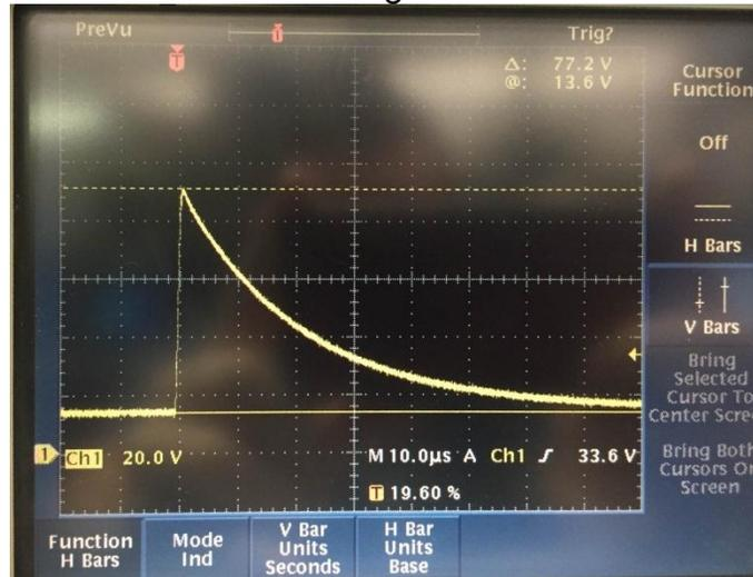
**Figure 48: Pulse 2a test pulse**
