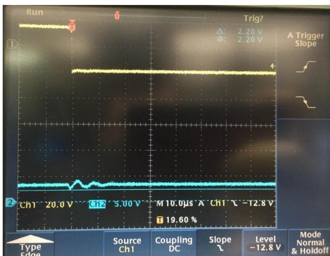
**Figure 47: Maximum undershoot is 2.2V, which may be too low to maintain some downstream converters regulation. Additional hold-up caps can be added to converter inputs to prevent loss of regulation during the pulse**
