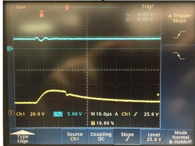
**Figure 50: Maximum overshoot is 4V which is low enough to avoid damage to downstream devices**
