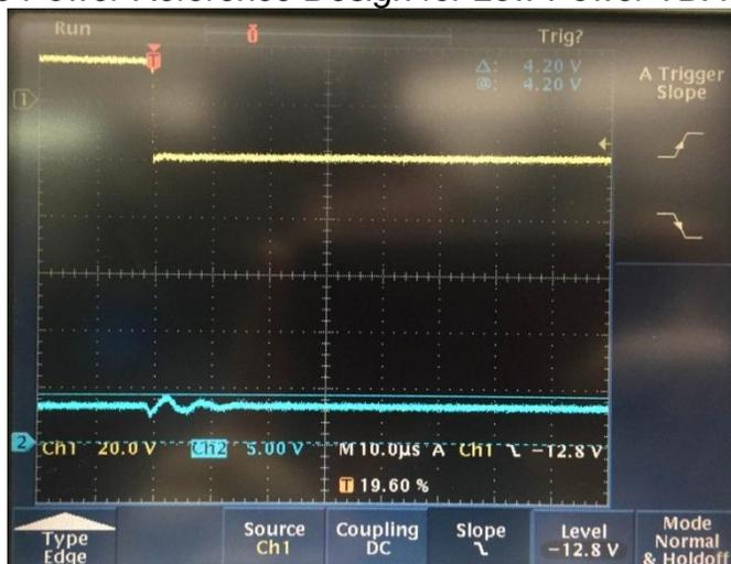
**Figure 46: Maximum overshoot is 4.2V which protects downstream circuits**
