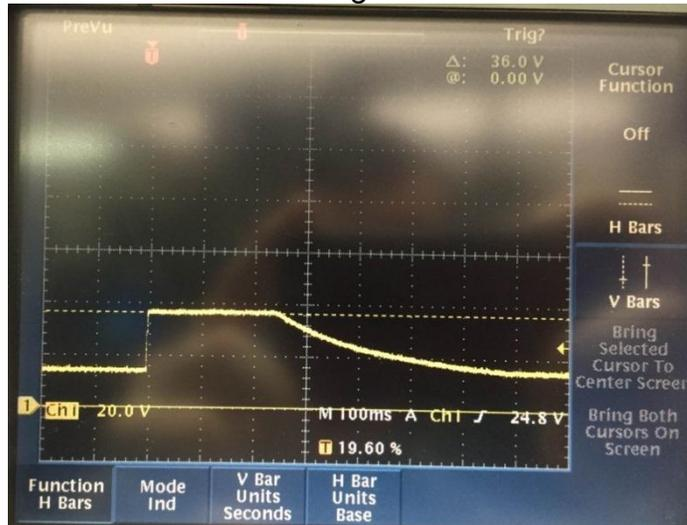
**Figure 51: Pulse 5b (clamped load dump) test pulse**
