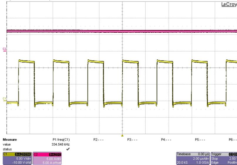
The device is switching at 334 kHz
