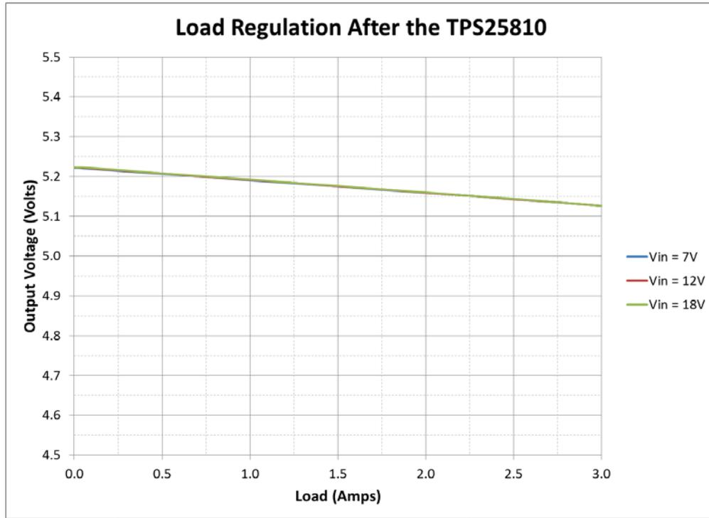
The load regulation of the board measured after the USB cable is shown in the figure below.
