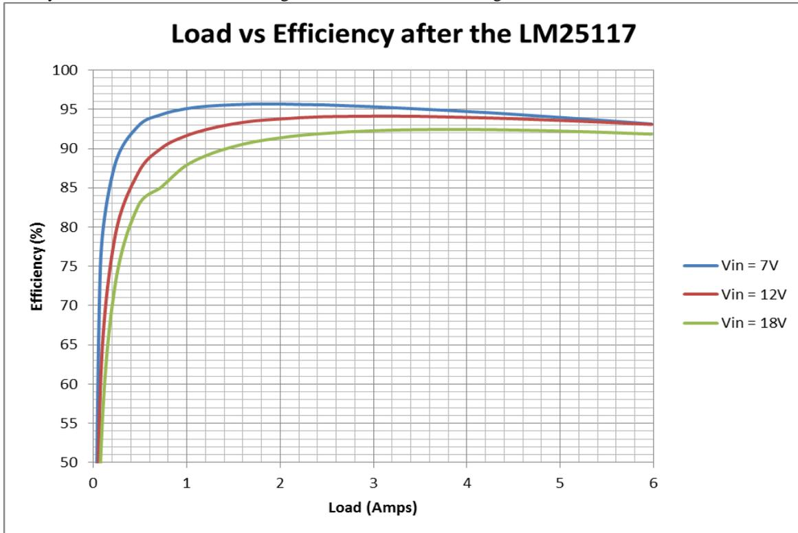
The efficiency of the board measured after the USB switch is shown in the figure below.
